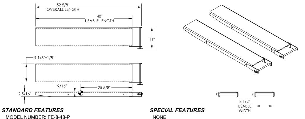
FORK EXTENSION WIDTH: 9 1/8" OVERALL WIDTH W/ RETAINING PIN: 11"
