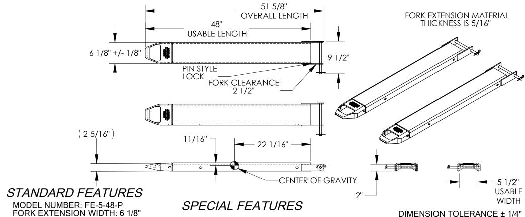
OVERALL WIDTH W/ RETAINING PIN: 9 1/2" NONE
