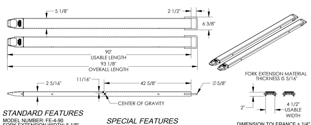
FORK EXTENSION WIDTH: 5 1/8" OVERALL WIDTH W/ LOOP: 6 3/8" **USABLE WIDTH: 4 1/2" OVERALL LENGTH: 93 1/8" USABLE LENGTH: 90"** FITS 4" WIDE x 2" MAX. THICKNESS FORK SOLID STEEL CONSTRUCTION TOUGH BAKED IN POWDER COATED YELLOW FINISH APPROX. WEIGHT / LOST LOAD = 139.28 LBS. PER PAIR
