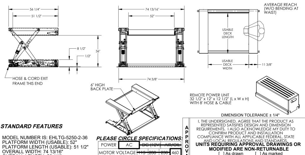
OVERALL WIDTH: 74 13/16" OVERALL LENGTH: 56 1/4" PLATFORM RAISED HEIGHT: 36" PLATFORM LOWERED HEIGHT: 1/2"
