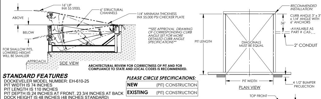
DURABLE LIQUID PAINT BROWN FINISH WITH YELLOW DECK SIDES & TOE GUARDS \*\*\*SINGLE AXLE CAPACITY NOT TO EXCEED 70% OF LOAD\*\*\* ALL STRUCTURAL STEEL CONSTRUCTION WELDING MEETS AWS. DESIGN, ENGINEERING, AND FABRICATION
