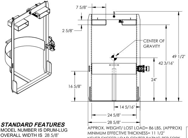
OVERALL WIDTH IS 28 5/8" OVERALL LENGTH IS 19 3/4" OVERALL HEIGHT IS 49 1/2" **UNIFORM CAPACITY IS 1,000 LBS** RATCHET STRAP SECURES DRUM ACCOMMODATES 30 AND 55-GALLON
