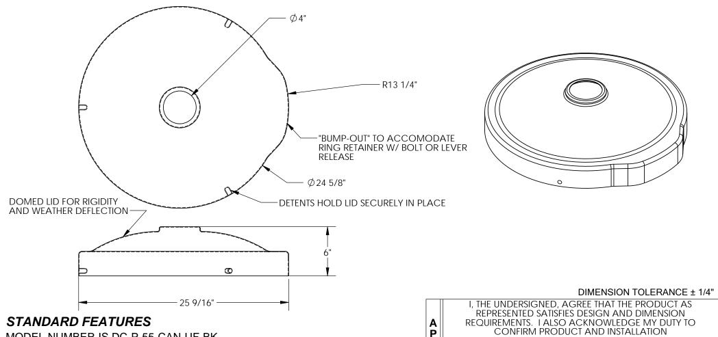
MODEL NUMBER IS DC-P-55-CAN-UF-BK OVERALL DIAMETER IS \$\infty 24 5/8"\$ OVERALL LENGTH IS 25 9/16" OVERALL HEIGHT IS 6" MADE FROM LOW-DENSITY POLYETHYLENE DETENTS HOLD LID SECURELY IN PLACE DOMED LID FOR RIGIDITY AND WEATHER DEFLECTION "BUMP-OUT" ON OUTER DIAMETER WILL ACCOMODATE RING RETAINER W/ BOLT OR INSIDE OR OUTSIDE LEVER RELEASE
