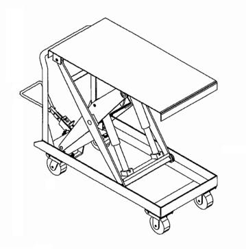
After receiving a hydraulic elevating cart, visually inspect the frame components and hydraulic unit for damage. If damage is evident, notify delivering carrier immediately and file necessary claims.
