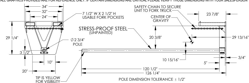
HORIZONTAL CENTER OF GRAVITY: 29 13/16" VERTICAL CENTER OF GRAVITY: 10 15/16" LOST LOAD: 479 LBS. (APPROX.) MINIMUM EFFECTIVE THICKNESS = LESS THAN 1" NOTE: NEVER EXCEED LOAD CENTER RATING PER FORK TRUCK MANUFACTURER'S GUIDELINES. DO NOT USE THIS FORK TRUCK ATTACHMENT IF LOAD WILL EXCEED FORK TRUCK MANUFACTURER'S LOAD CENTER RATING.
