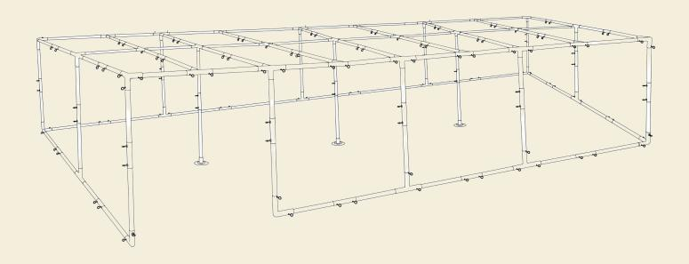
The horizontal poles are all 5 feet, and the vertical poles are made up of 2 - 4 ft poles attached together with a 2-Way Connector - just like the horizontal poles from Step 2.
