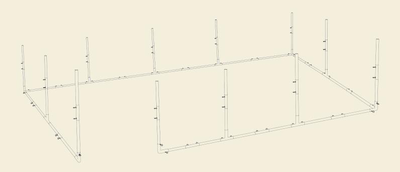
The upward poles are all 4 feet long. Take 2 - 4 foot poles and connect them using a 2- Way Connector to create an 8 foot vertical pole.
