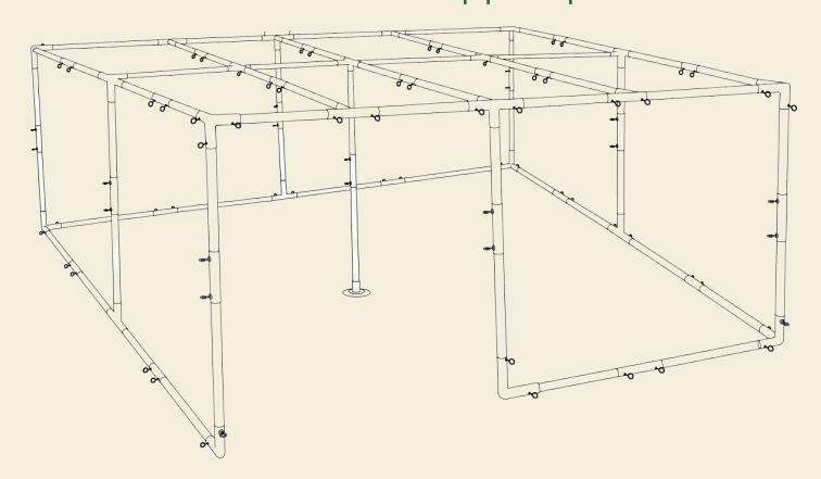
The horizontal poles are all 5 feet, and the vertical pole is made up of 2 - 4 ft poles.
