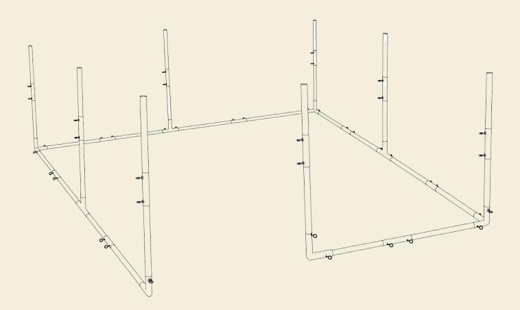
The upward poles are all 4 feet long. Take 2 - 4 foot poles and connect them using a 2- Way Connector to create an 8 foot vertical pole.
