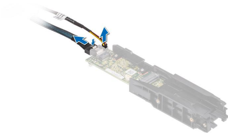
Figure 191. Removing the BOSS S2 power and signal cable from the BOSS S2 module
