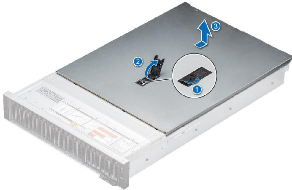
Figure 27. Removing the system cover
