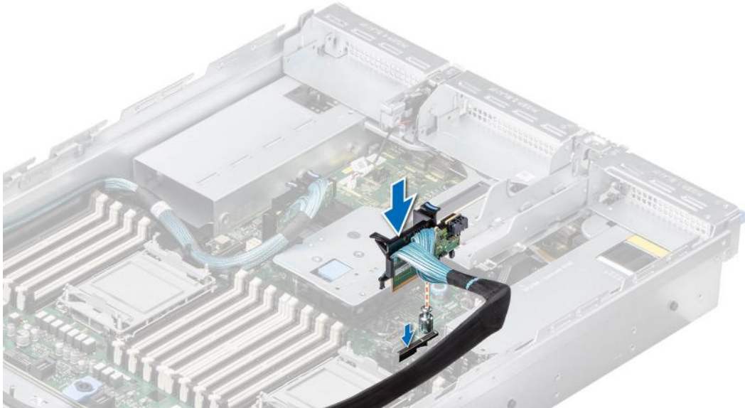
Figure 168. Installing the R1 paddle card
