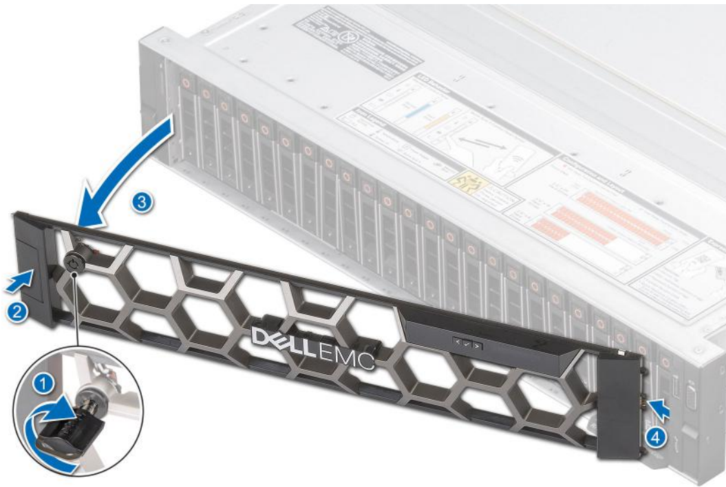
Figure 25. Removing the front bezel with the LCD panel
