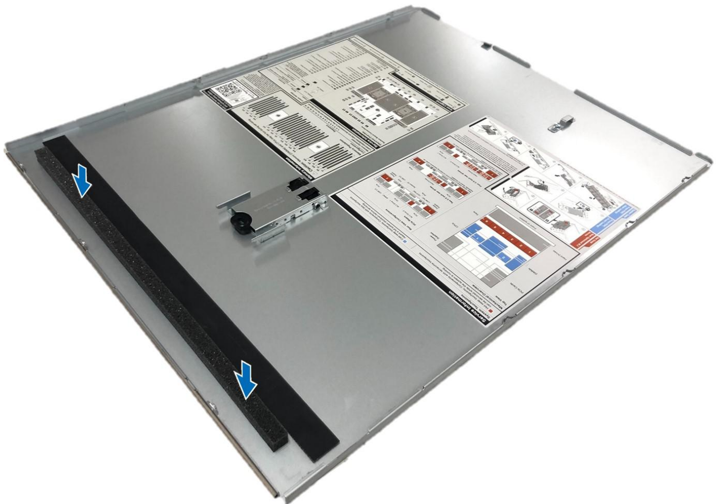
Figure 226. Installing Mylar foam on the system cover
