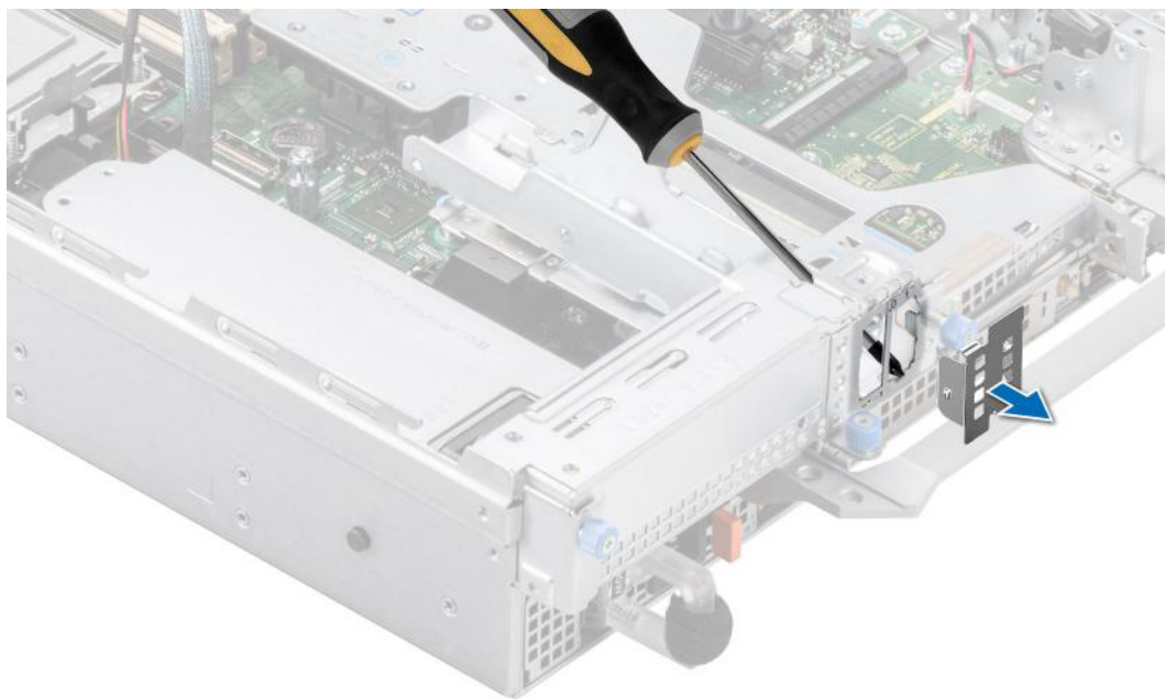
Figure 224. Removing the BOSS S2 module blank
