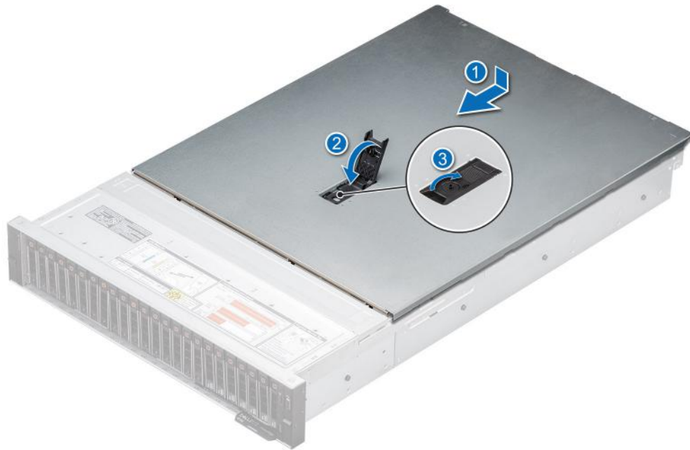
Figure 28. Installing the system cover
