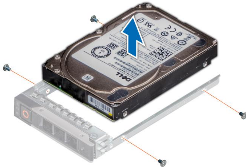
Figure 53. Removing the drive from the drive carrier
