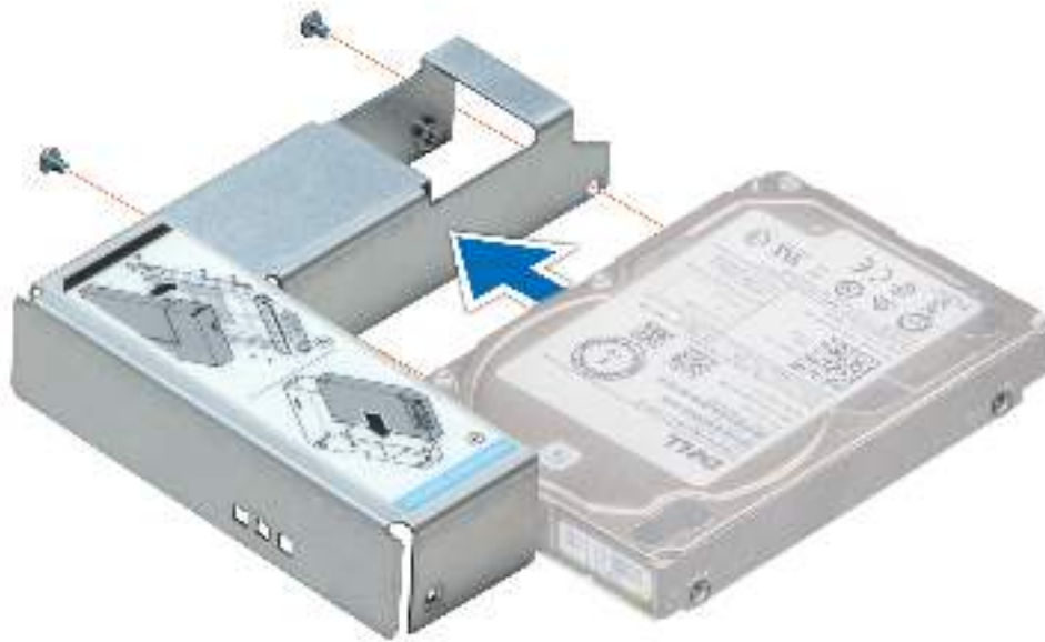
Figure 57. Installing a 2.5-inch drive into a 3.5-inch drive adapter
