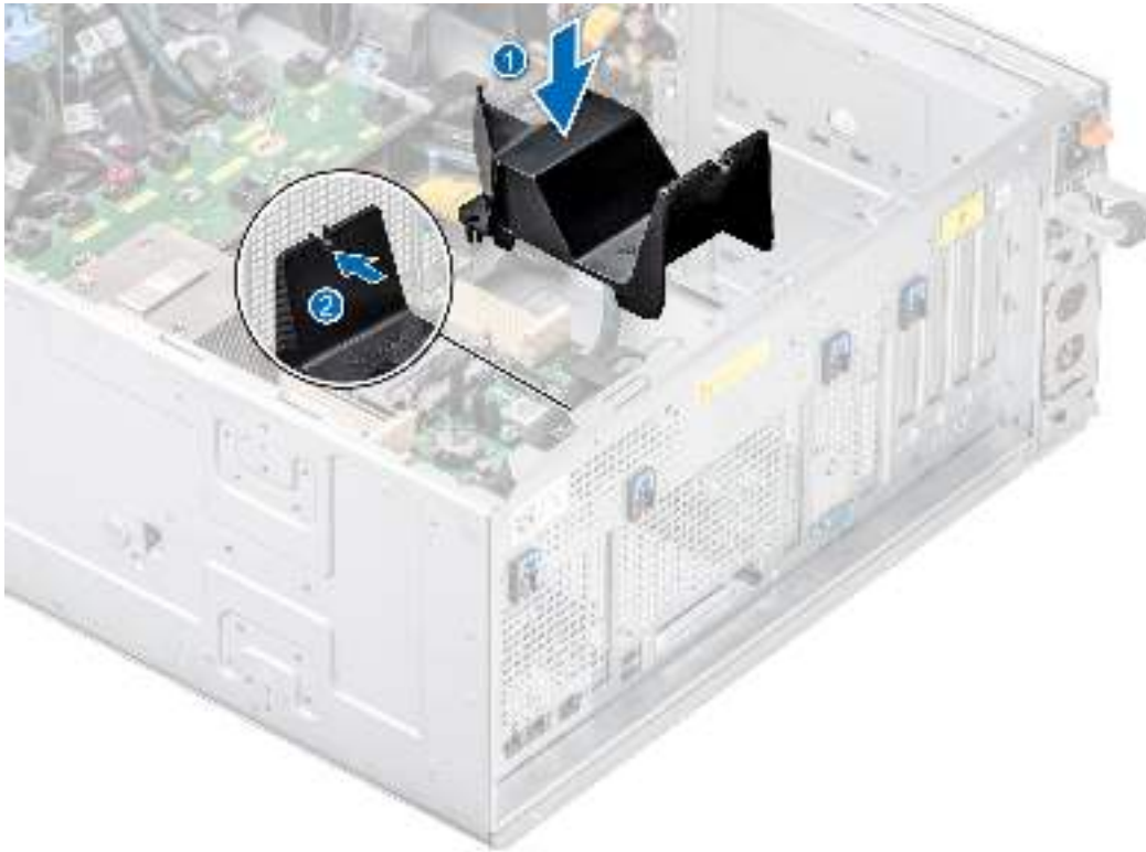
Figure 158. Installing the OCP air shroud.
