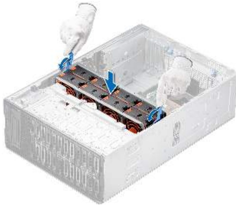
Figure 40. Installing the cooling fan cage
