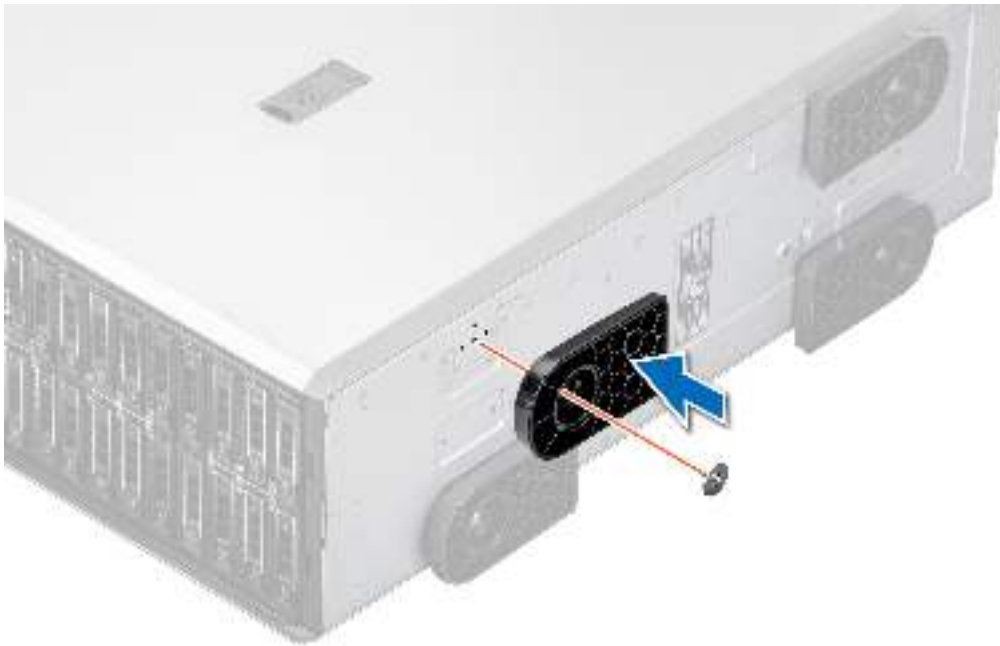
Figure 30. Installing the system feet
