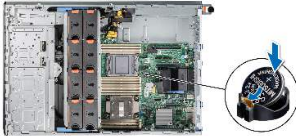
Figure 162. Installing the system battery
