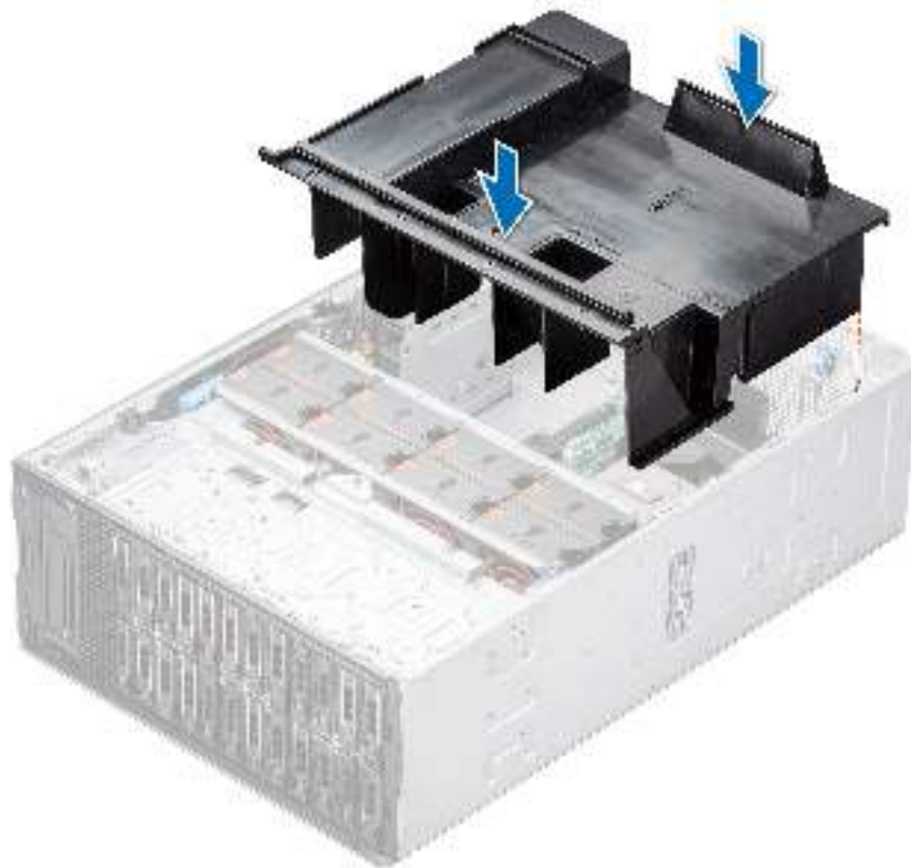
Figure 36. Installing the air shroud
