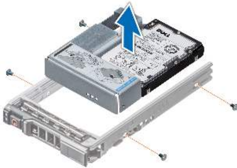
Figure 54. Removing a 3.5-inch drive adapter from a 3.5-inch drive carrier
