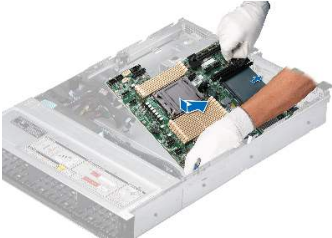
Figure 127. Installing the system board
