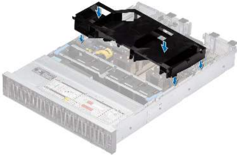
Figure 26. Installing the air shroud
