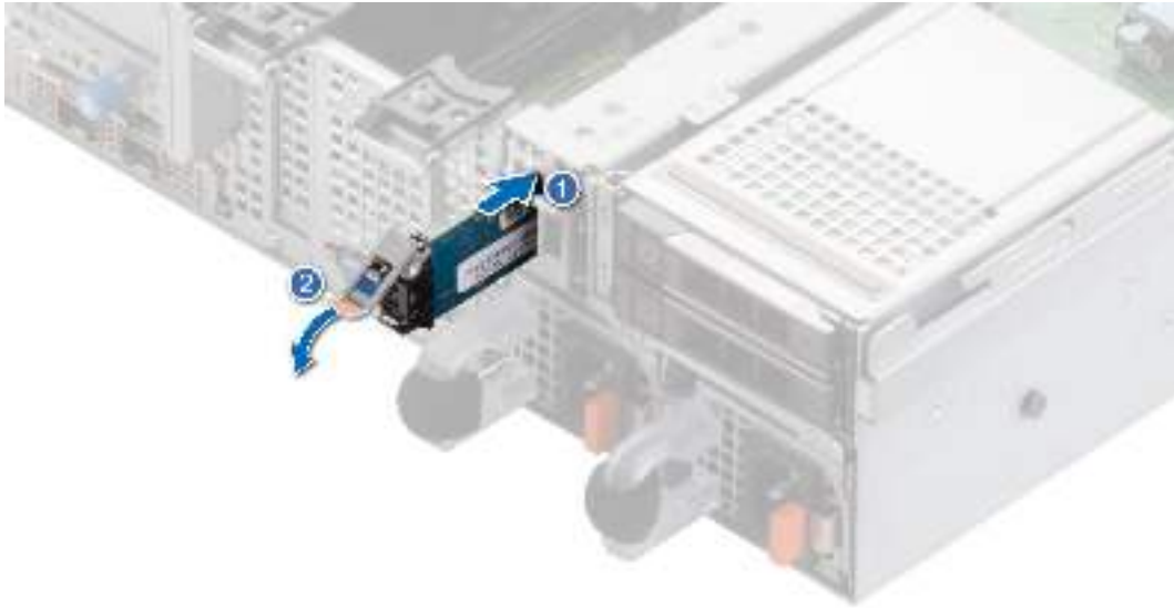
Figure 103. Installing the BOSS S2 card carrier
