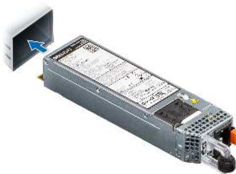
Figure 123. Installing a power supply unit
