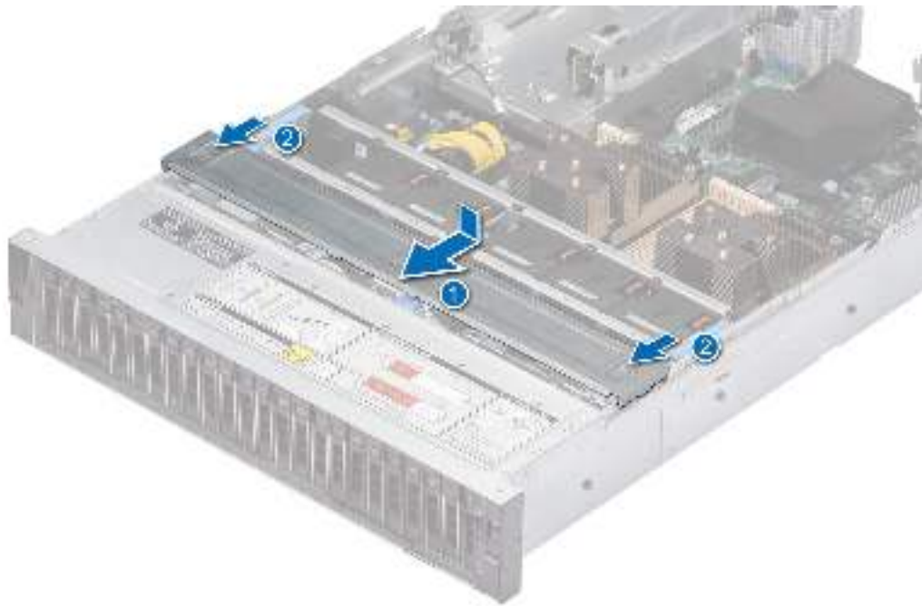
Figure 22. Installing the drive backplane cover
