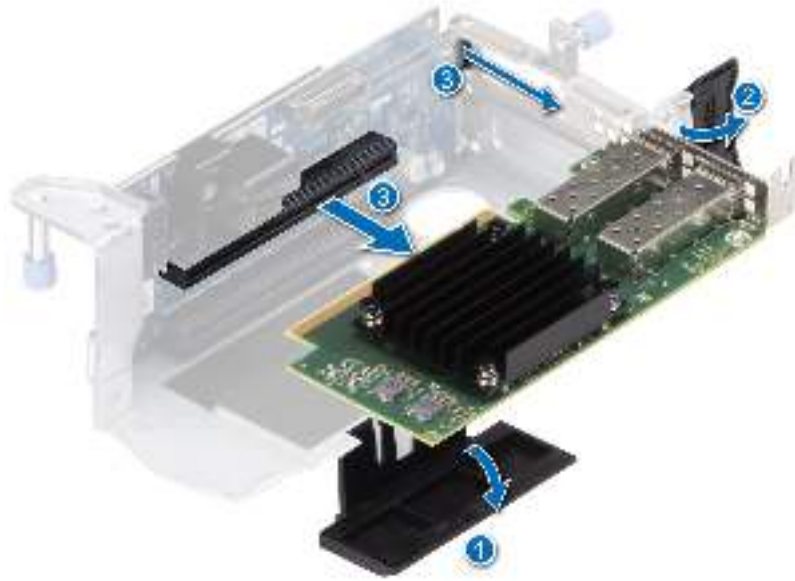
Figure 85. Removing an expansion card from Riser 1B
