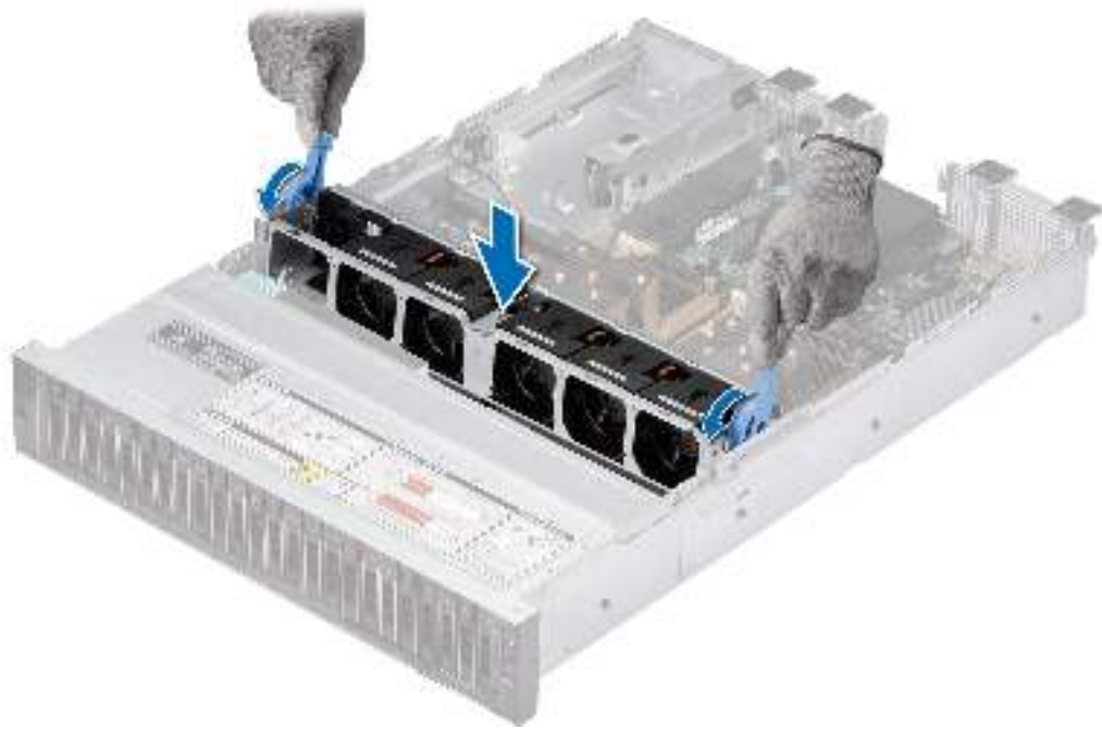
Figure 30. Installing the cooling fan cage
