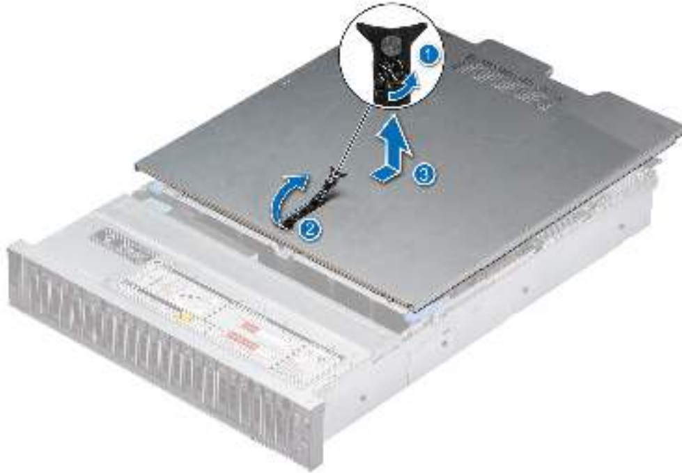
Figure 19. Removing the system cover
