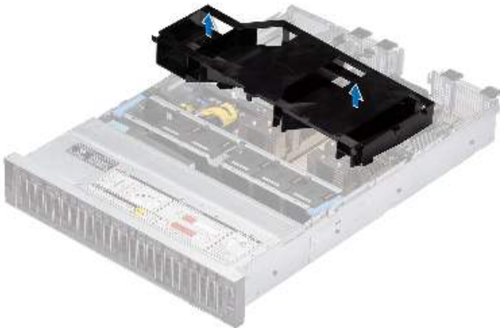
Figure 25. Removing the air shroud
