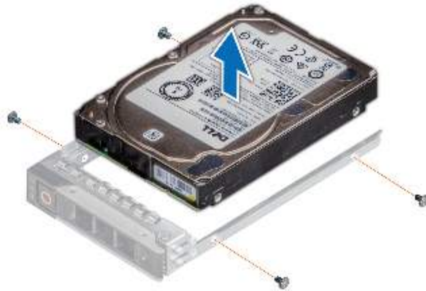
Figure 43. Removing the drive from the drive carrier
