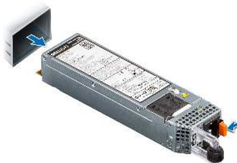
Figure 122. Removing a power supply unit
