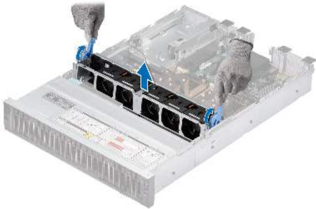
Figure 29. Removing the cooling fan cage
