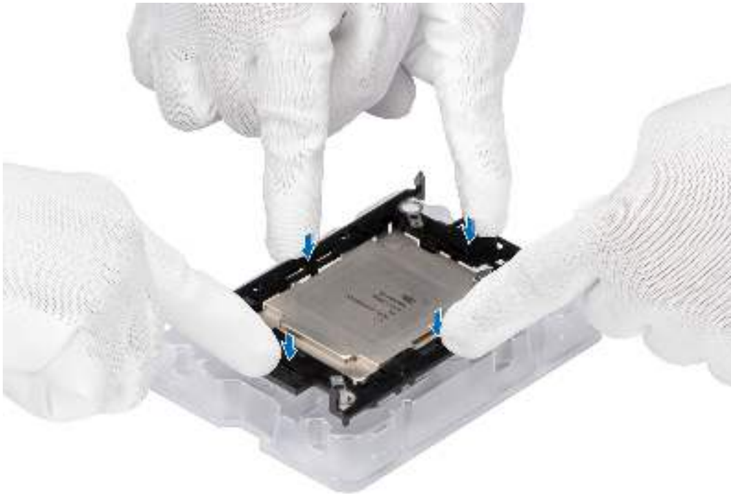
Figure 71. Press the carrier on the four sides
