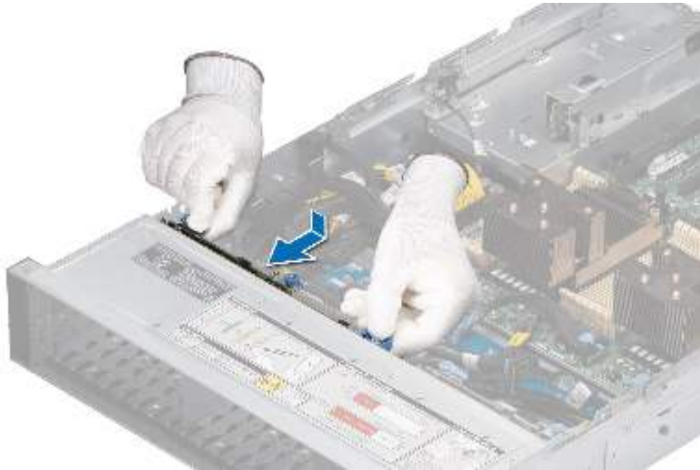
Figure 50. Installing the drive backplane
