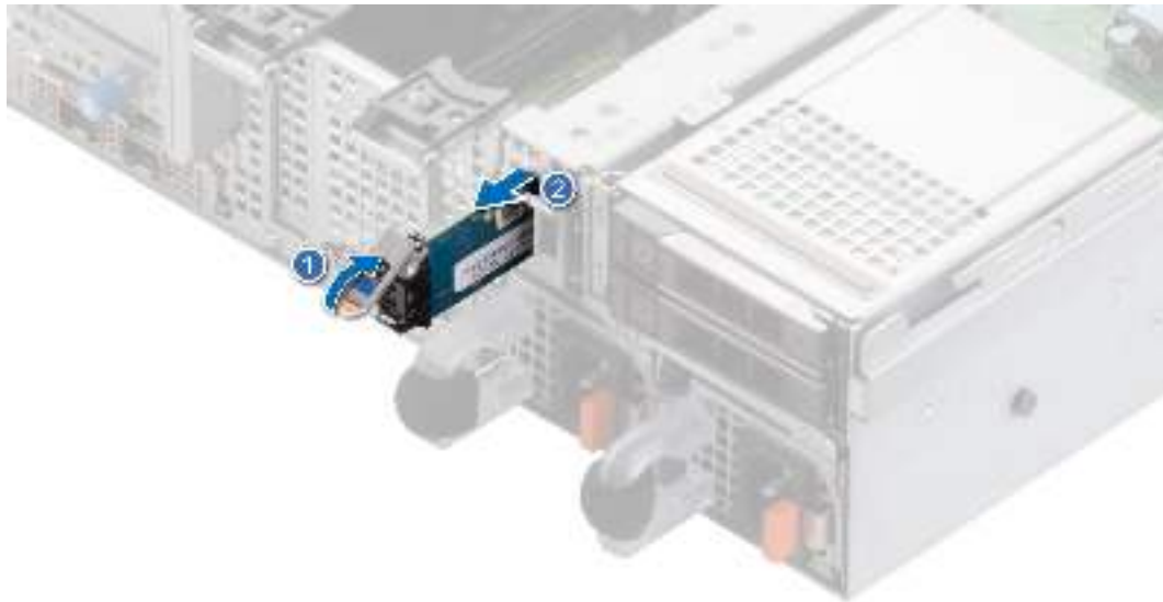
Figure 94. Removing the BOSS S2 card carrier
