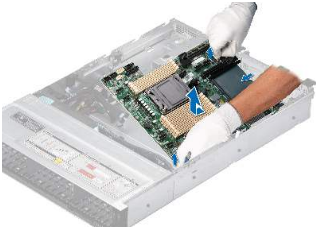
Figure 126. Removing the system board
