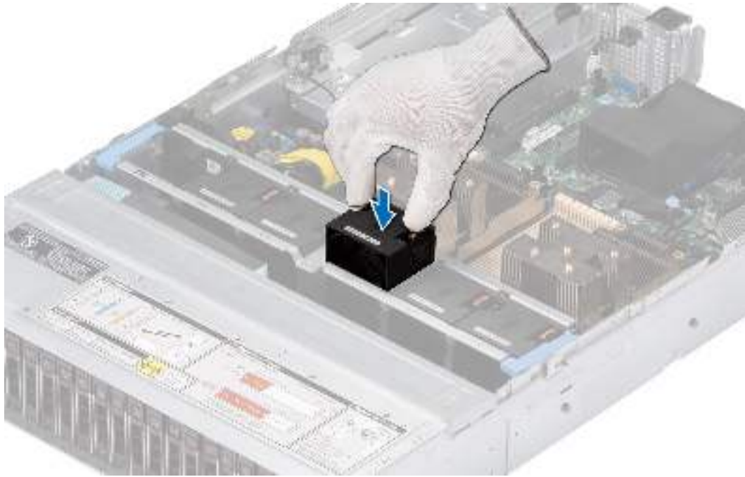
Figure 28. Installing a cooling fan
