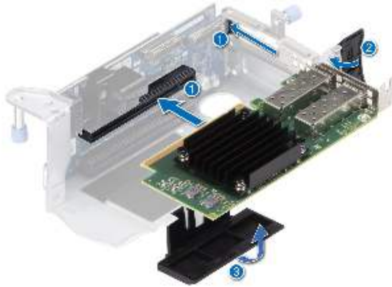
Figure 88. Installing the expansion card in the Riser 1A
