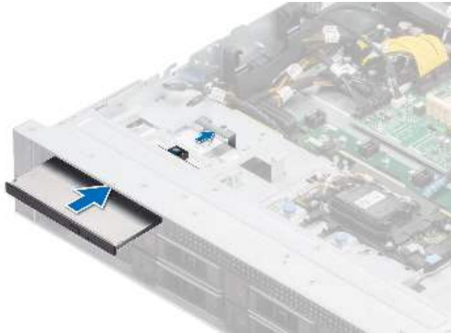
Figure 24. Installing the optical disk drive
