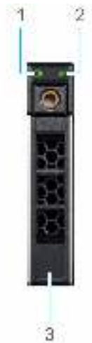
Figure 139. Drive indicators on the drive and the mid drive tray backplane
