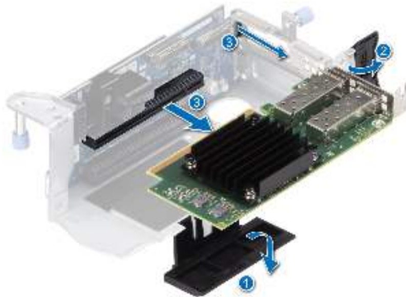
Figure 84. Removing an expansion card from the Riser 1A
