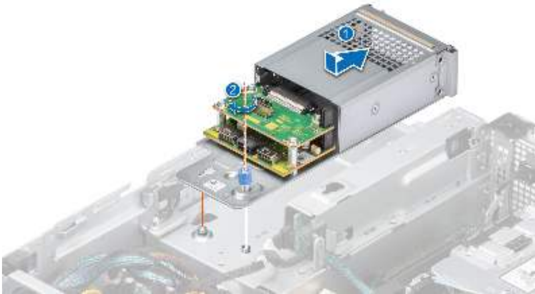
Figure 111. Installing the rear drive module
