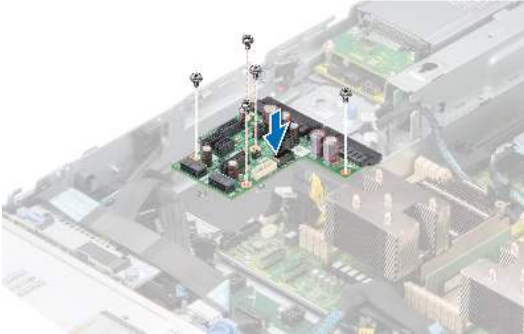
Figure 125. Installing the power interposer board
