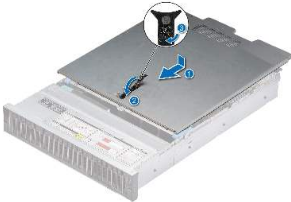
Figure 20. Installing the system cover
