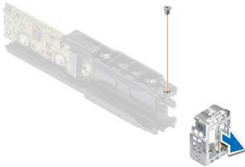
Figure 98. Removing the BOSS S2 module cover
