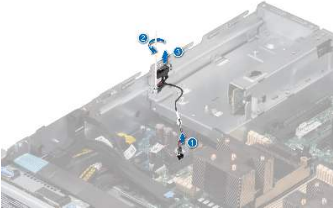
Figure 35. Removing the intrusion switch module
