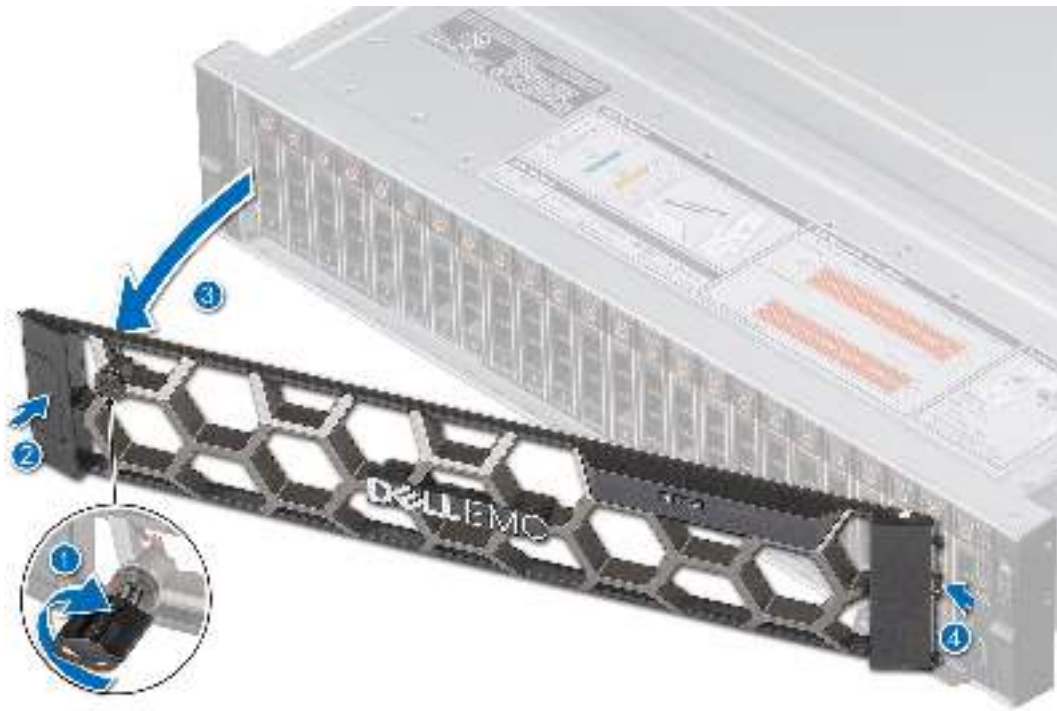
Figure 17. Removing the front bezel with the LCD panel
