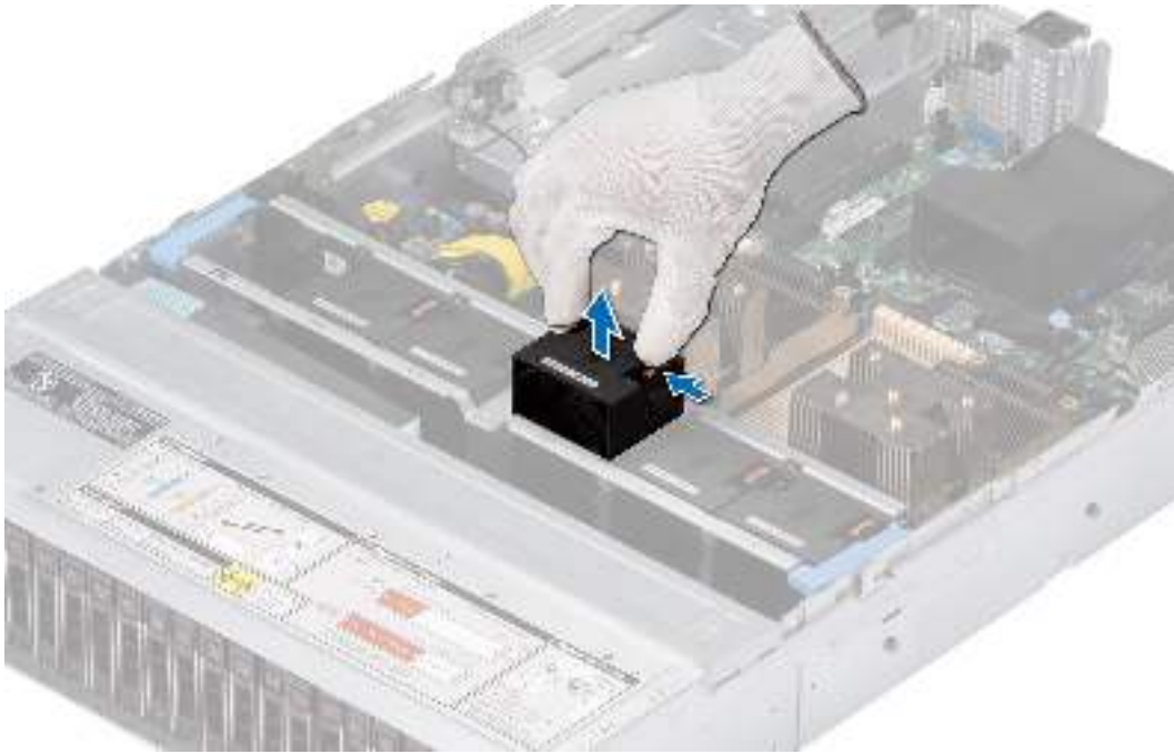
Figure 27. Removing a cooling fan
