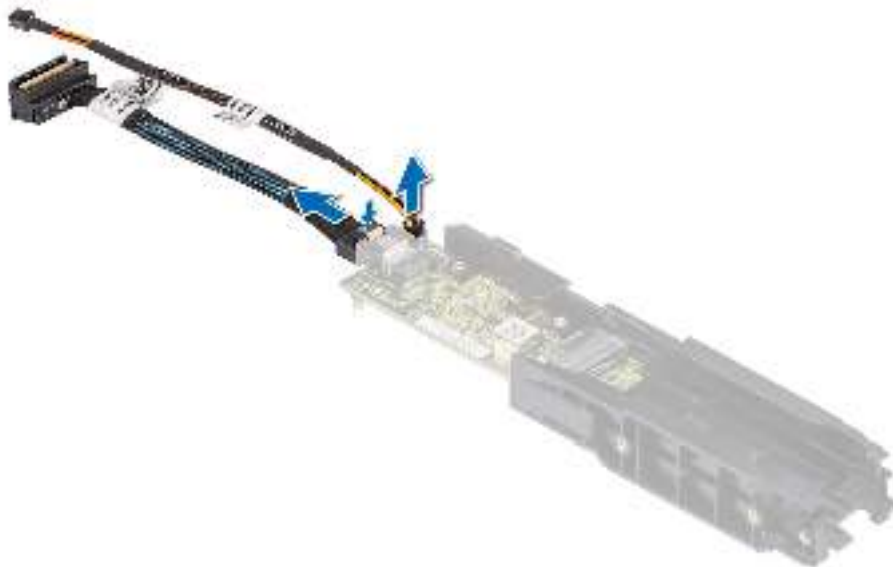
Figure 97. Removing the BOSS power cable and BOSS signal cable from the BOSS S2 controller card module
