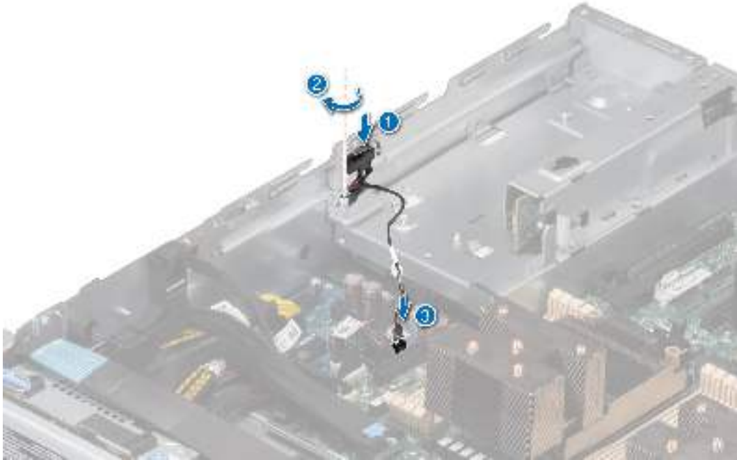
Figure 36. Installing the intrusion switch
