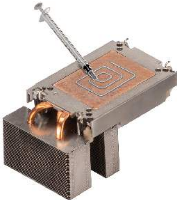
Figure 72. Applying thermal grease
