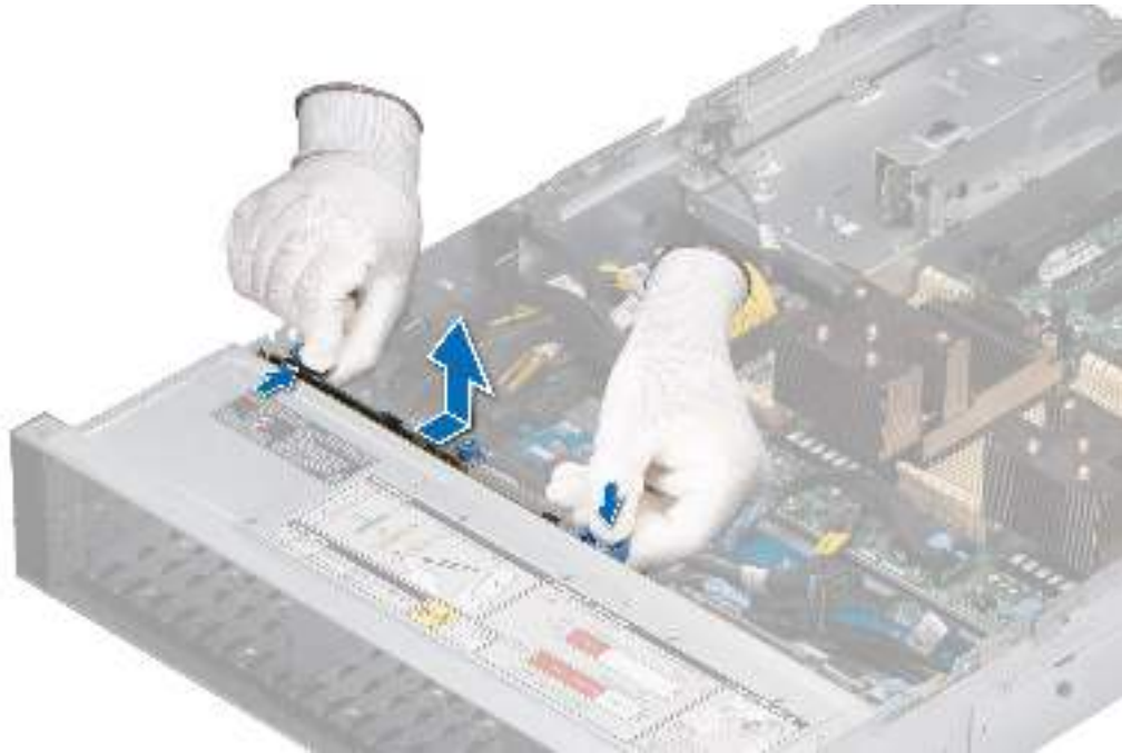
Figure 49. Removing the drive backplane
