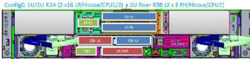
Figure 7. Rear view of the system with riser config 0: direct attach NVMe cards (either 6x NVMe direct attach or 4x NVMe direct attach + 4 Universal slots)
