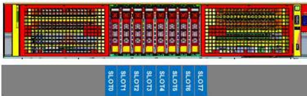
Figure 2. Front view of the R750xa with x8 SAS/SATA SSD on x8 NVMe
