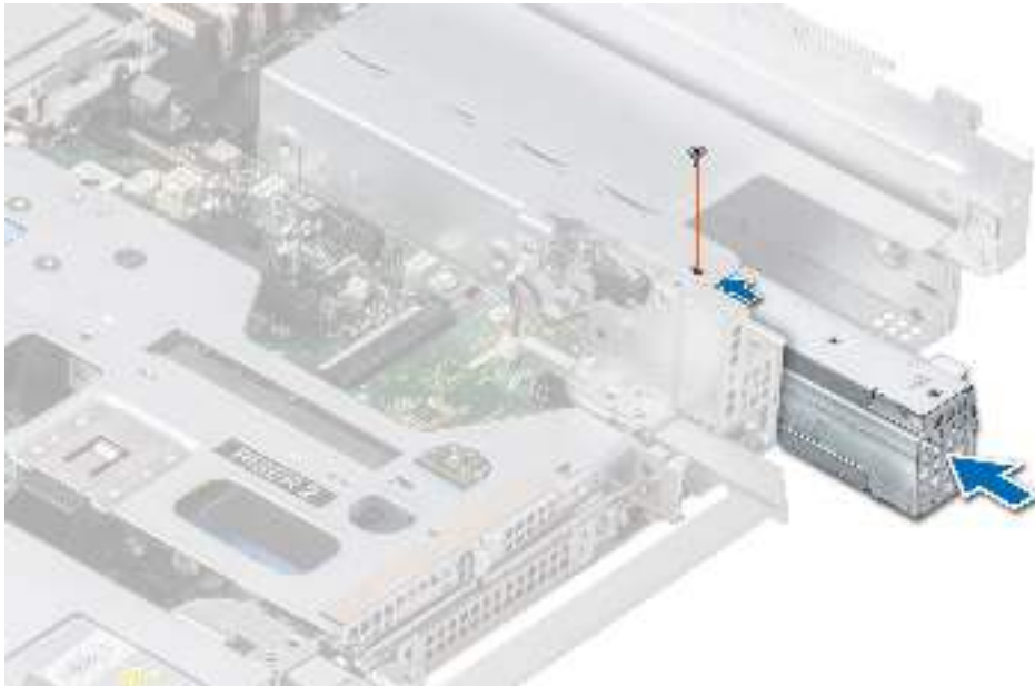
Figure 164. Installing a power supply unit adapter
