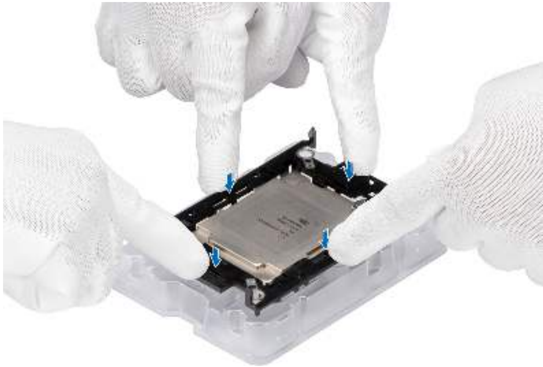
Figure 68. Press the retaining clip on the four sides
