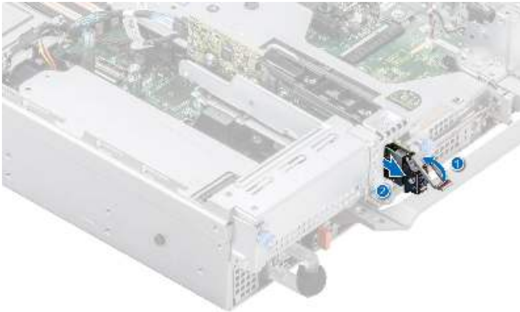
Figure 142. Removing the BOSS S2 card carrier
