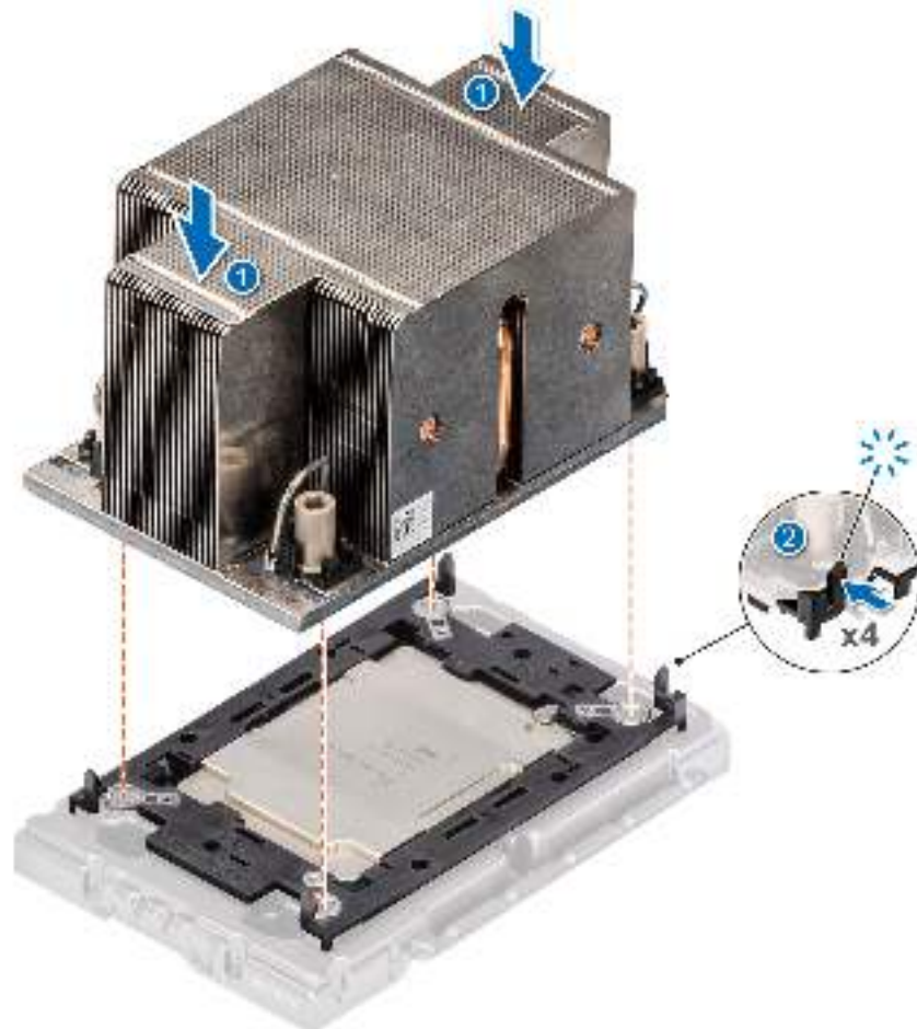
Figure 71. Installing the heat sink onto the processor
