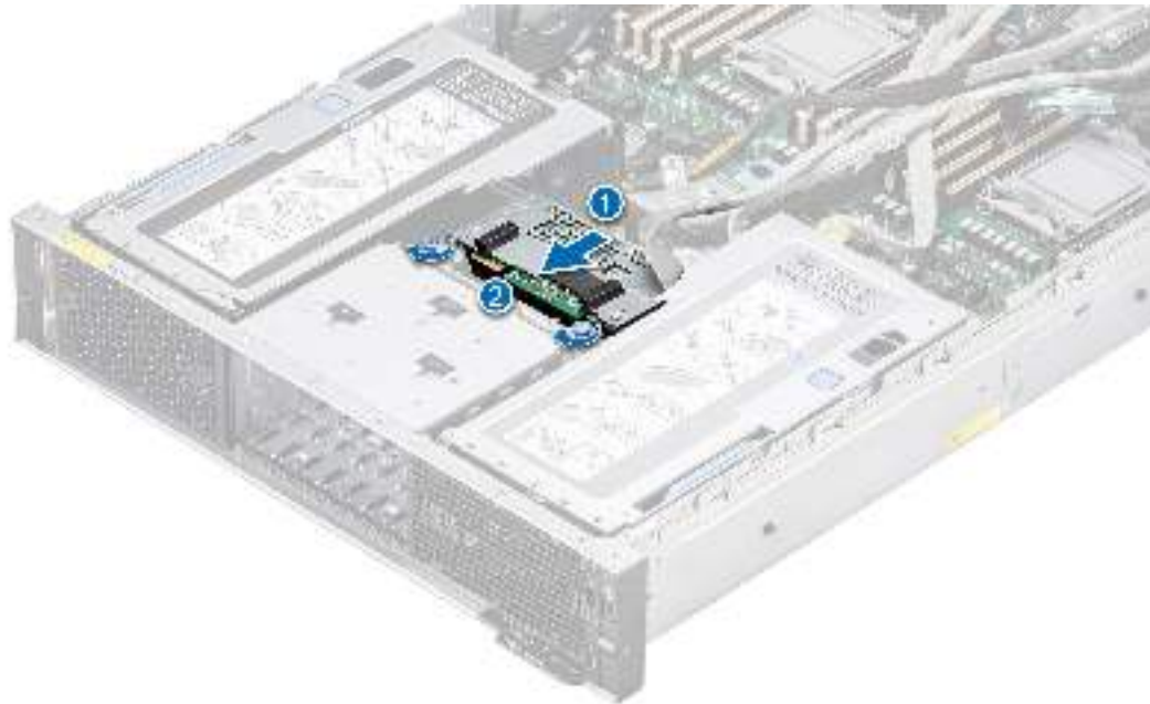
Figure 48. Installing the rear mounting front PERC module
