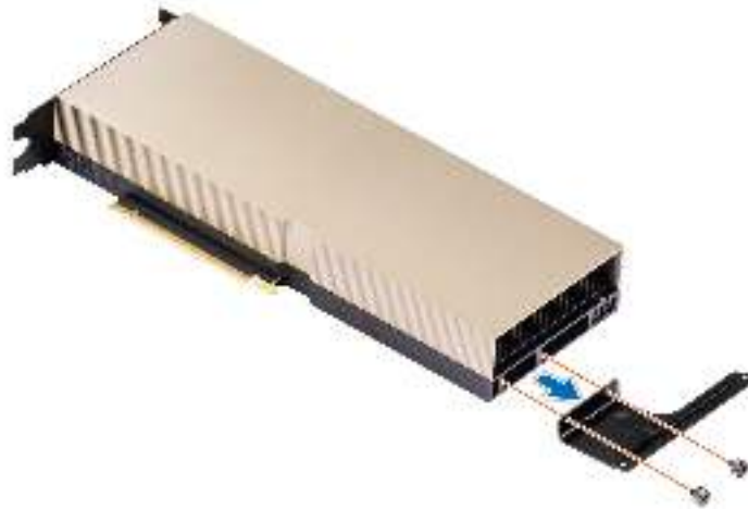
Figure 102. Removing the standard bracket with two screws
