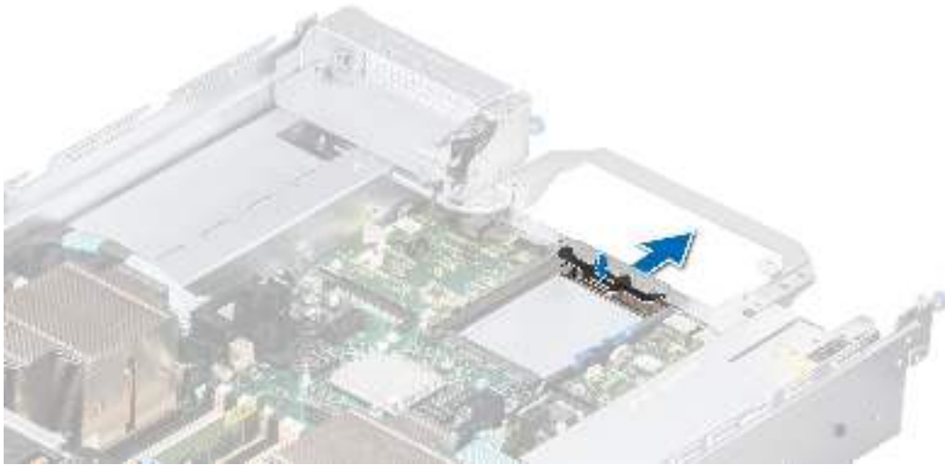
Figure 159. Removal of filler bracket
