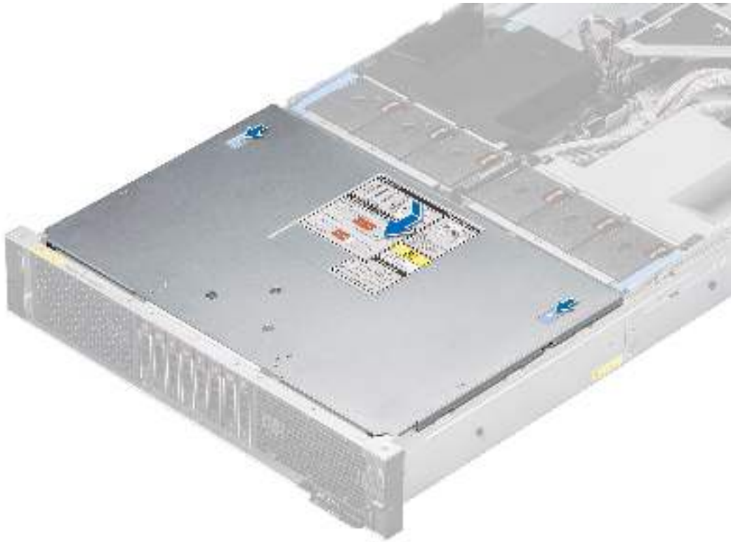
Figure 26. Installing the drive backplane cover
