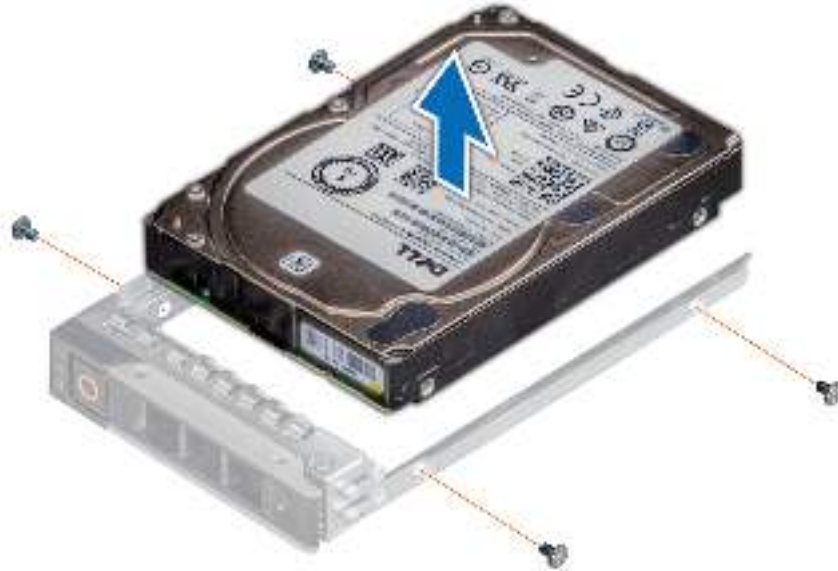
Figure 42. Removing the drive from the drive carrier
