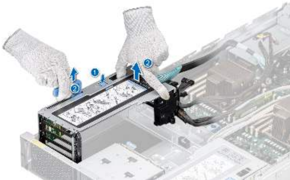
Figure 107. Removing the left GPU riser module
