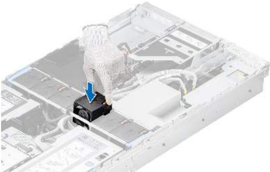
Figure 36. Installing a cooling fan
