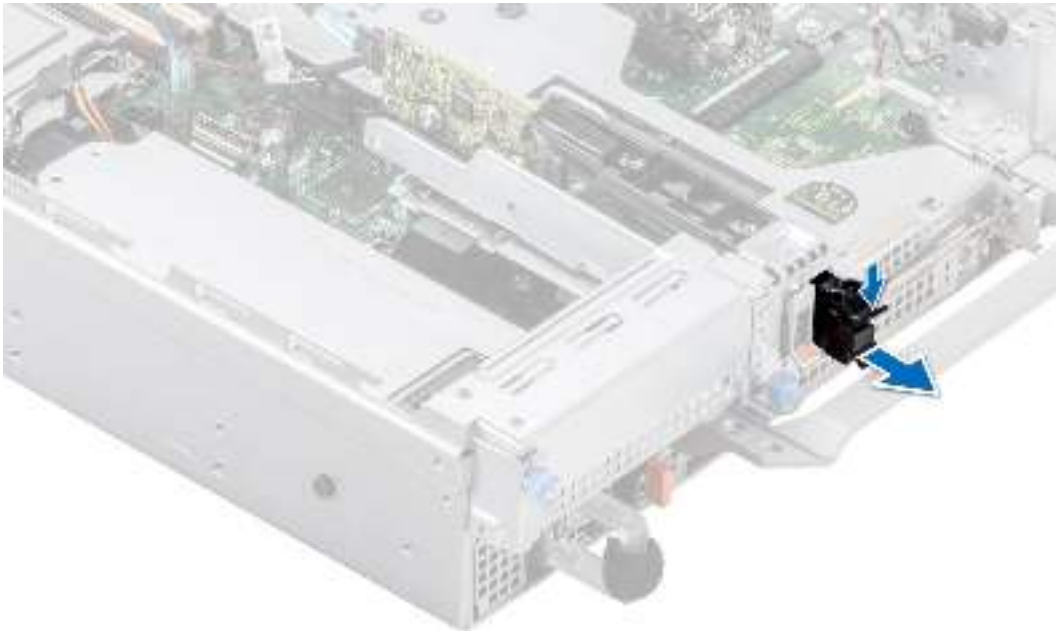
Figure 140. Removing the BOSS S2 card carrier blank
