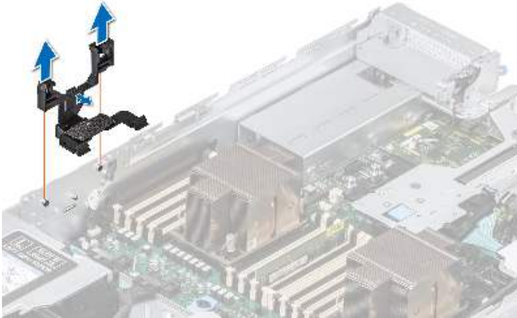
Figure 37. Removing the side wall bracket
