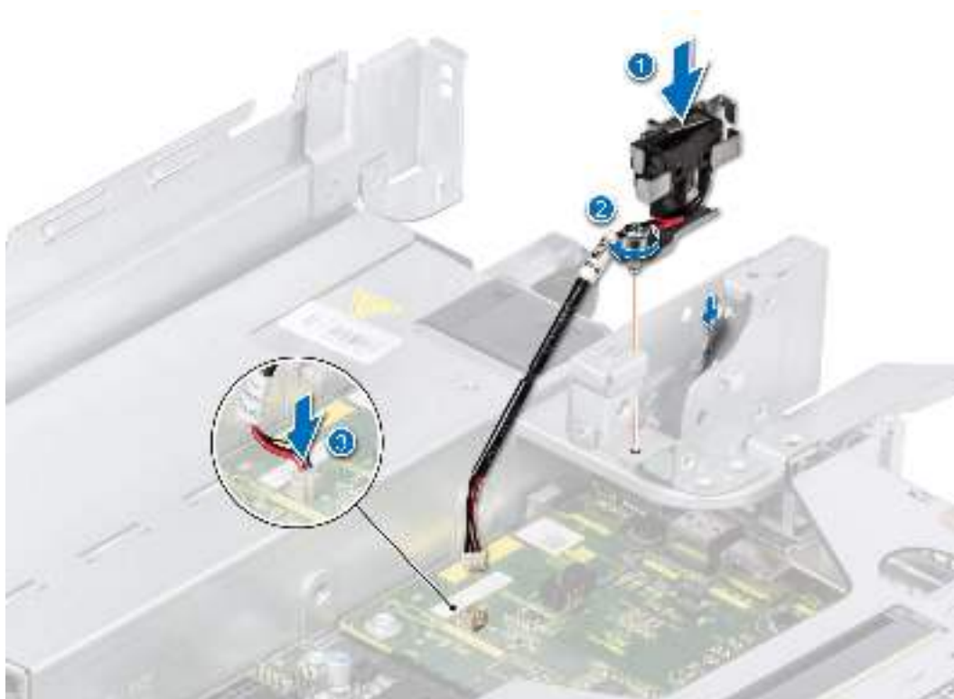
Figure 156. Installing the intrusion switch module
