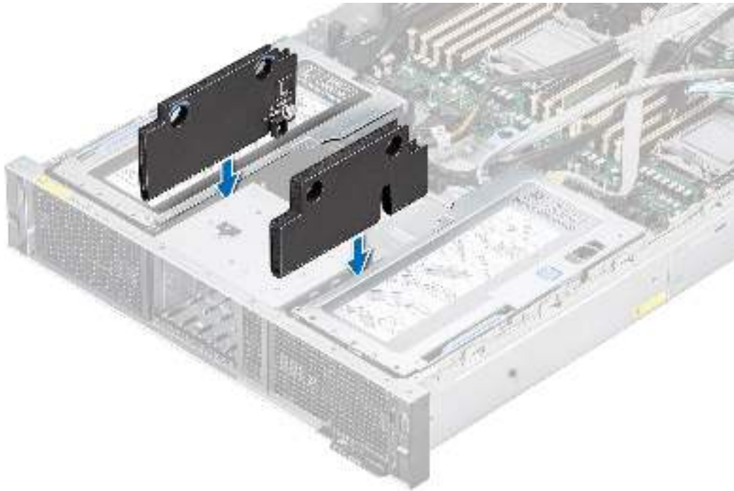
Figure 115. Installing the NVLink sponge
