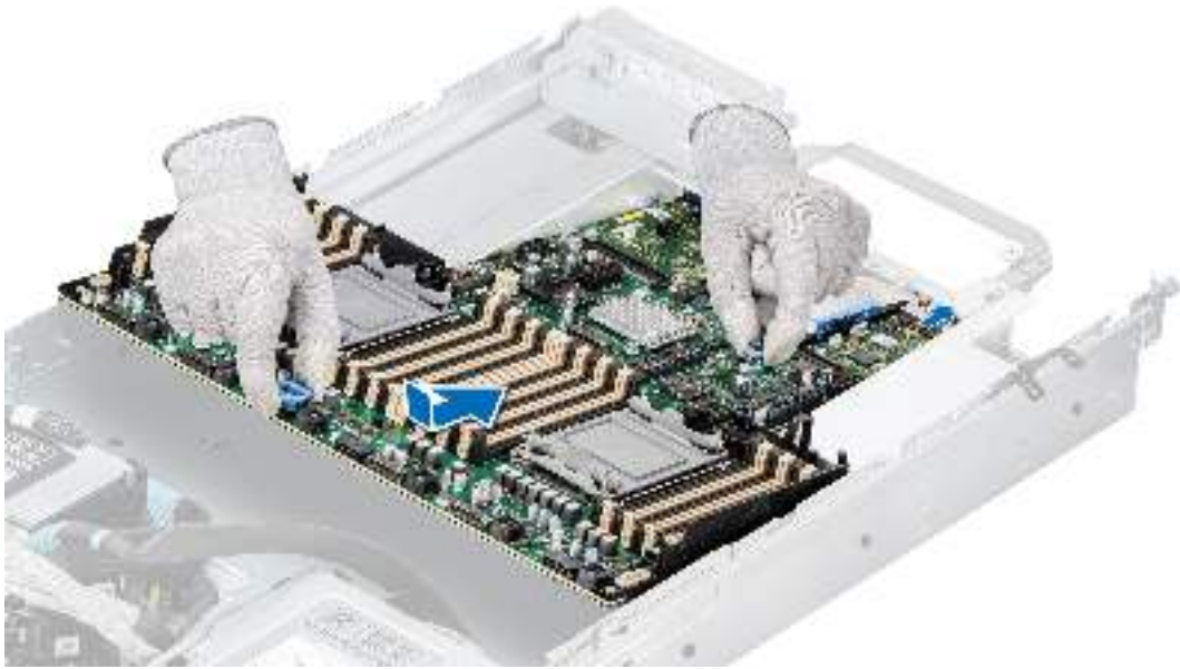
Figure 169. Installing the system board
