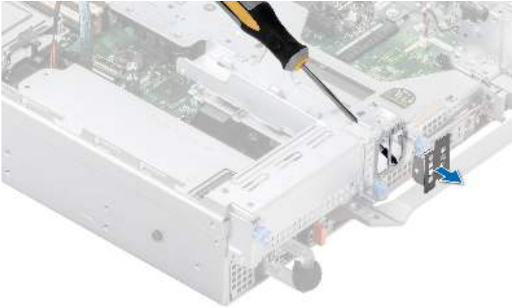
Figure 138. Removing the BOSS S2 module blank
