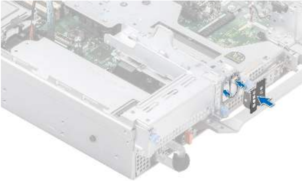
Figure 139. Installing the BOSS S2 module blank
