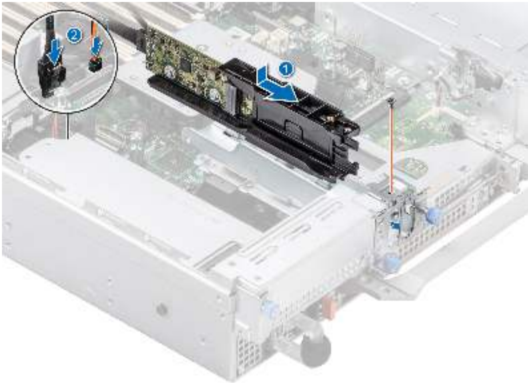
Figure 148. Installing the BOSS S2 module
