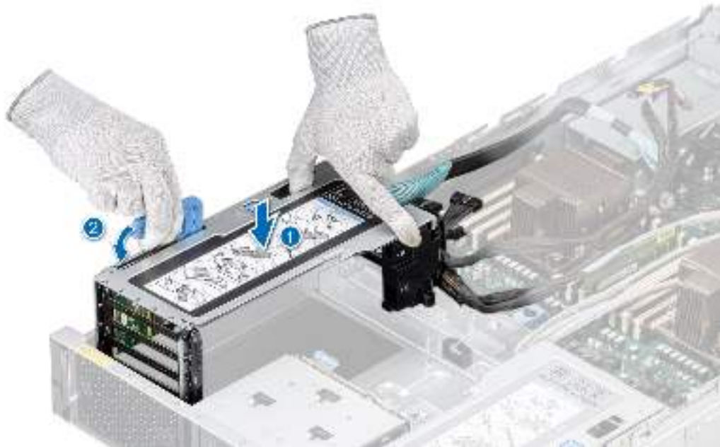
Figure 109. Installing the left GPU riser module
