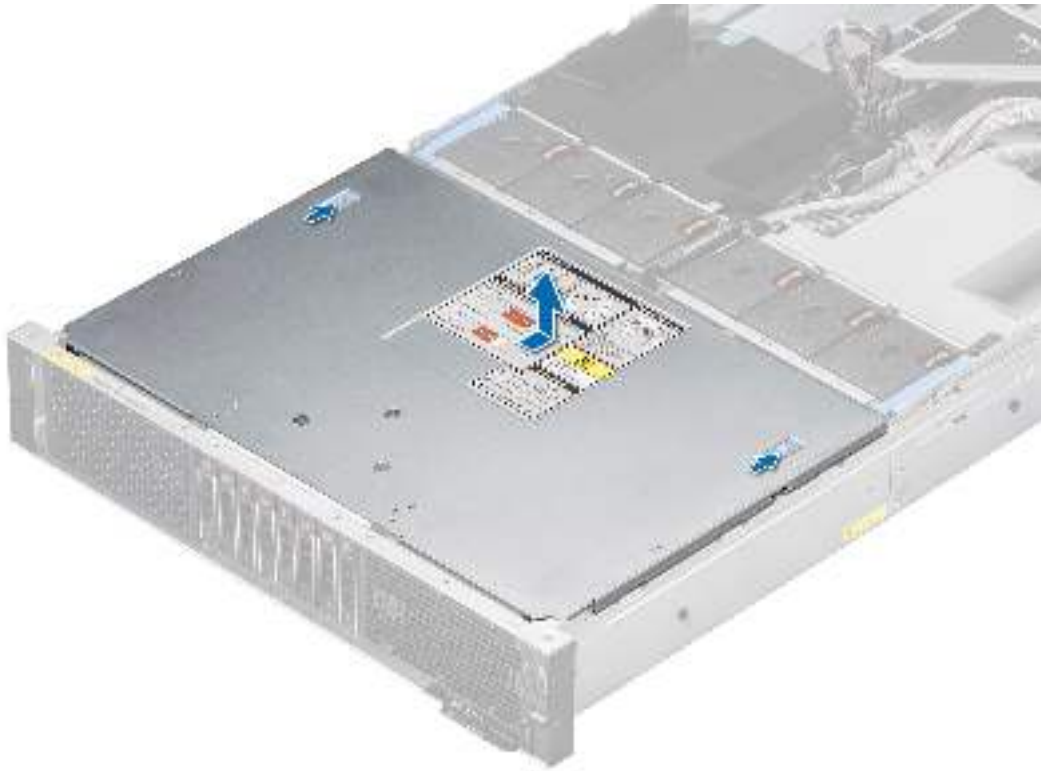
Figure 25. Removing the drive backplane cover
