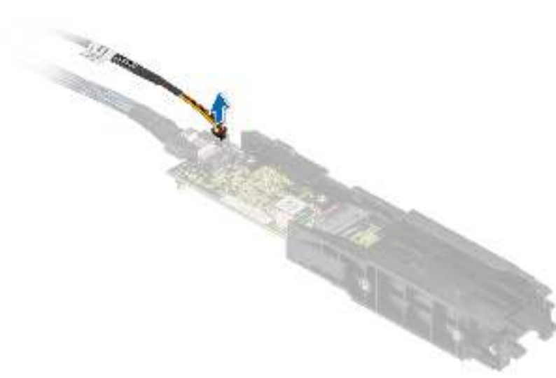
Figure 144. Disconnecting the BOSS S2 power cable
