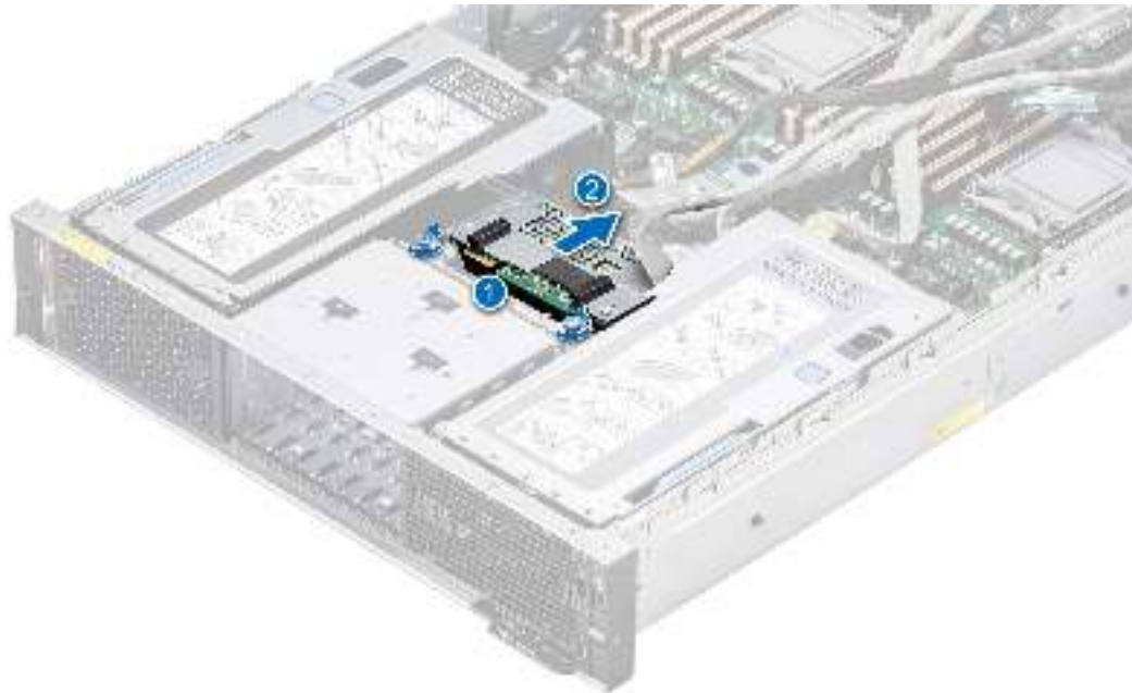
Figure 47. Removing the rear mounting front PERC module
