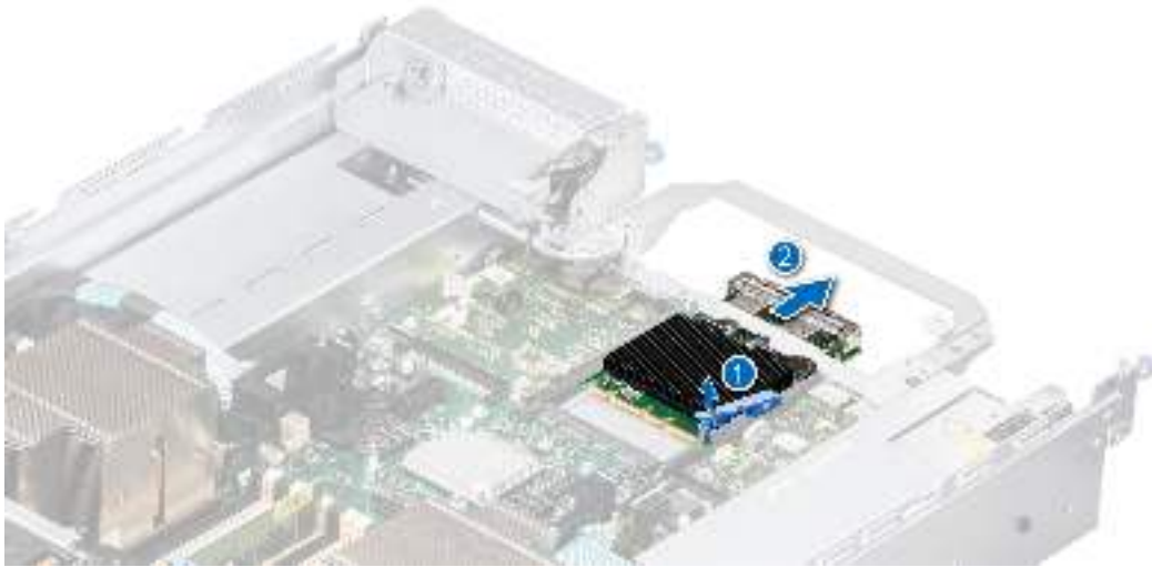
Figure 157. Removing the OCP card
