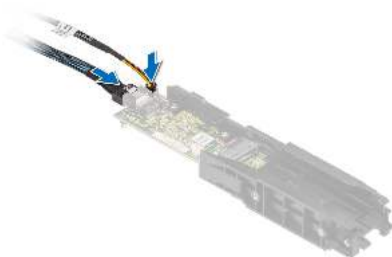
Figure 147. Connecting the BOSS S2 power and signal cables to the BOSS S2 module
