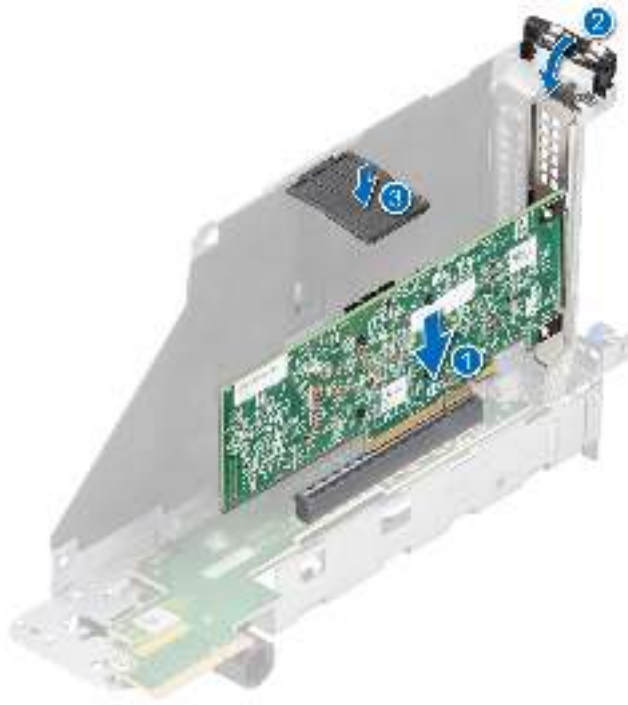
Figure 95. Installing an expansion card into the expansion card riser
