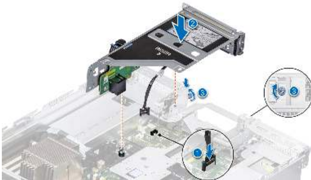
Figure 127. Connecting the serial COM port
