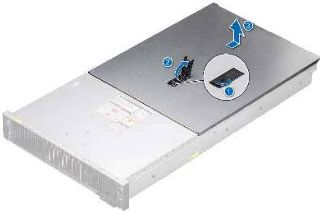
Figure 23. Removing the system cover
