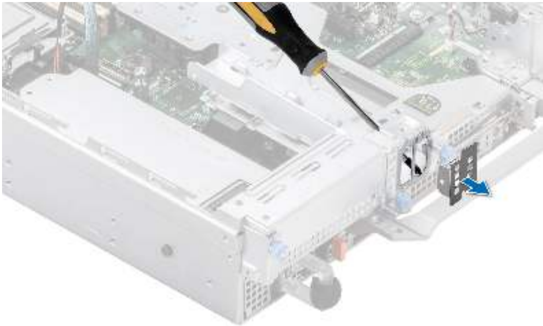
Figure 178. Removing the BOSS S2 module blank
