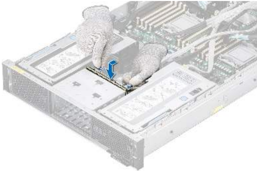
Figure 51. Installing the drive backplane
