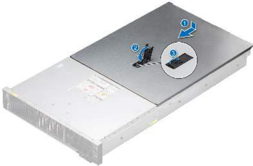
Figure 24. Installing the system cover
