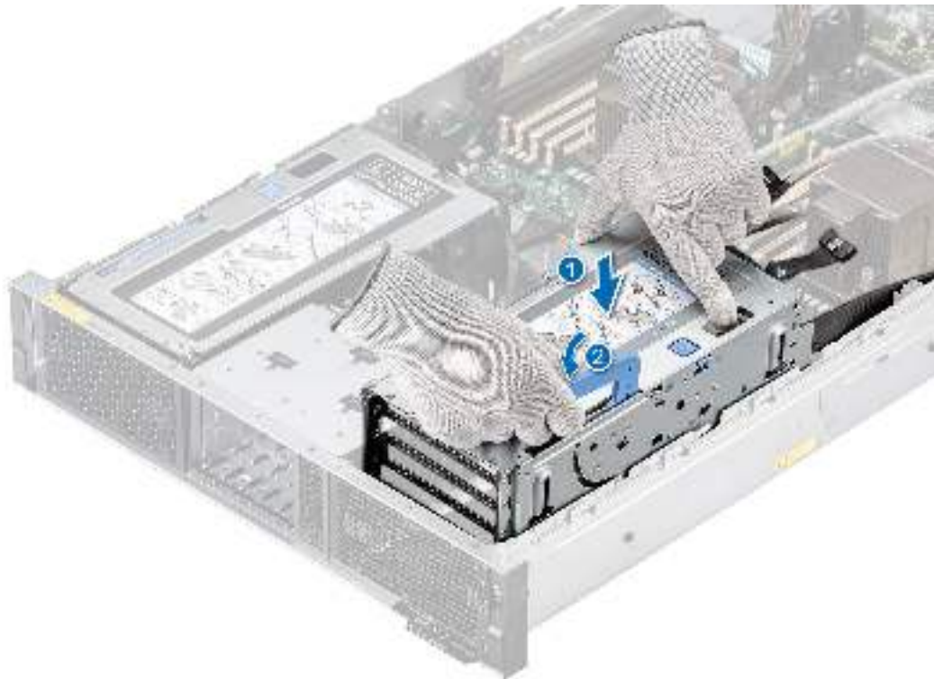
Figure 108. Installing the right GPU riser module
