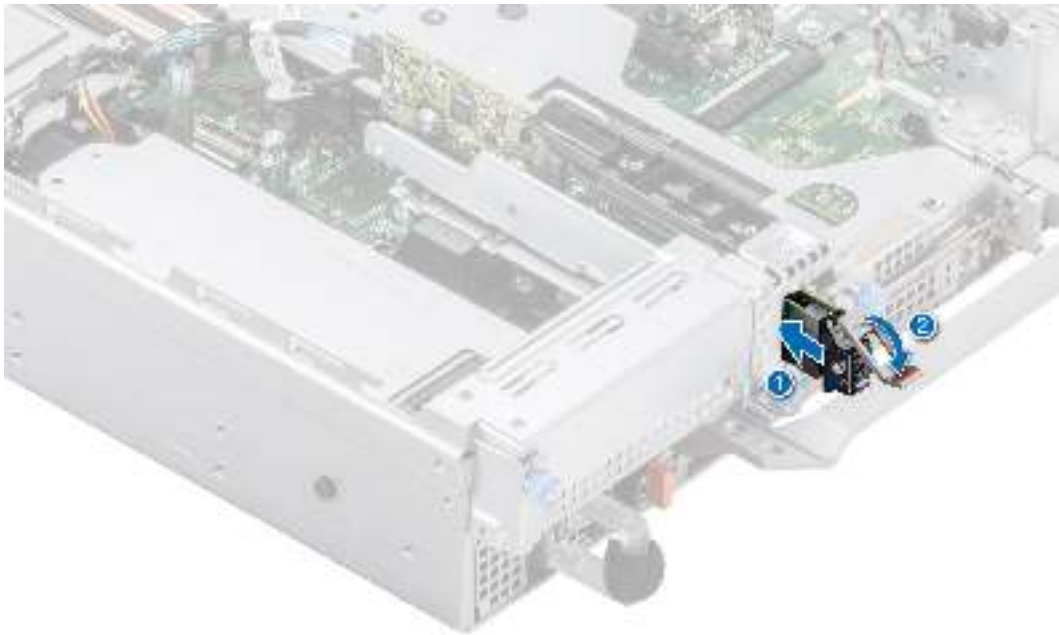
Figure 150. Installing the BOSS S2 card carrier
