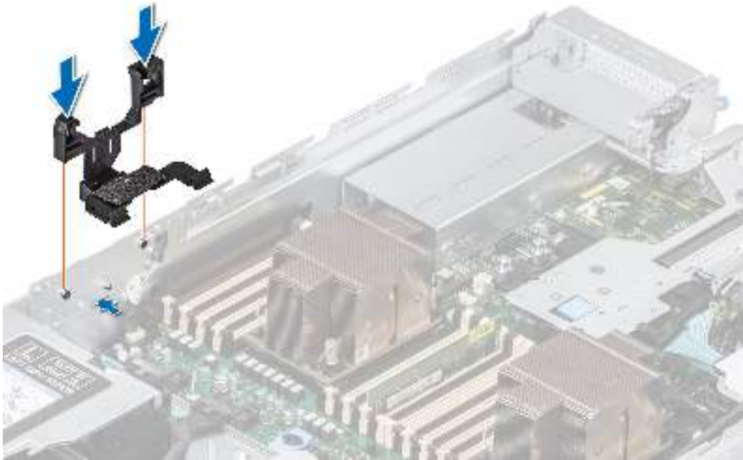
Figure 38. Installing the side wall bracket
