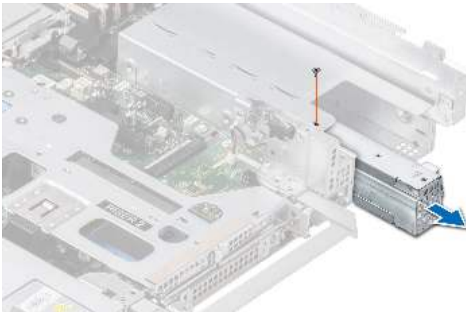
Figure 163. Removing a power supply unit adapter
