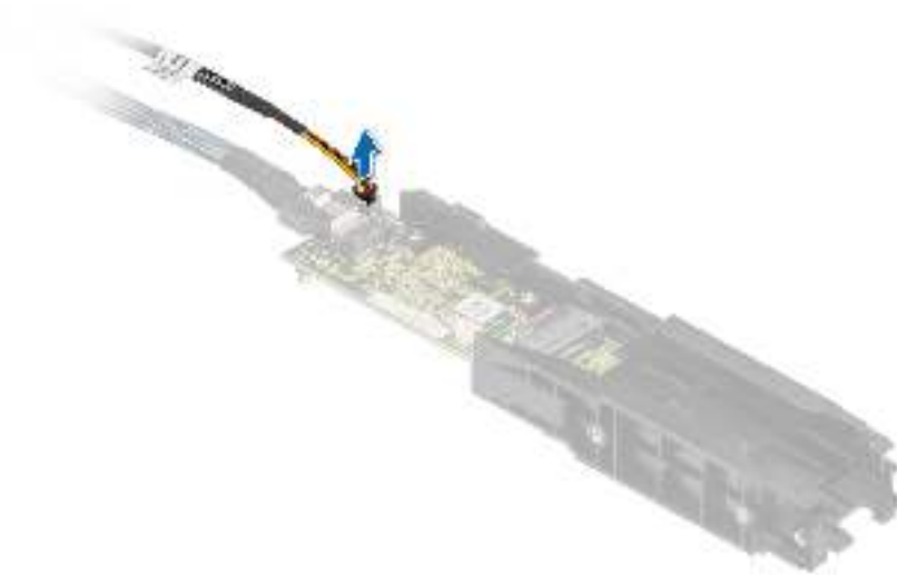
Figure 81. Disconnecting the BOSS S2 power cable
