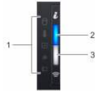
Figure 4. Left control panel with optional iDRAC Quick Sync 2 indicator
