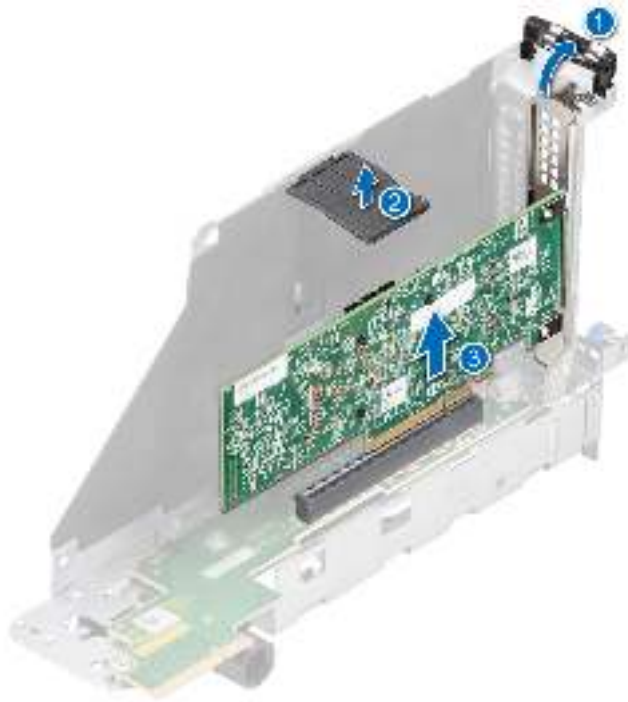
Figure 92. Removing expansion card from the expansion card riser
