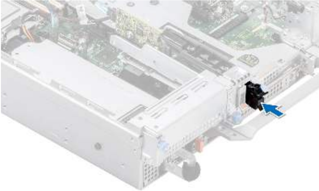
Figure 141. Installing the BOSS S2 card carrier blank
