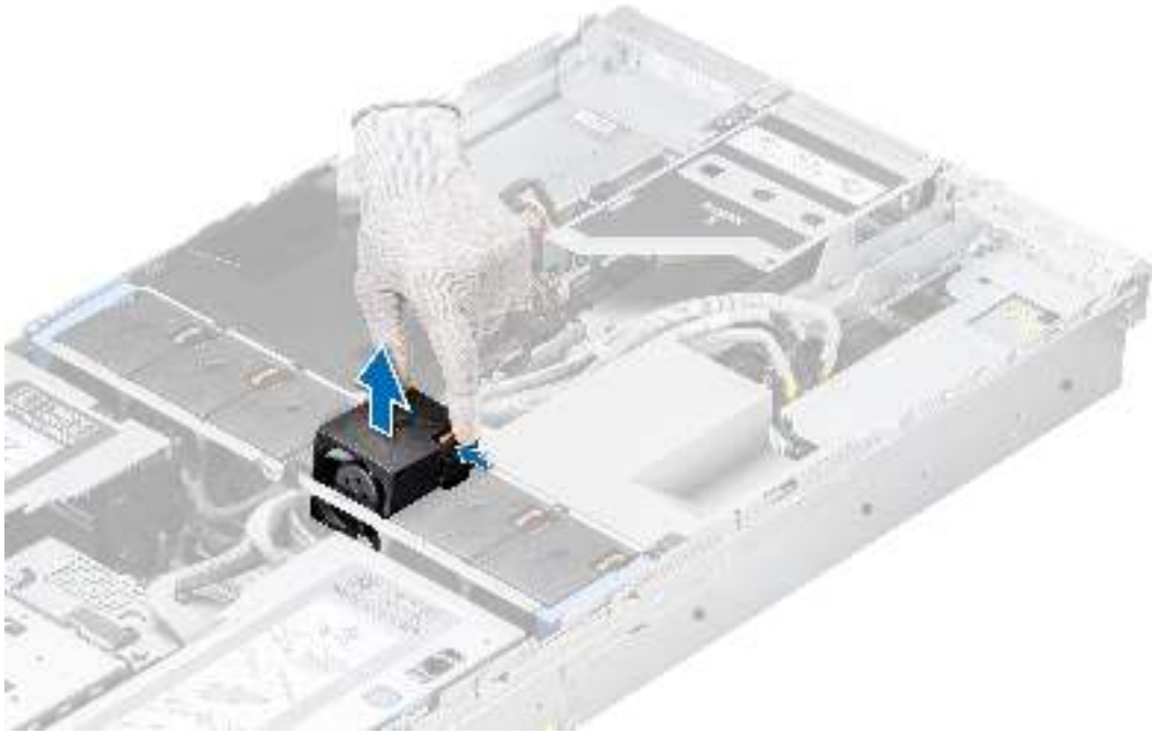
Figure 35. Removing a cooling fan
