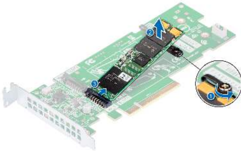
Figure 136. Removing the M.2 SSD module
