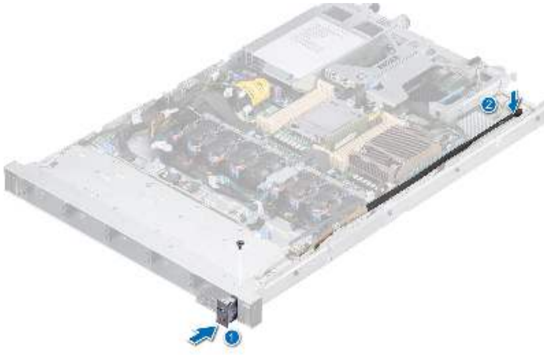
Figure 118. Installing the VGA module
