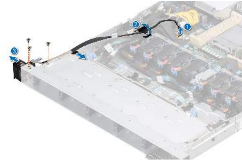
Figure 128. Removing the left control panel
