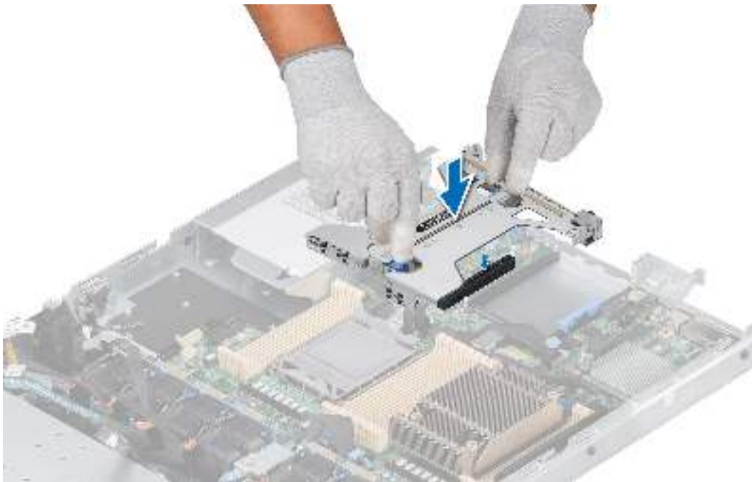
Figure 76. Installing the Riser 2c
