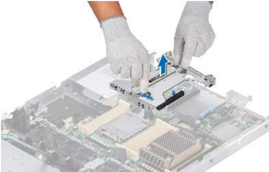
Figure 72. Removing the Riser 2c
