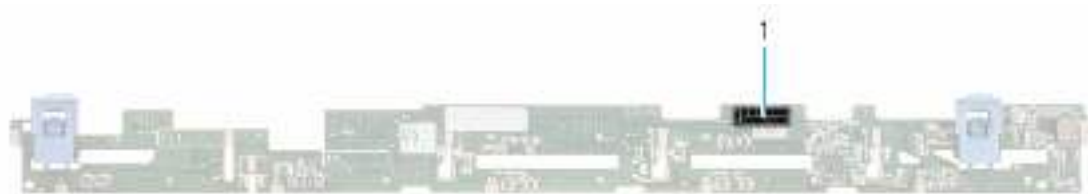
Figure 33. 8 x 2.5-inch drive backplane
