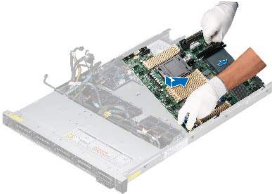
Figure 126. Installing the system board
