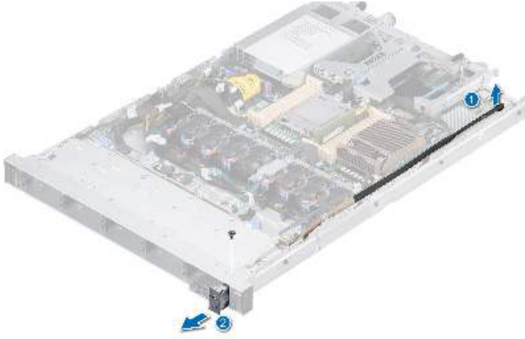
Figure 117. Removing the VGA module
