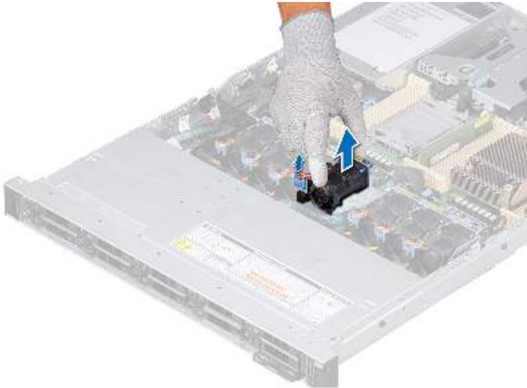
Figure 20. Removing a cooling fan
