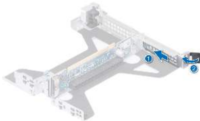
Figure 83. Installing filler bracket in the Riser 2b (SNAPI)
