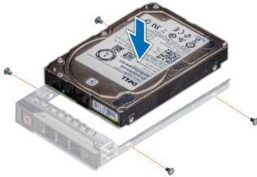
Figure 29. Installing a drive into the drive carrier
