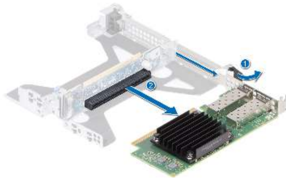
Figure 79. Removing an expansion card from Riser 2b (SNAPI)
