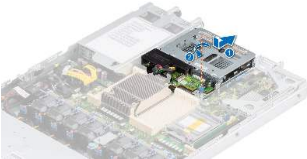
Figure 94. Installing the 2.5-inch rear drive cage
