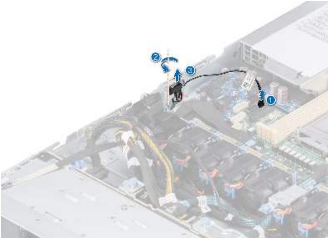
Figure 22. Removing the intrusion switch module
