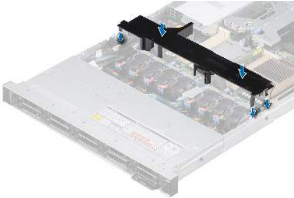
Figure 19. Installing the air shroud
