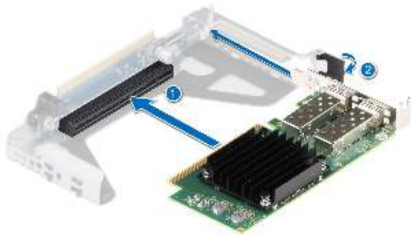
Figure 89. Installing an expansion card into a Riser 1
