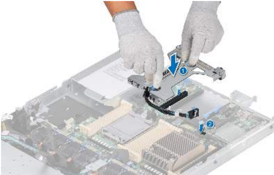
Figure 75. Installing the Riser 2b with SNAPI module
