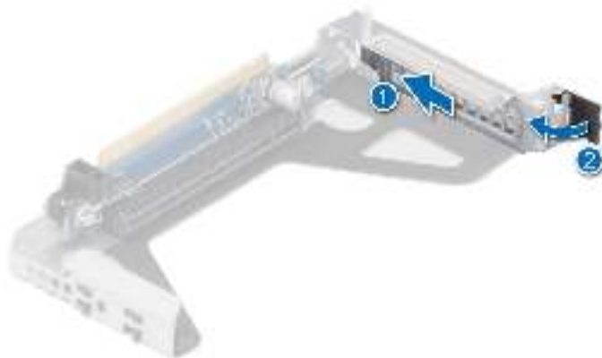
Figure 81. Installing filler bracket in the Riser 1
