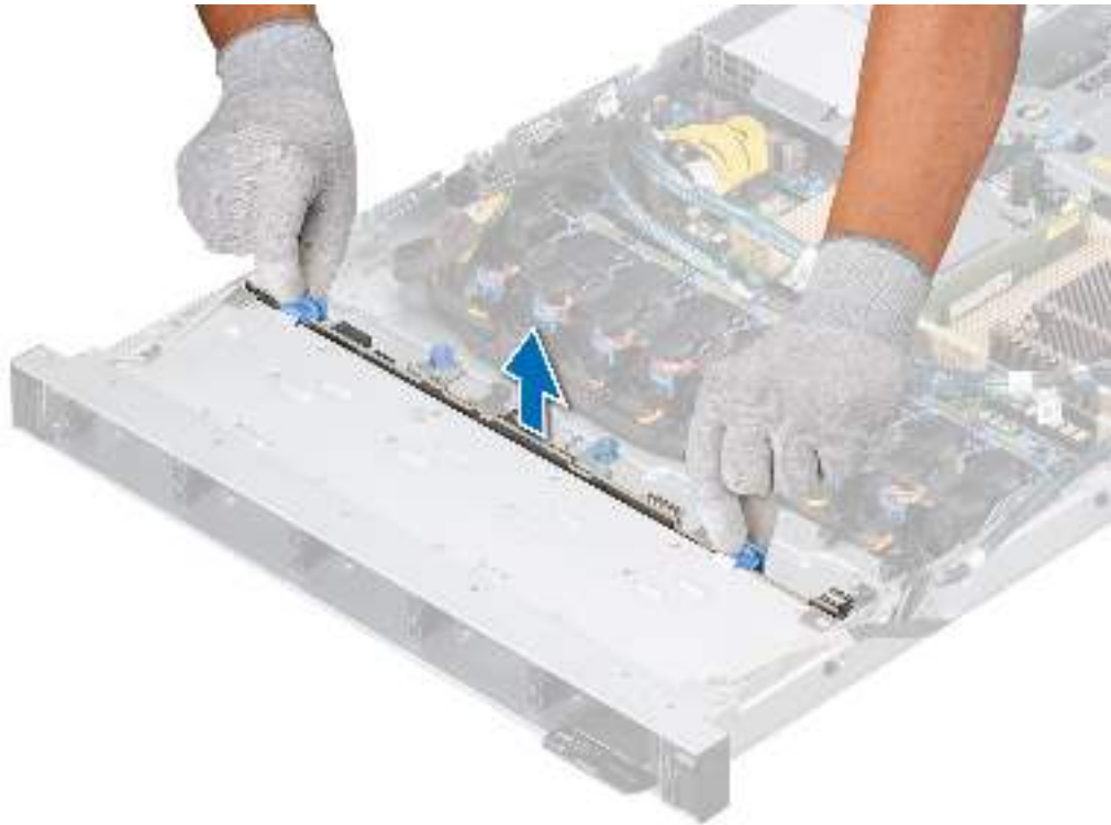
Figure 35. Removing the backplane
