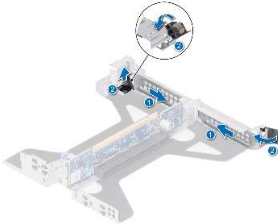
Figure 82. Installing filler bracket in the Riser 2a
