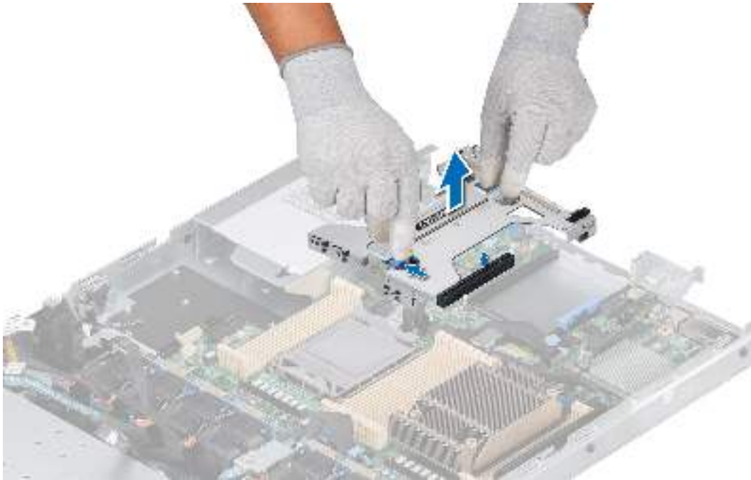
Figure 70. Removing the Riser 2a
