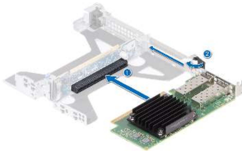
Figure 91. Installing an expansion card into a Riser 2b (SNAPI)
