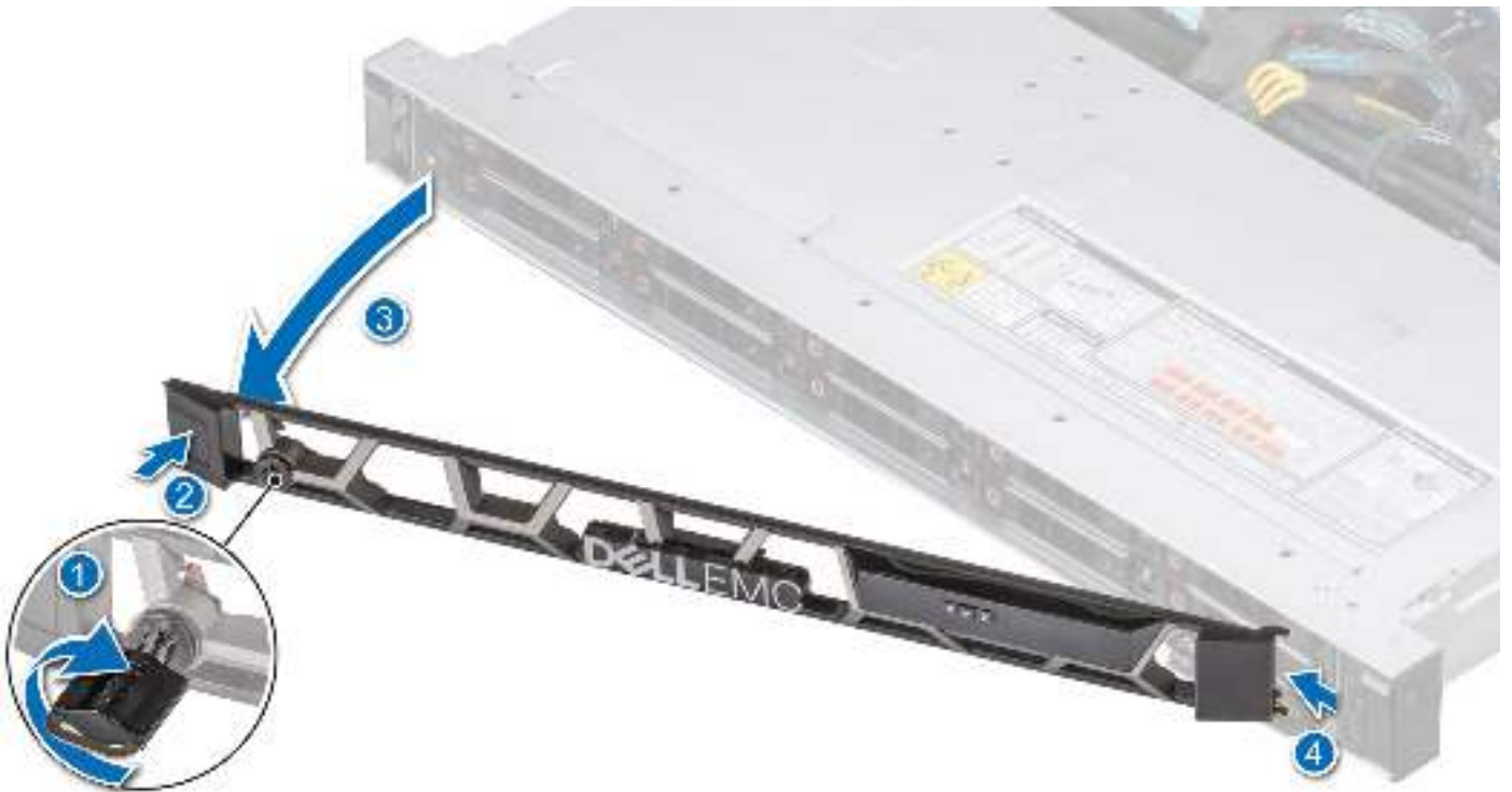
Figure 12. Removing the front bezel with the LCD panel
