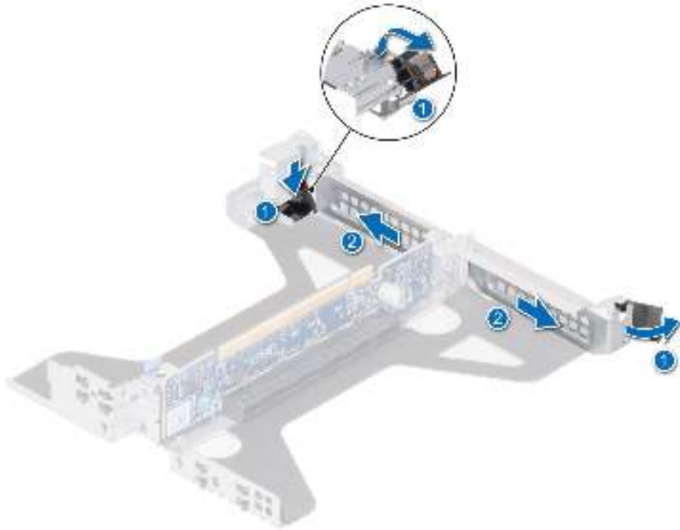
Figure 86. Removing filler bracket from Riser 2a
