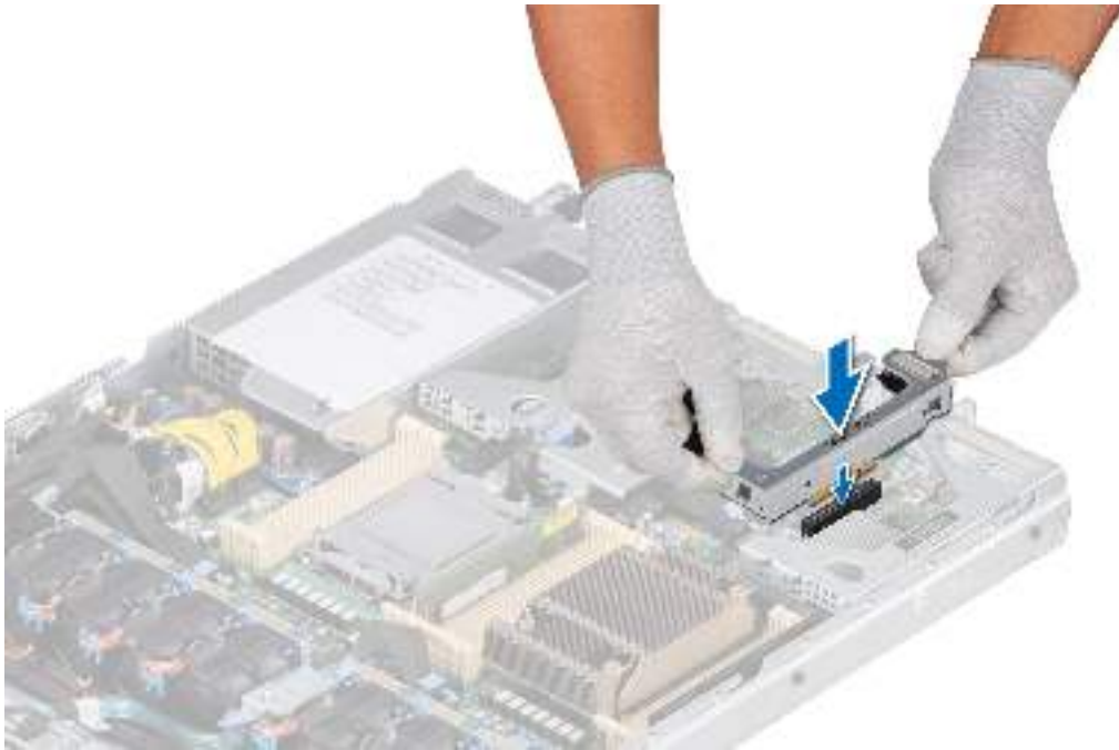
Figure 102. Installing the M.2 BOSS riser
