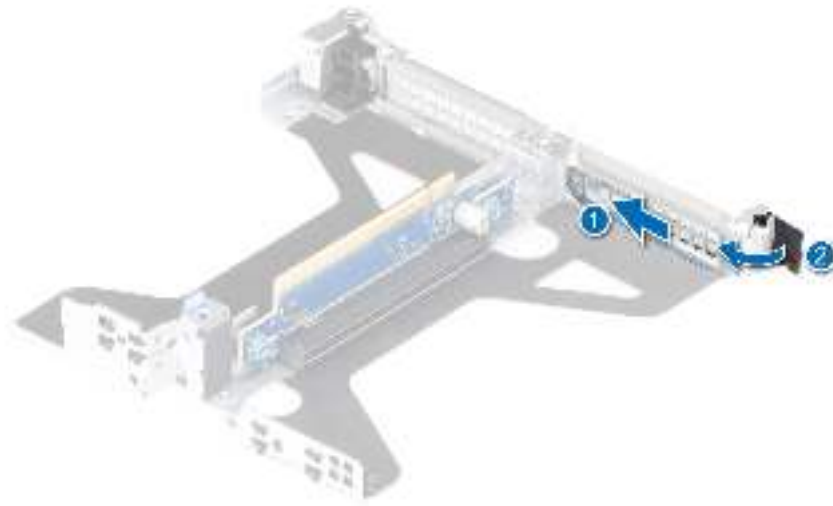
Figure 84. Installing filler bracket in the Riser 2c
