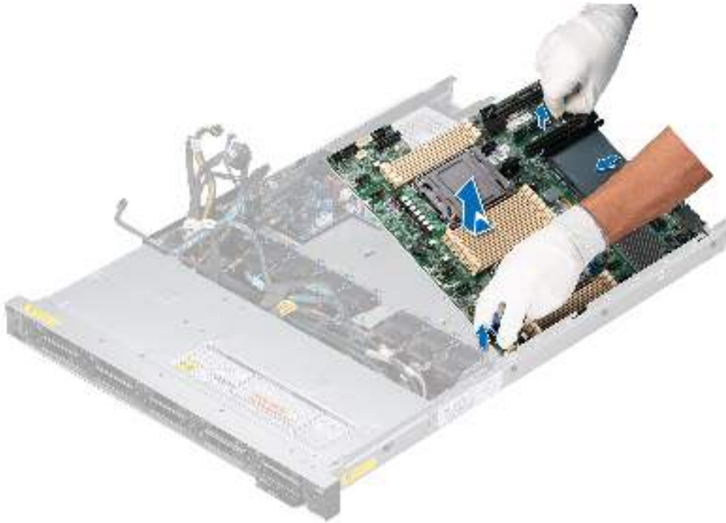
Figure 125. Removing the system board
