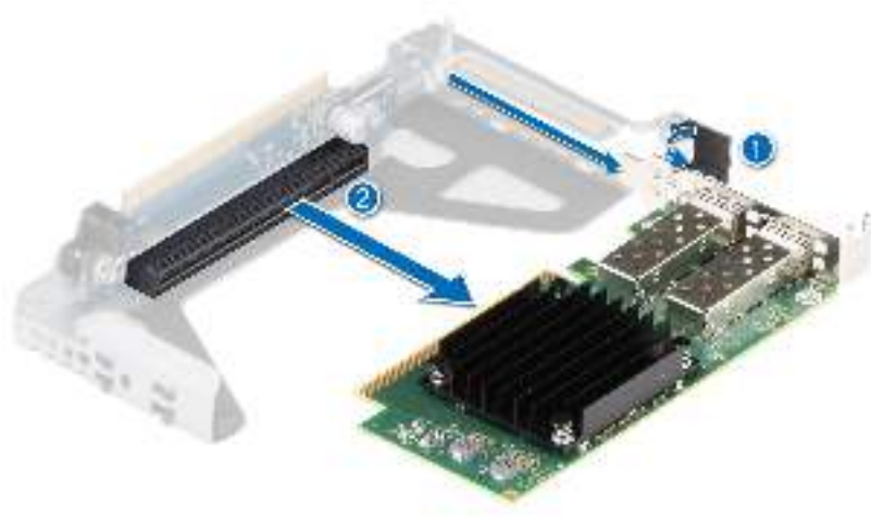
Figure 77. Removing an expansion card from the Riser 1
