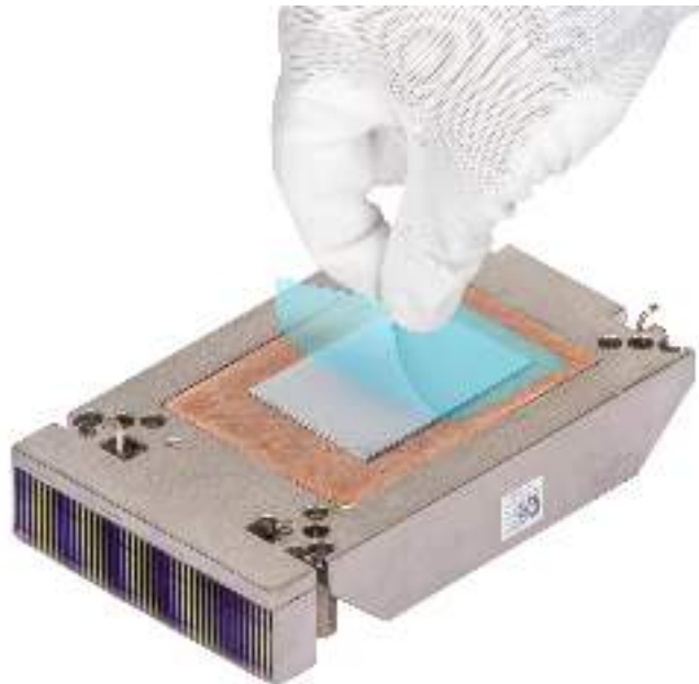
Figure 60. Remove the Thermal Interface Material (TIM) protective film
