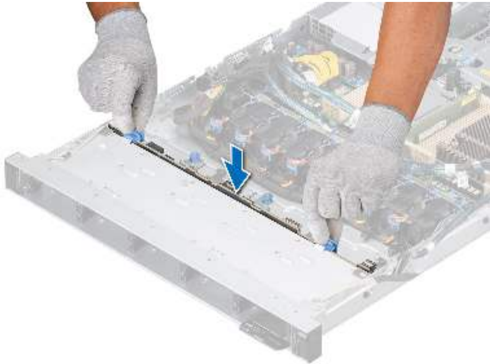
Figure 36. Installing the drive backplane
