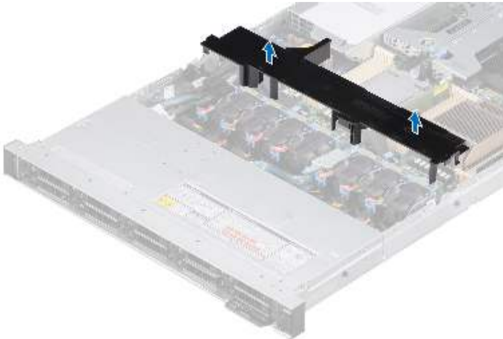
Figure 18. Removing the air shroud
