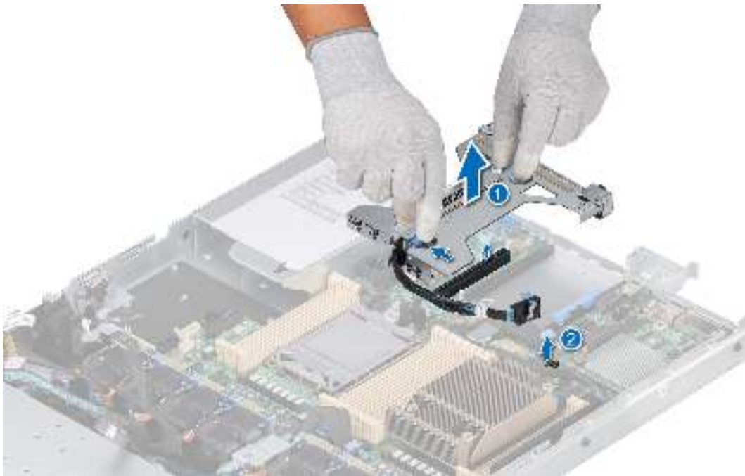
Figure 71. Removing the Riser 2b with SNAPI module
