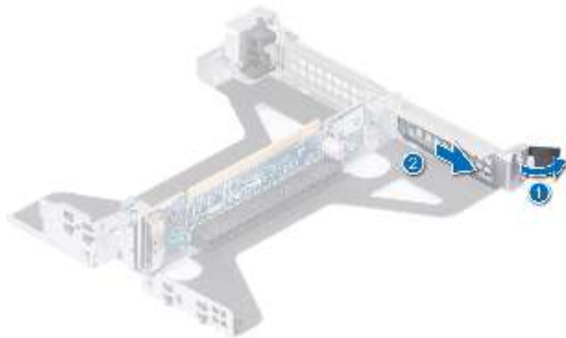
Figure 87. Removing filler bracket from Riser 2b (SNAPI)
