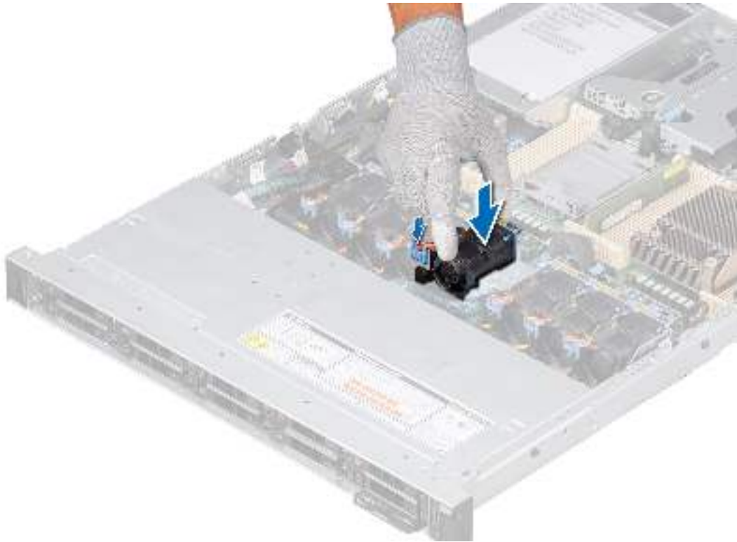
Figure 21. Installing a cooling fan
