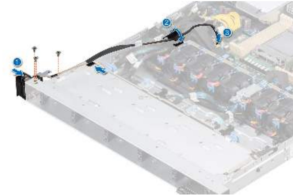
Figure 129. Installing the left control panel
