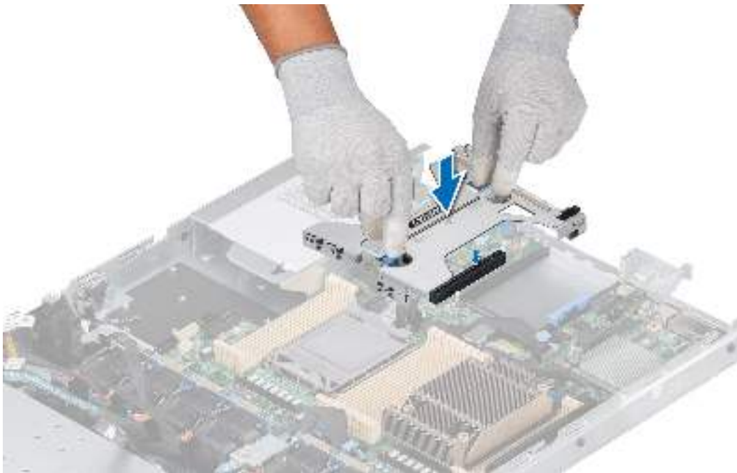
Figure 74. Installing the Riser 2a
