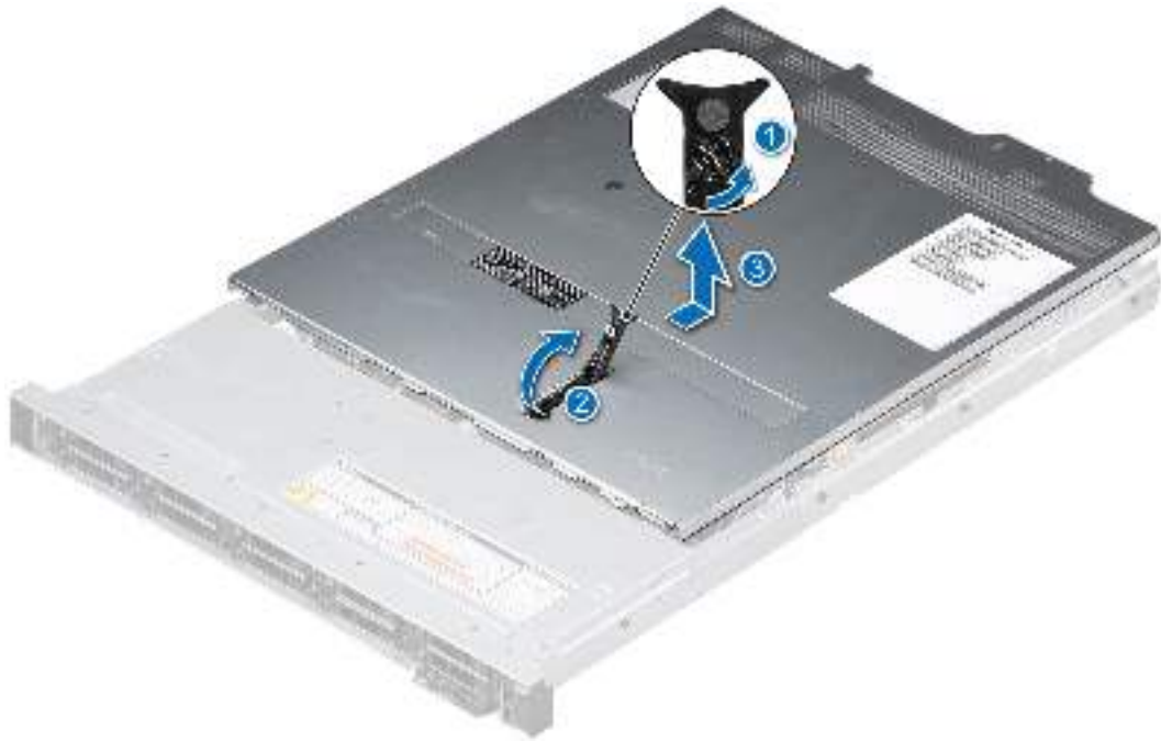
Figure 14. Removing the system cover
