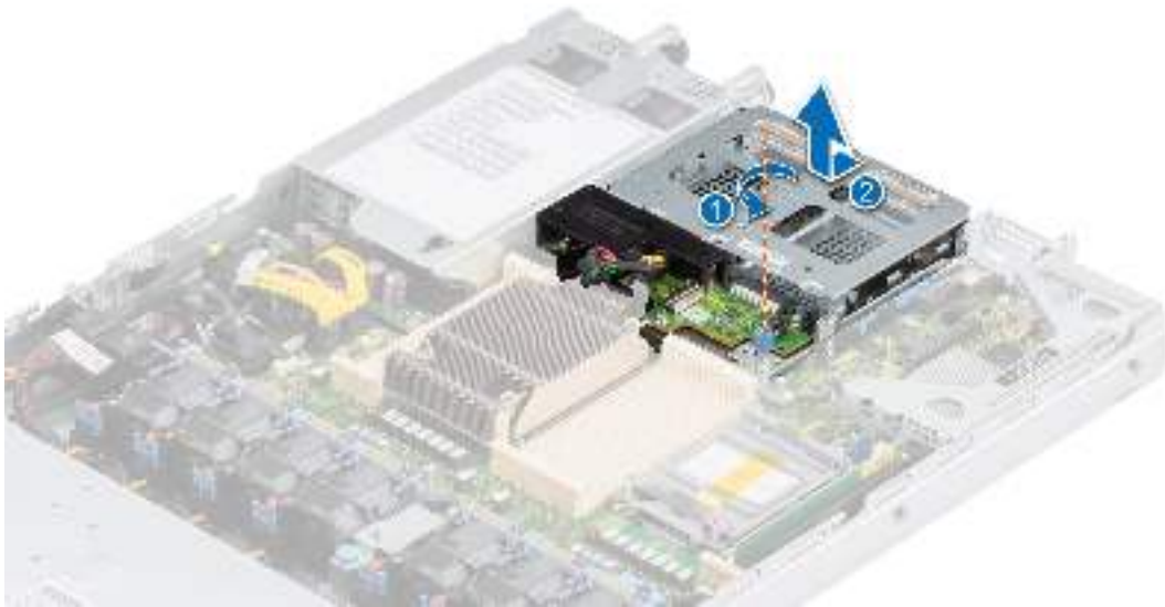
Figure 93. Removing the 2.5-inch rear drive cage
