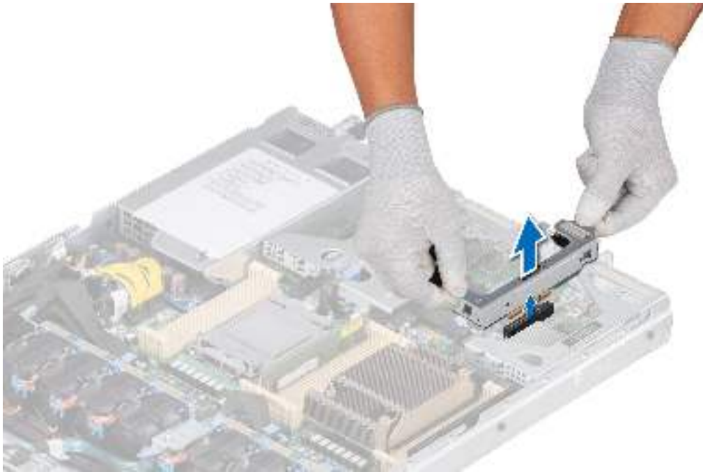
Figure 101. Removing the M.2 BOSS riser
