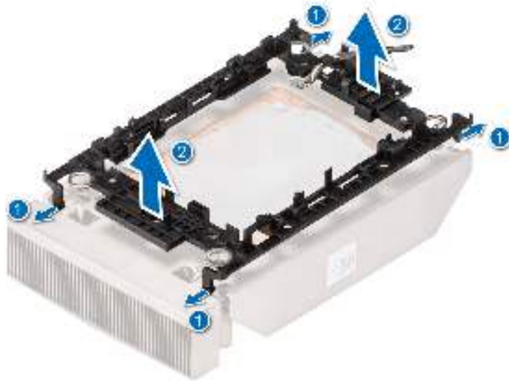
Figure 56. Removing the processor carrier
