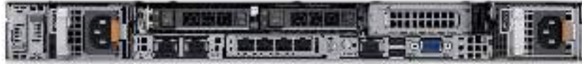
Figure 6. Rear view of the R650 with 2x 2.5 inches Storage drives, 1x LP PCIe Gen4 slot and Hot-plug BOSS
