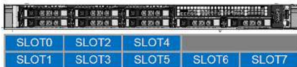
Figure 2. Front view of the R650, 8x 2.5 inches SAS/SATA Chassis
