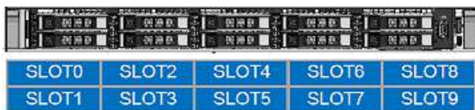
Figure 4. Front View of the R650, 10x 2.5 inches SAS/SATA or NVMe
