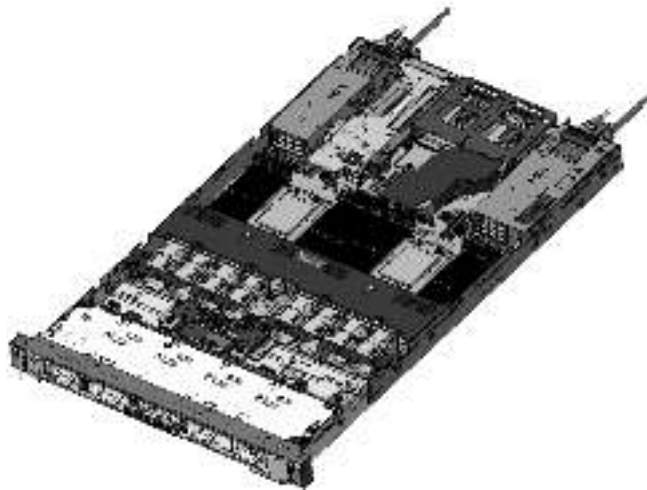
Figure 10. Inside the system, R650 with 2x Rear drives and 1 PCIe Gen4 slot
