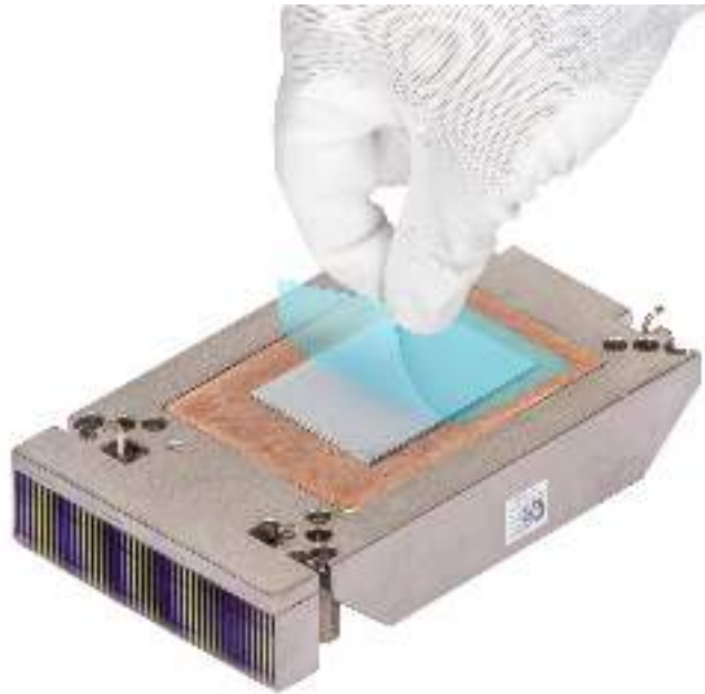
Figure 63. Remove the Thermal Interface Material (TIM) protective film
