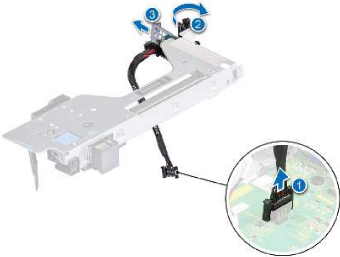
Figure 124. Removing the serial COM port
