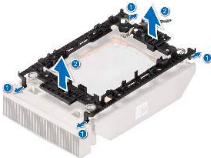
Figure 59. Removing the processor carrier
