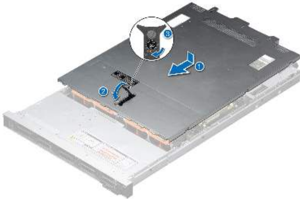
Figure 27. Installing the system cover
