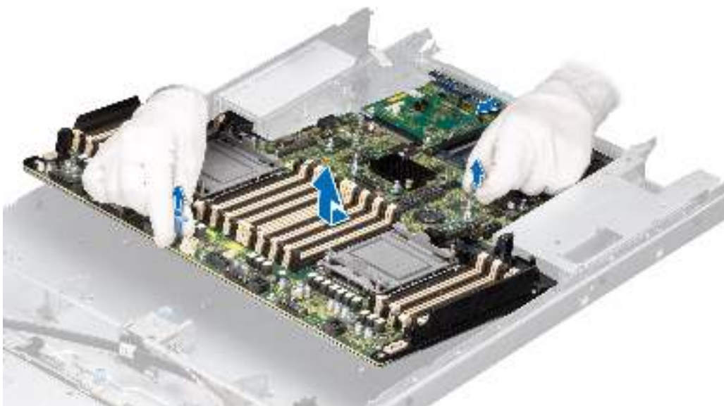
Figure 128. Removing the system board
