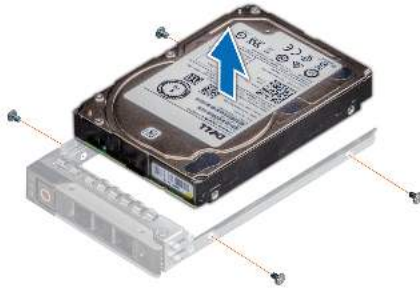
Figure 40. Removing the drive from the drive carrier
