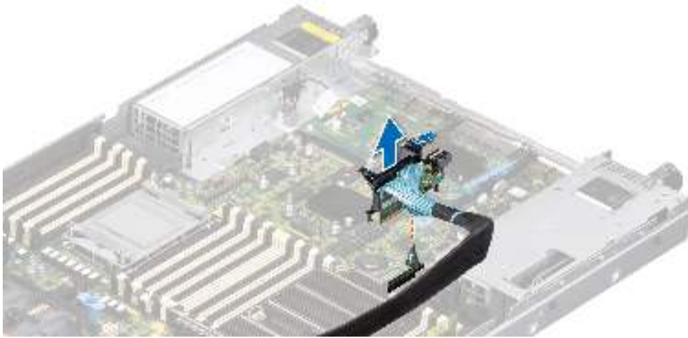
Figure 86. Removing the R1 paddle card
