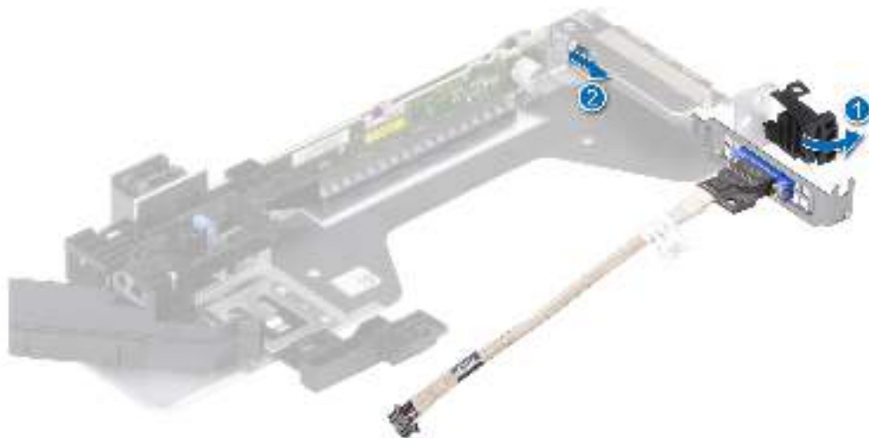
Figure 116. Removing the VGA port
