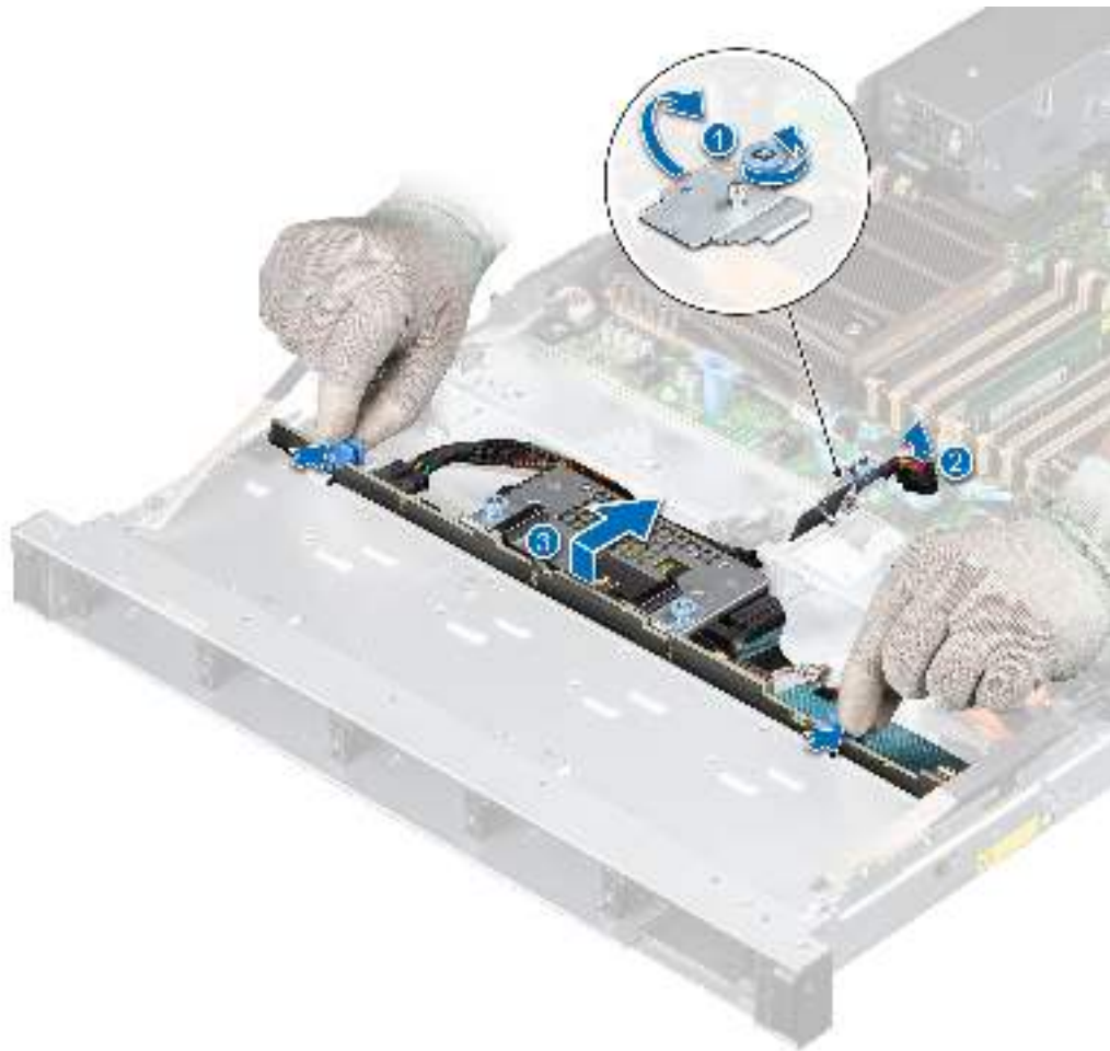
Figure 45. Removing the drive backplane
