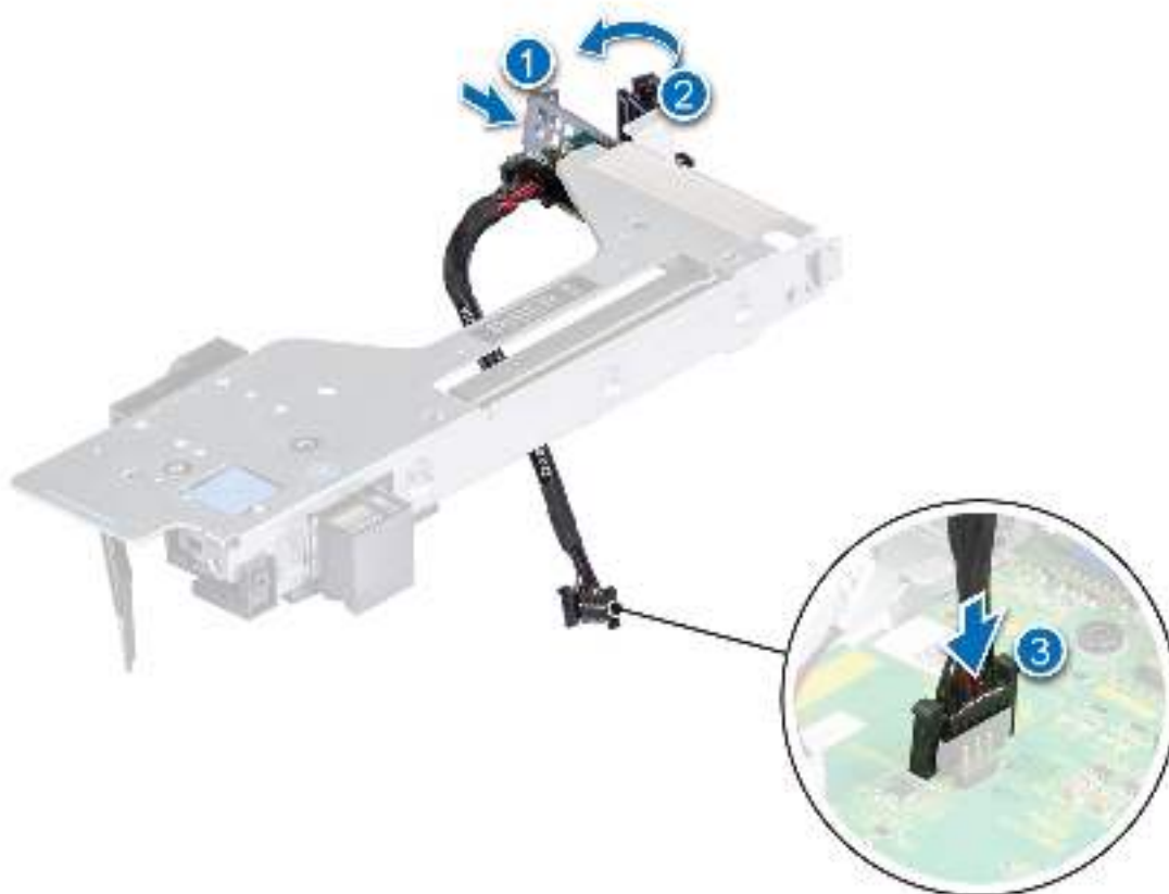
Figure 127. Installing the serial COM port
