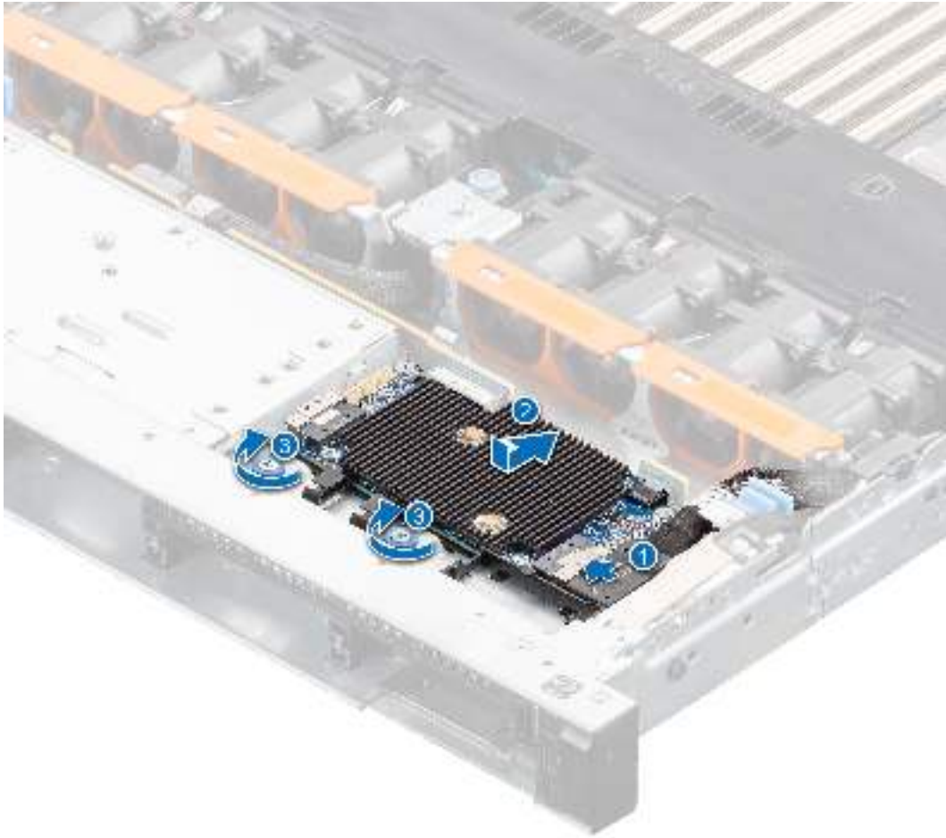
Figure 48. Installing the front mounting front PERC module
