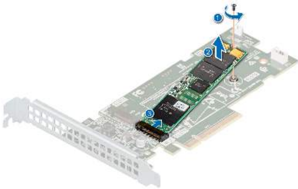
Figure 90. Removing the M.2 SSD module
