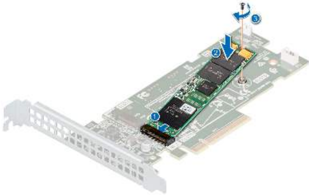
Figure 91. Installing the M.2 SSD module
