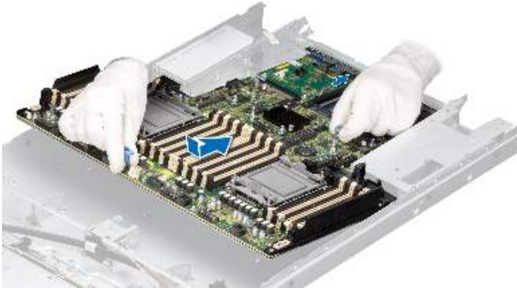
Figure 129. Installing the system board
