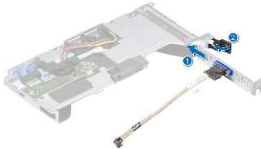
Figure 119. Installing the rear VGA port
