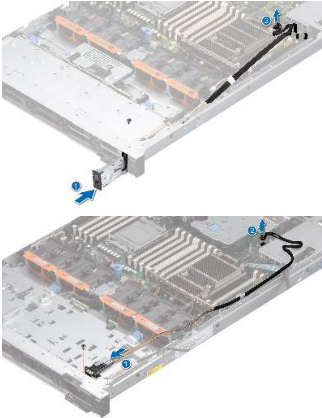
Figure 115. Installing the VGA module
