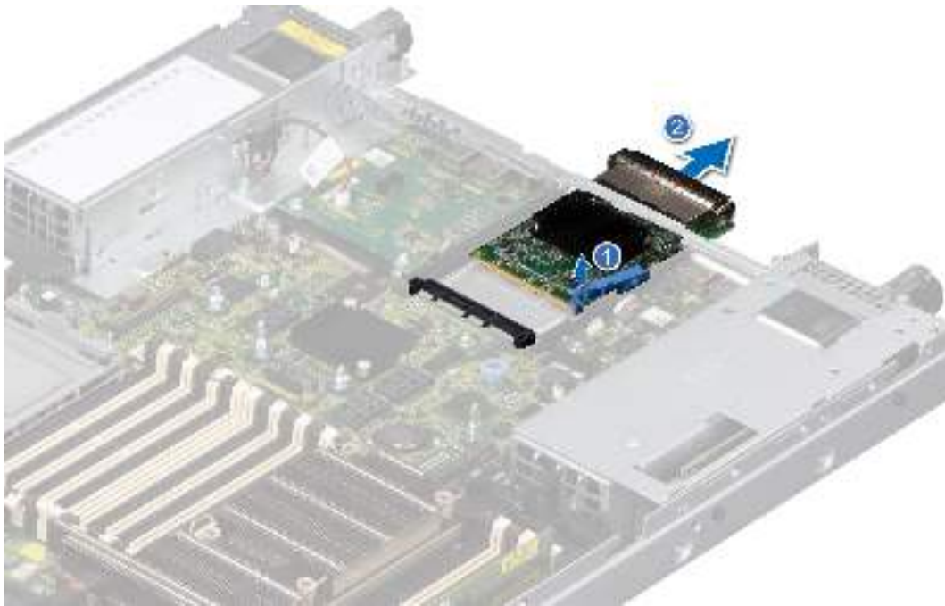
Figure 108. Removing the OCP card
