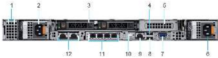
Figure 9. Rear view of the system with 2 x 2.5-inch rear drive module and 1 x LP PCIe slot
