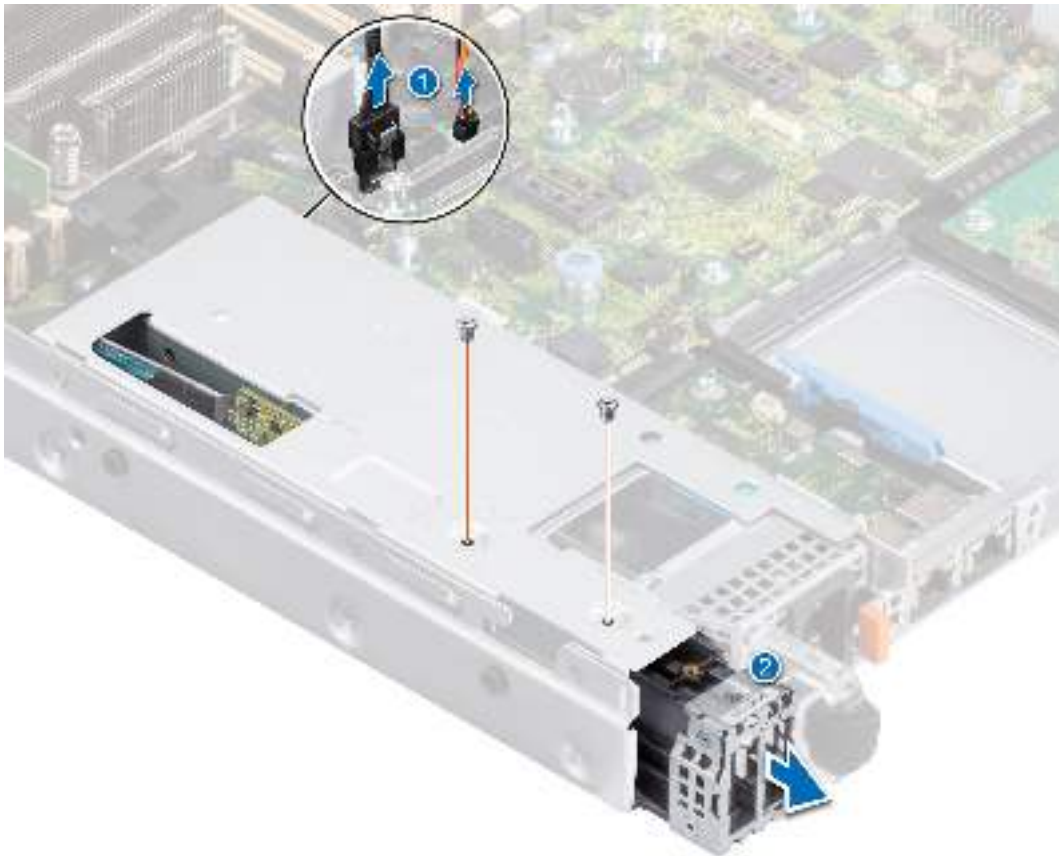
Figure 96. Removing the BOSS S2 module
