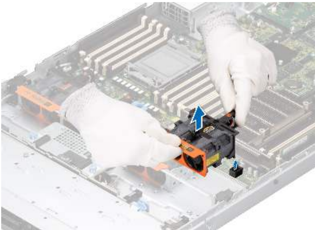
Figure 34. Removing a cooling fan module
