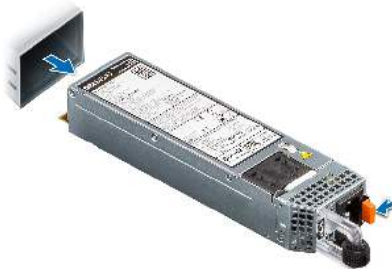
Figure 122. Removing a power supply unit
