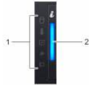
Figure 5. Left control panel without optional iDRAC Quick Sync 2.0 indicator
