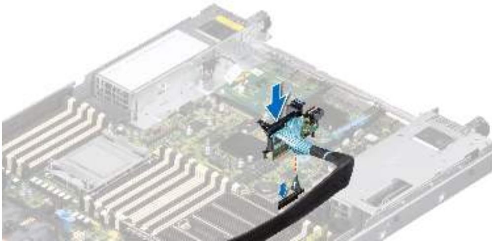
Figure 87. Installing the R1 paddle card
