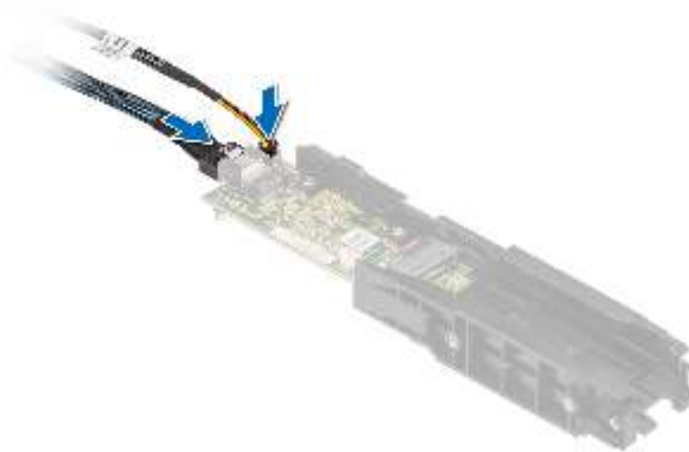
Figure 100. Connecting the BOSS power cable and BOSS Signal cable to the BOSS S2 module
