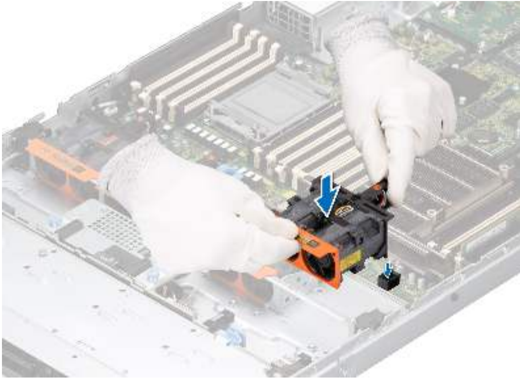
Figure 35. Installing a cooling fan module
