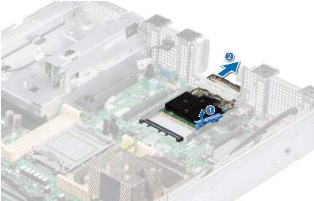
Figure 90. Removing the OCP card
