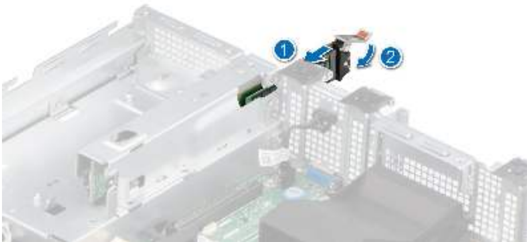
Figure 85. Installing the BOSS S2 card carrier
