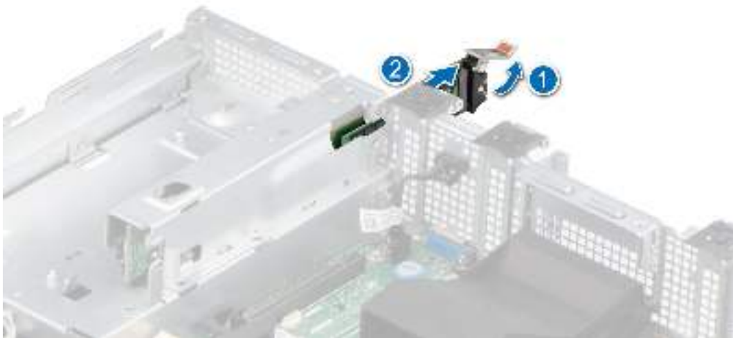
Figure 74. Removing the BOSS S2 card carrier
