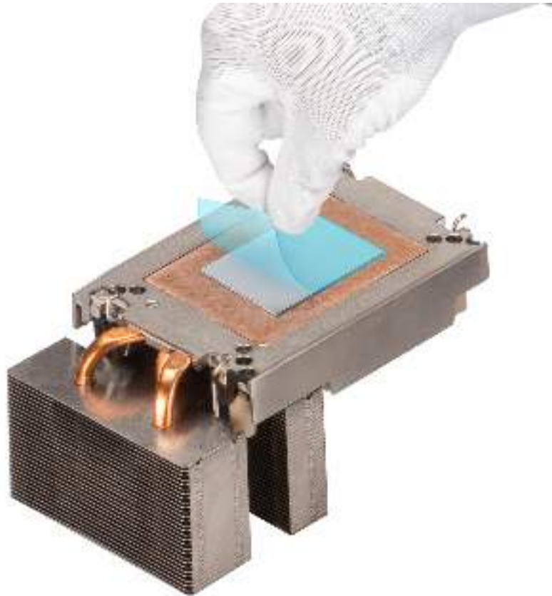
Figure 63. Remove the Thermal Interface Material (TIM) protective film
