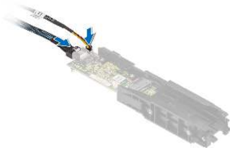
Figure 81. Connecting the BOSS power cable and BOSS Signal cable to the BOSS S2 module
