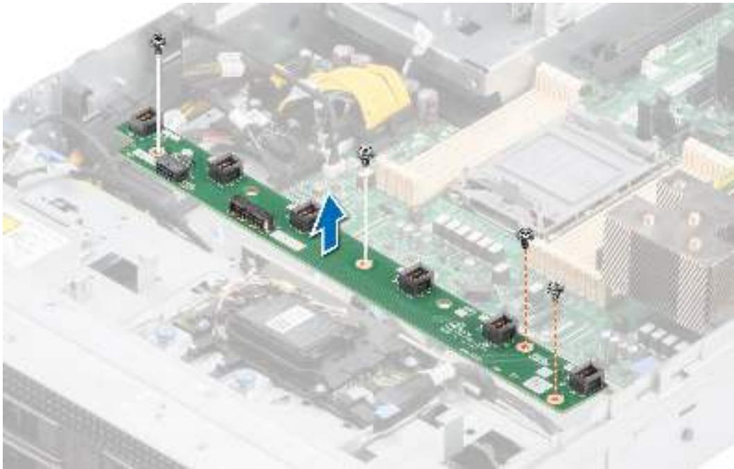
Figure 104. Removing the cooling fan cage board.
