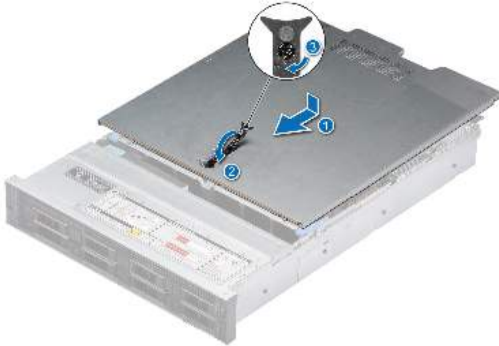
Figure 21. Installing the system cover
