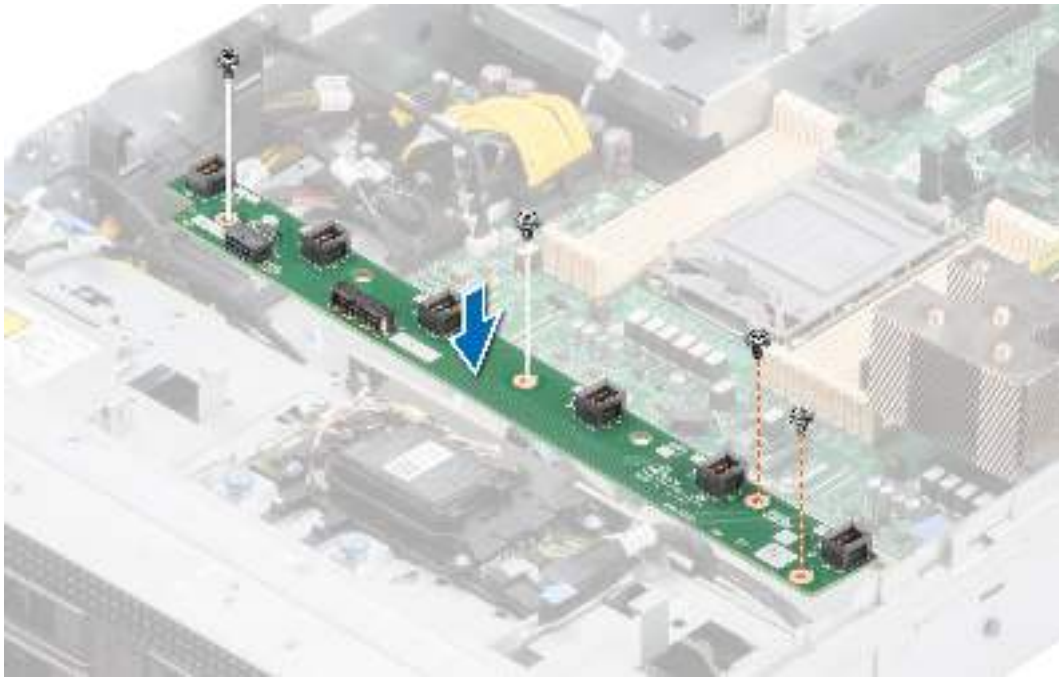
Figure 105. Installing the cooling fan cage board
