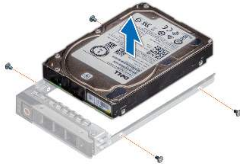
Figure 40. Removing the drive from the drive carrier
