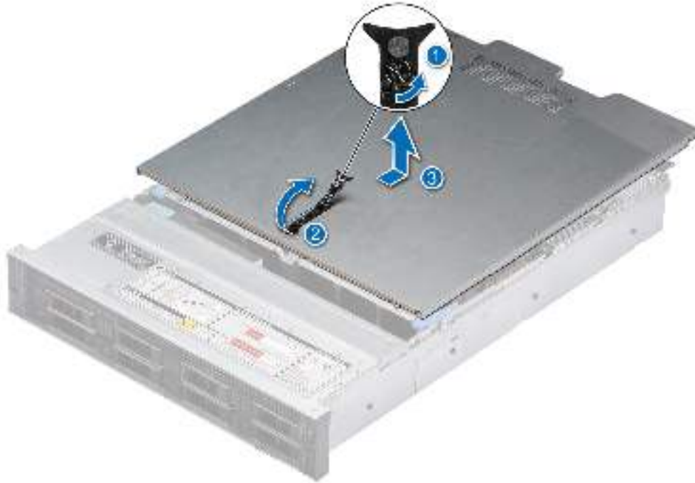
Figure 20. Removing the system cover
