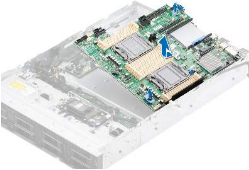
Figure 106. Removing the system board
