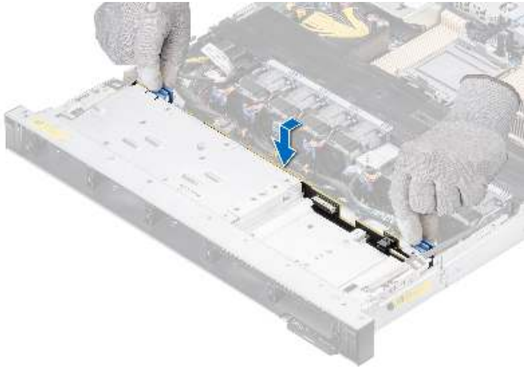
Figure 38. Installing the drive backplane
