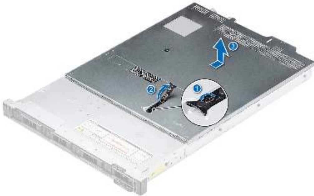
Figure 17. Removing the system cover
