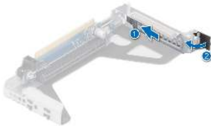
Figure 66. Installing filler bracket in the Riser 1
