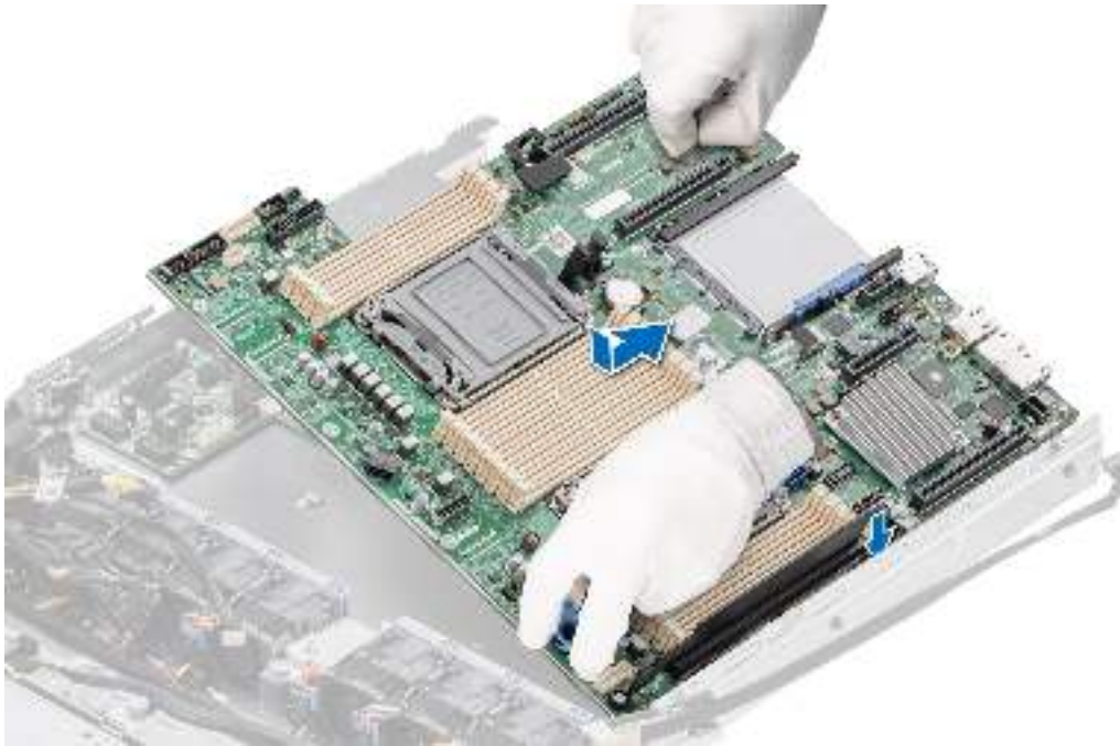
Figure 101. Installing the system board
