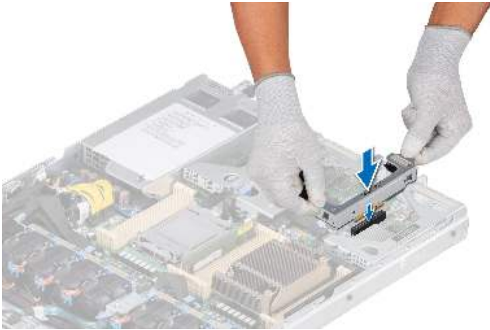
Figure 77. Installing the M.2 boss riser
