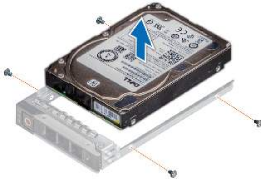
Figure 31. Removing the drive from the drive carrier
