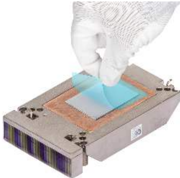
Figure 53. Remove the Thermal Interface Material (TIM) protective film
