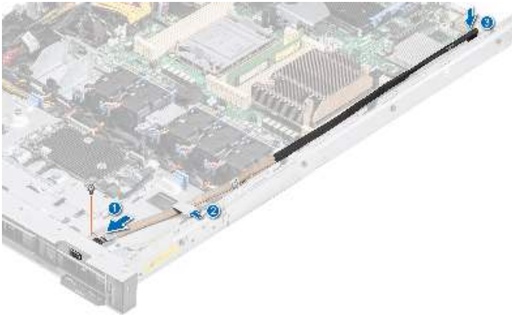
Figure 93. Installing the VGA module
