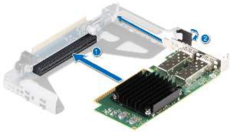
Figure 70. Installing an expansion card into a Riser 1
