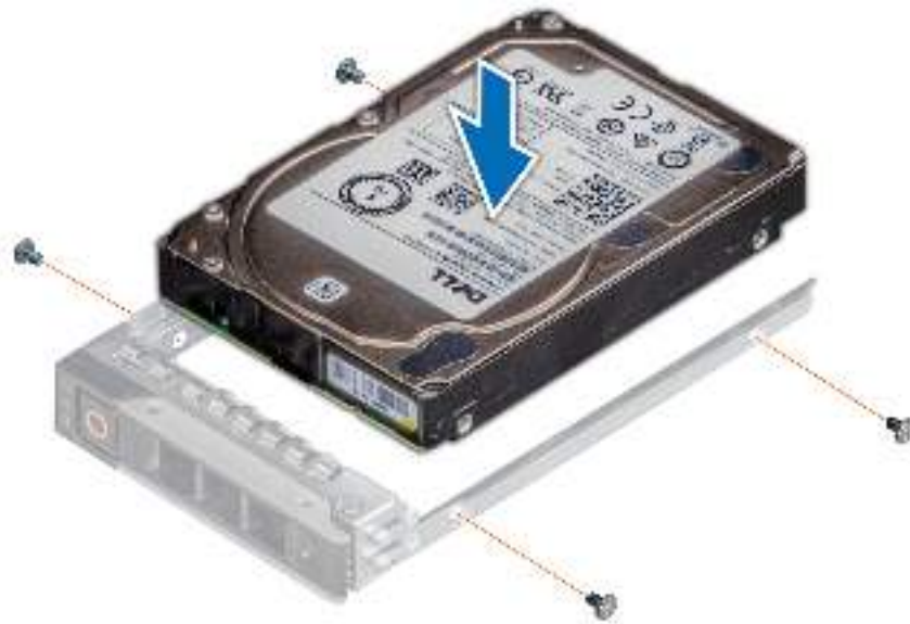
Figure 32. Installing a drive into the drive carrier
