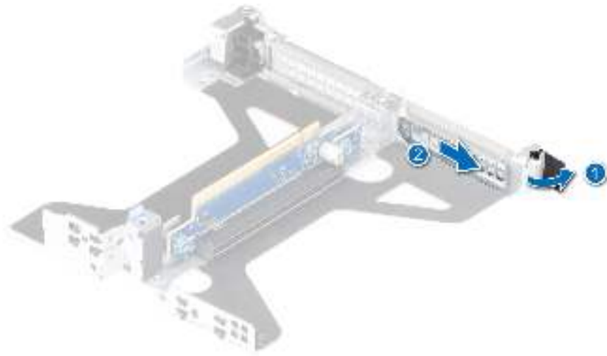
Figure 69. Removing filler bracket in the Riser 2c
