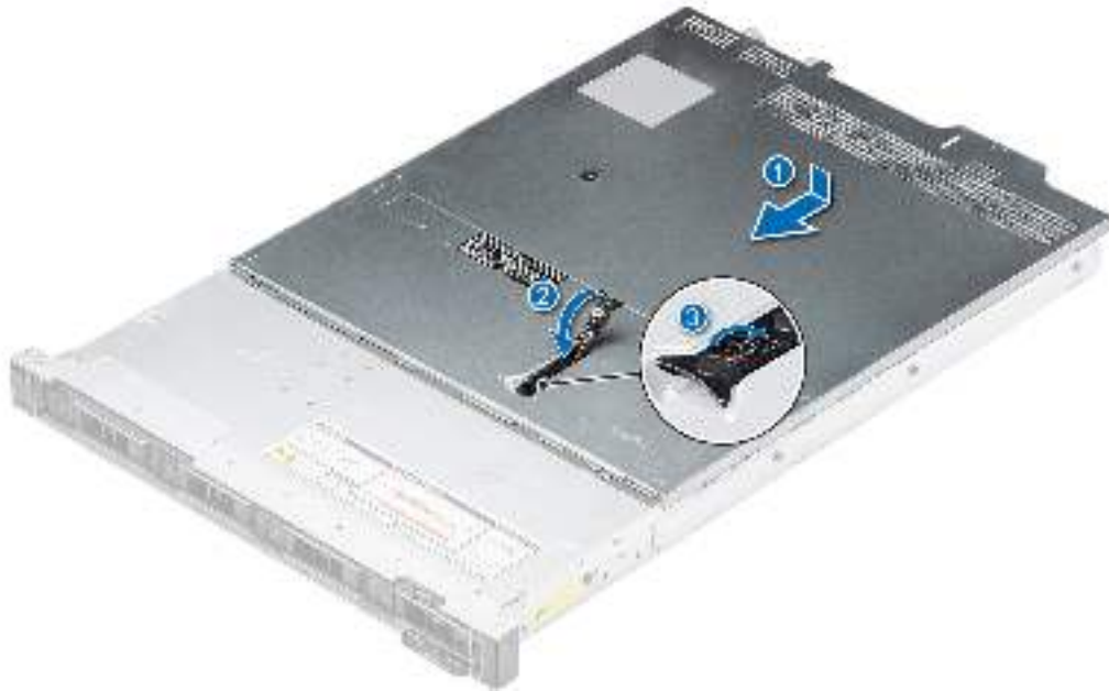
Figure 18. Installing the system cover
