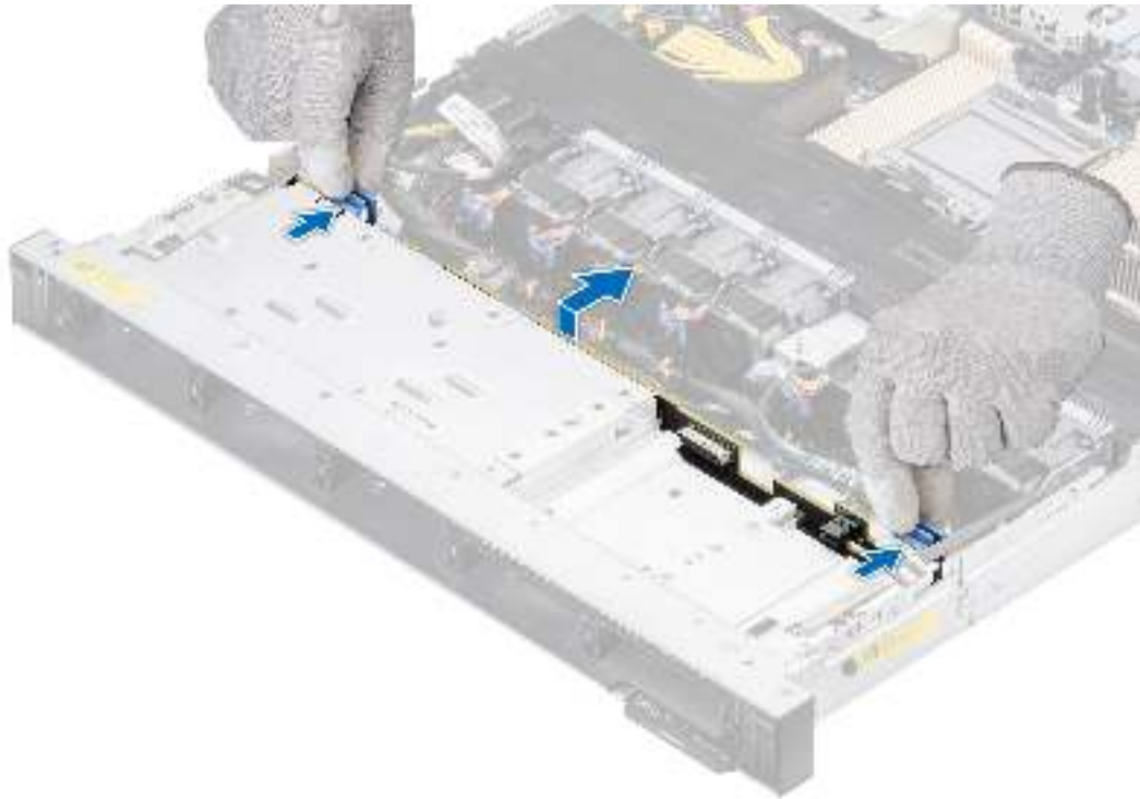
Figure 37. Removing the backplane
