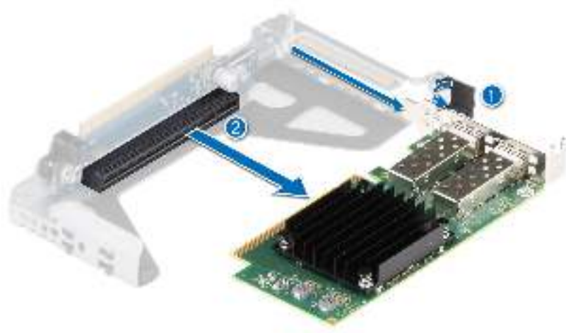
Figure 64. Removing an expansion card from the Riser 1
