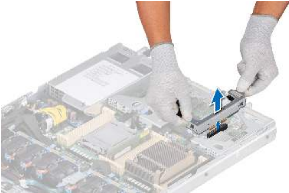
Figure 76. Removing the M.2 BOSS riser
