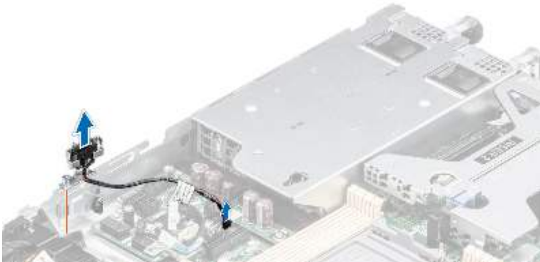
Figure 25. Removing the intrusion switch module
