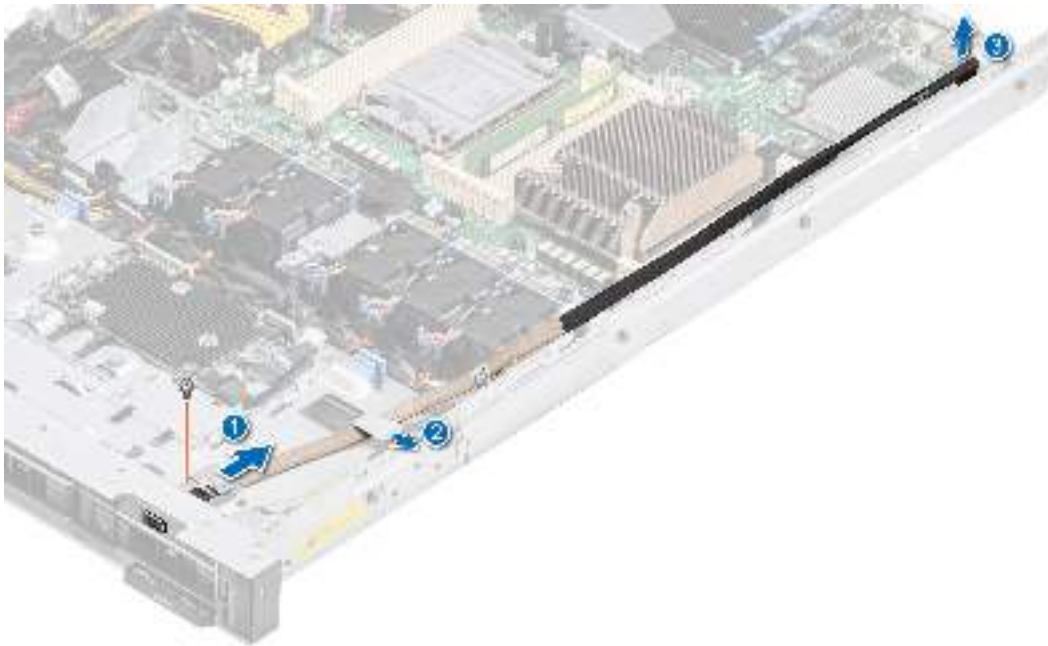
Figure 92. Removing the VGA module
