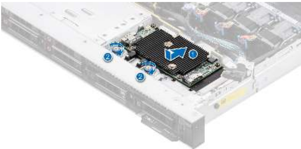
Figure 87. Installing the front mounting front PERC module for 8x2.5-inch system
