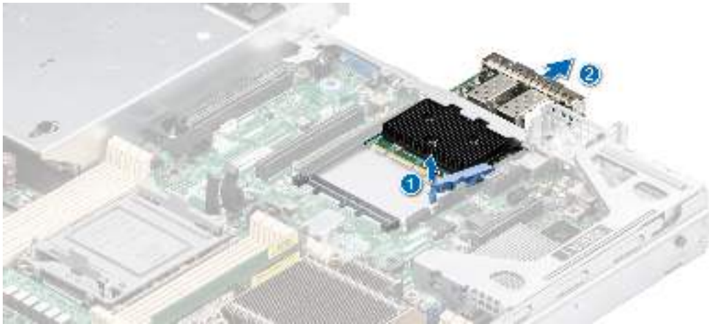
Figure 82. Removing the OCP card
