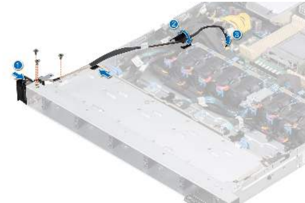
Figure 104. Installing the left control panel
