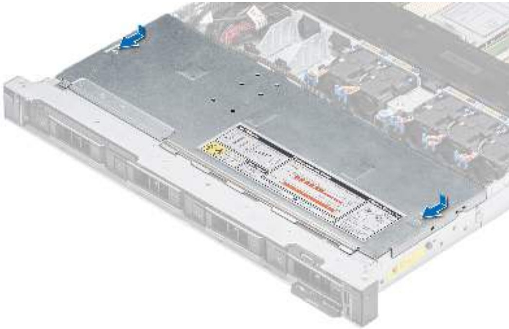
Figure 20. Installing the drive backplane cover
