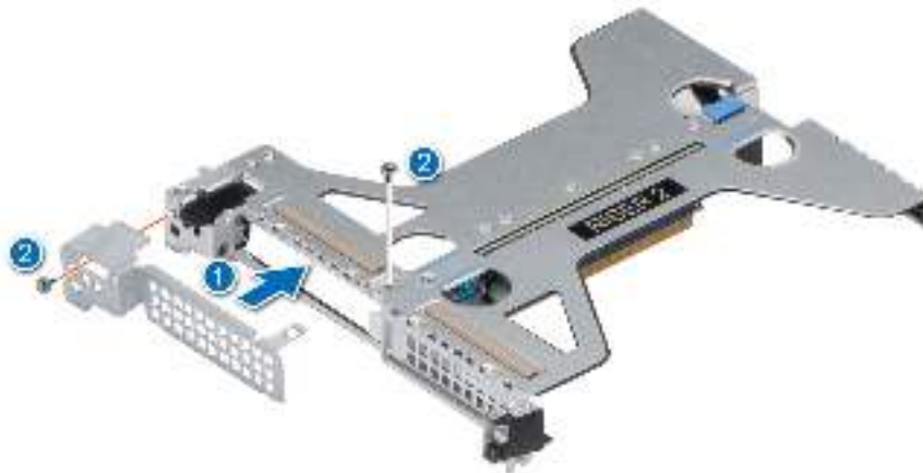
Figure 73. Installing the PCIe blank
