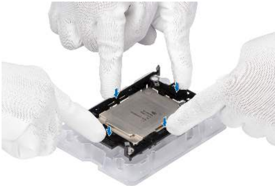
Figure 51. Press the carrier on the four sides
