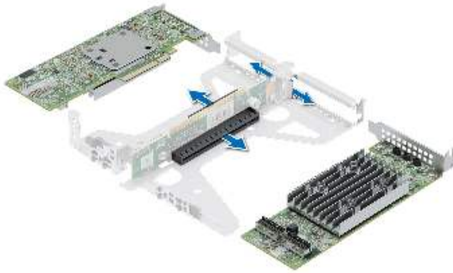
Figure 49. Removing an expansion card from riser
