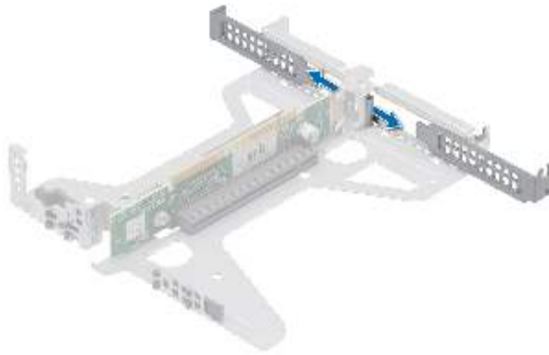
Figure 51. Removing filler bracket in the riser
