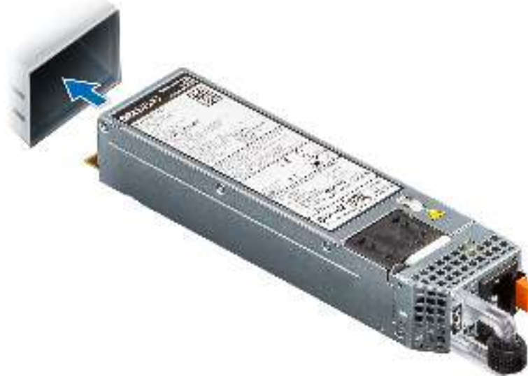
Figure 68. Installing a power supply unit
