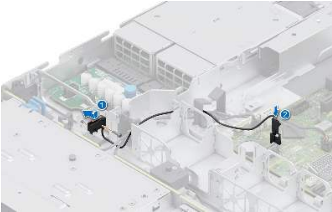
Figure 18. Installing the intrusion switch
