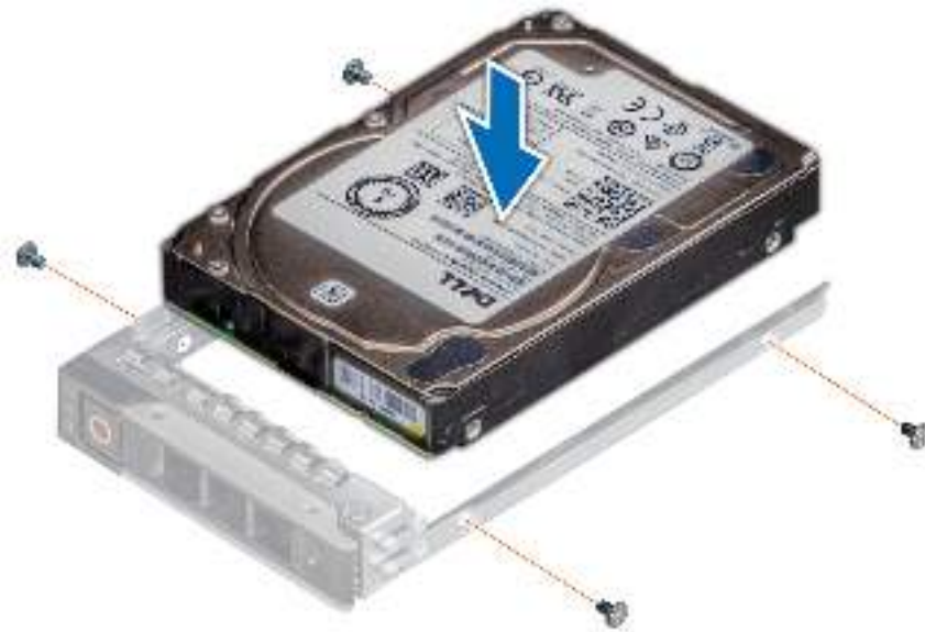
Figure 32. Installing a drive into the drive carrier
