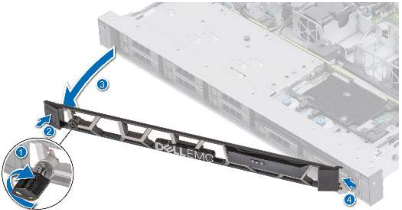
Figure 9. Removing the front bezel with the LCD panel
