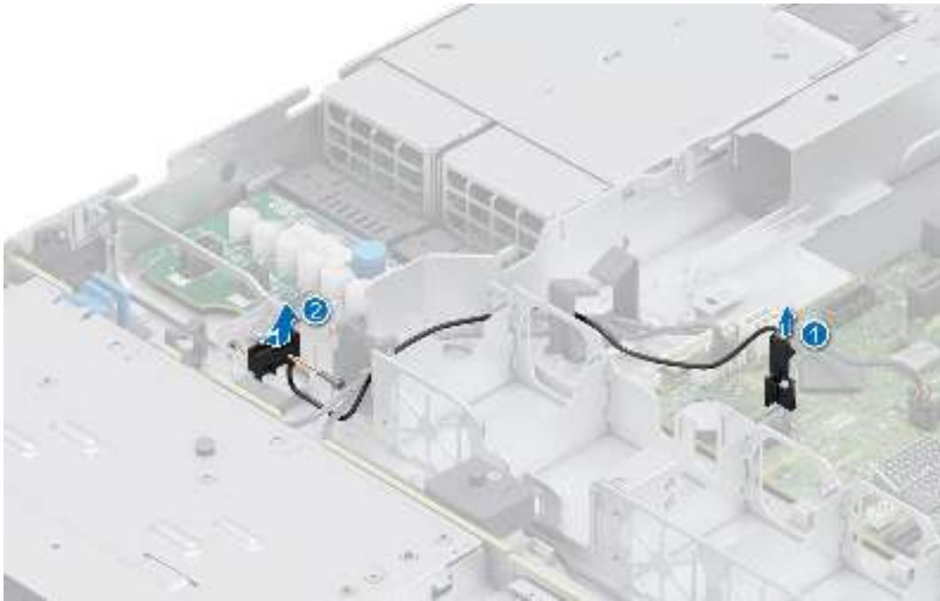
Figure 17. Removing the intrusion switch module
