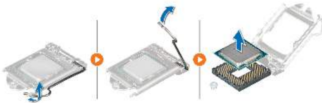
Figure 43. Removing the processor
