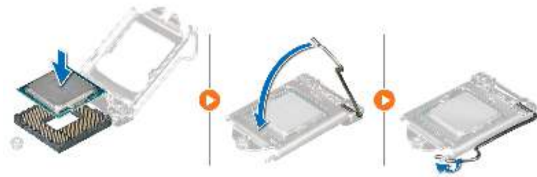
Figure 44. Installing the processor
