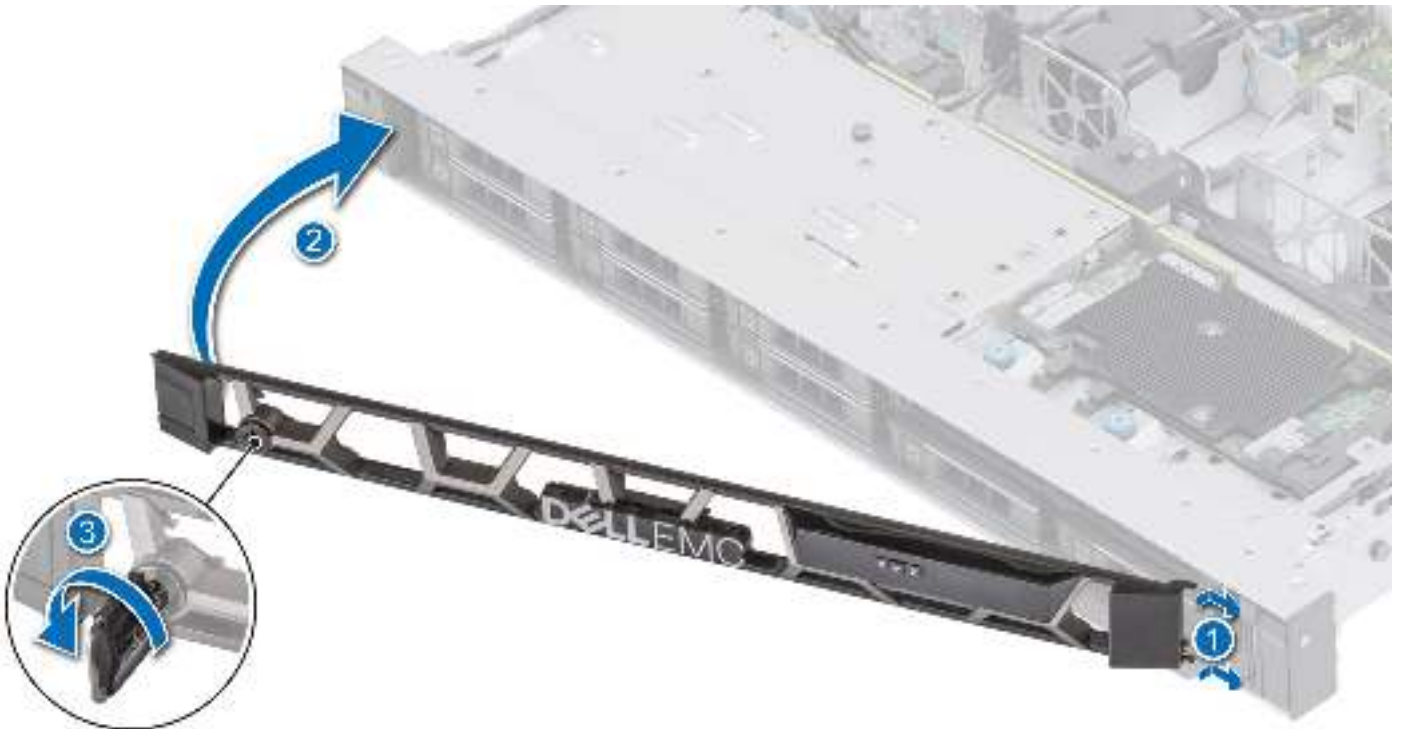
Figure 10. Installing the front bezel with the LCD panel
