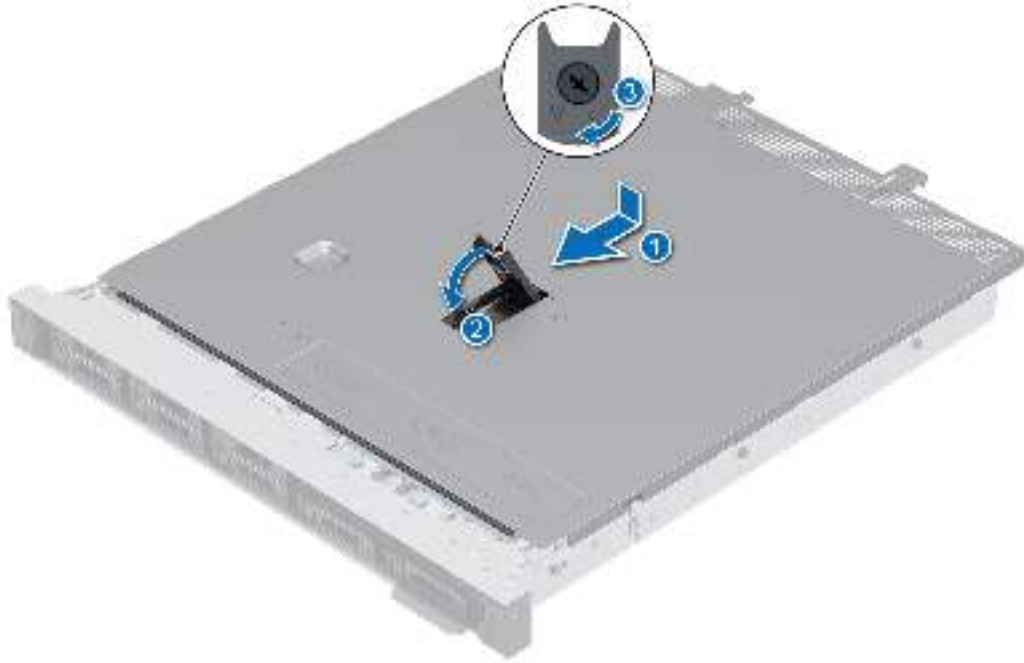
Figure 12. Installing the system cover
