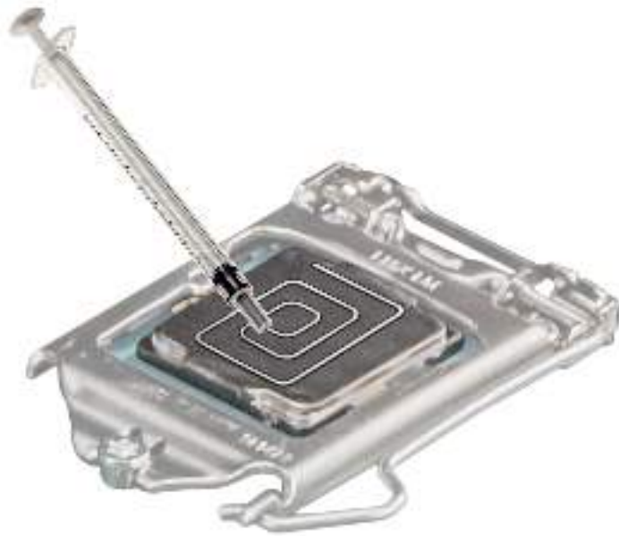
Figure 41. Applying thermal grease on top of the processor
