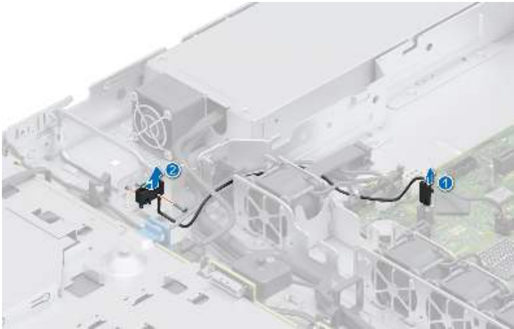
Figure 21. Removing the intrusion switch module
