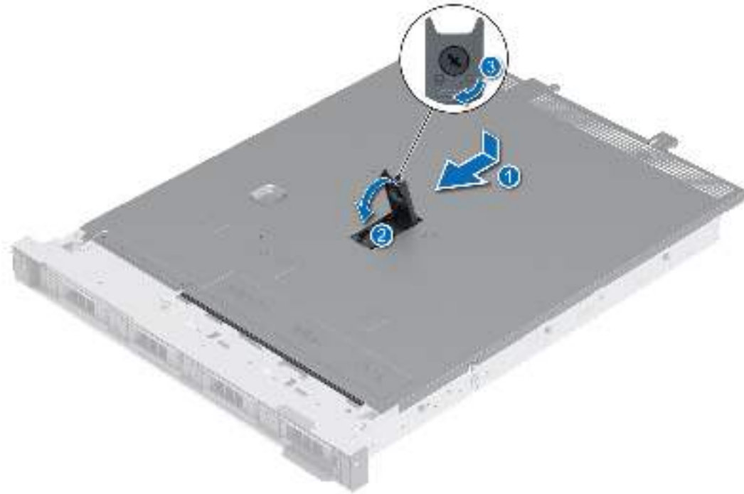
Figure 14. Installing the system cover
