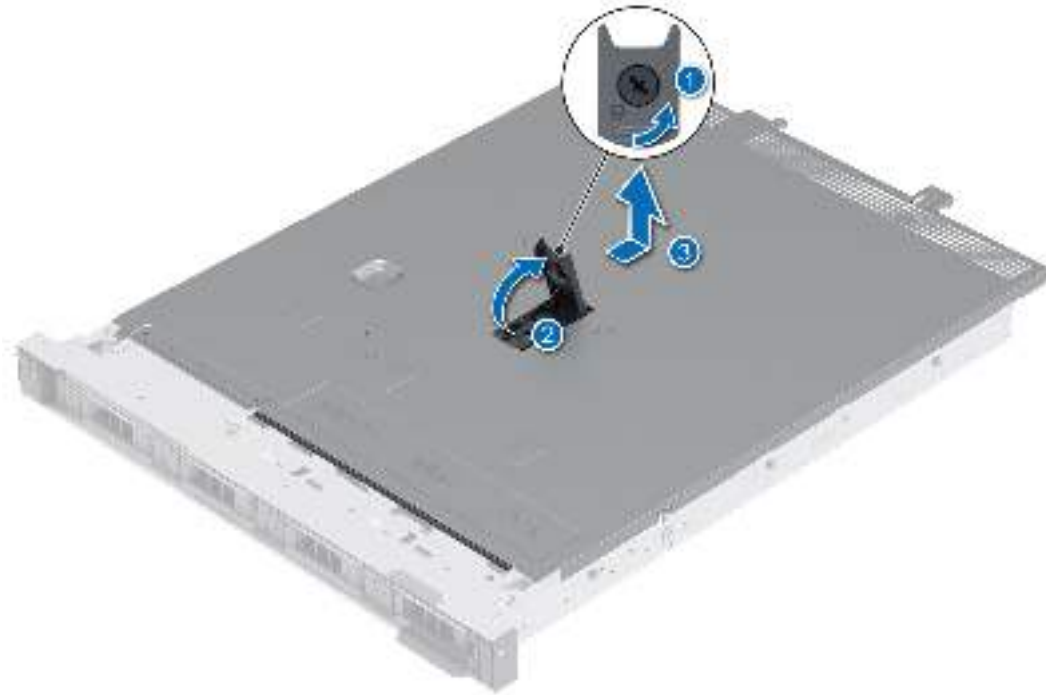
Figure 13. Removing the system cover
