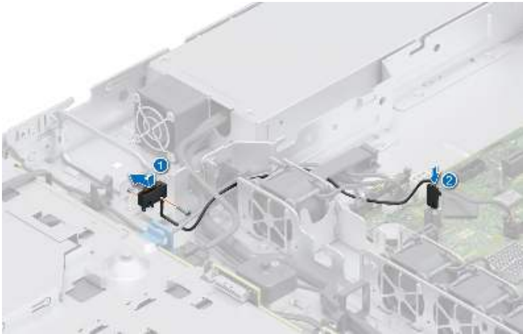
Figure 22. Installing the intrusion switch
