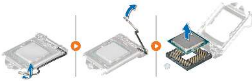
Figure 44. Removing the processor
