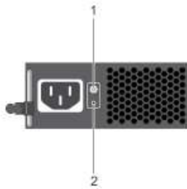
Figure 79. Non-redundant cabled AC PSU status indicator and self-diagnostic button
