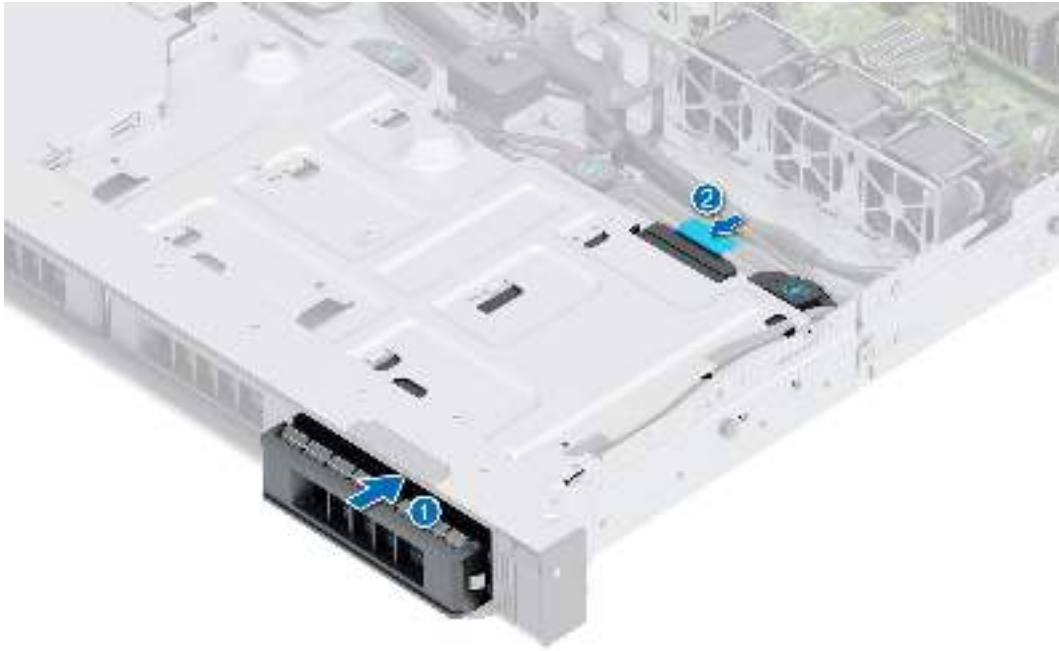
Figure 29. Installing the cabled drive
