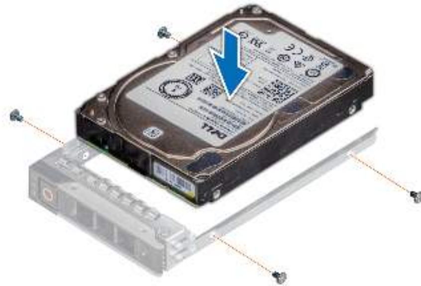
Figure 33. Installing a drive into the drive carrier
