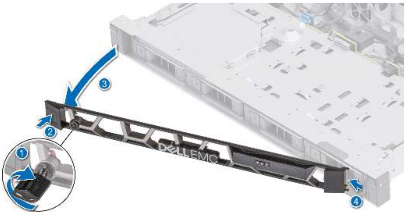
Figure 11. Removing the front bezel with the LCD panel
