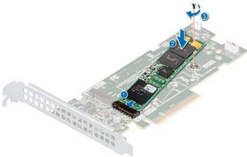
Figure 62. Installing the M.2 SSD module
