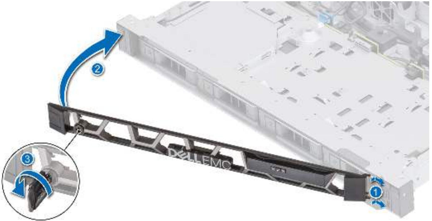
Figure 12. Installing the front bezel
