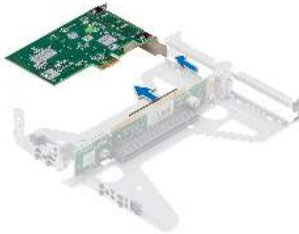
Figure 53. Removing an expansion card from the Riser
