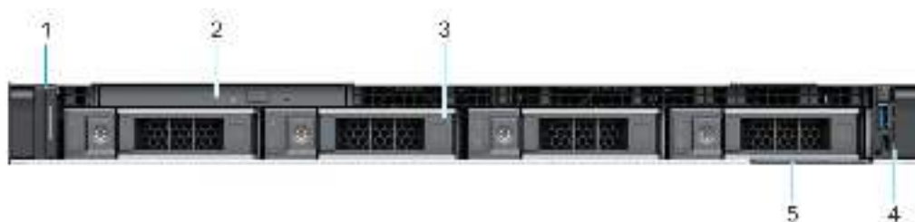
Figure 3. Front view of 2 x 3.5-inch cabled SAS/SATA drive system
