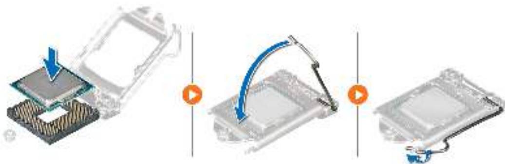
Figure 45. Installing the processor
