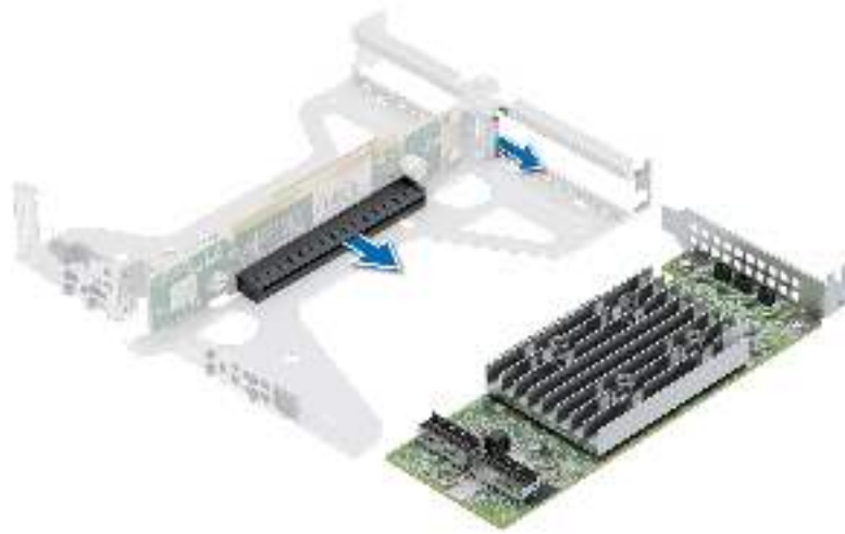
Figure 64. Installing the adapter PERC
