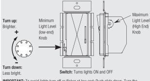
**IMPORTANT:** To avoid lights turn off or flicker at low end: Push slide down. Turn the low-end knob clockwise until the lights remain on without flickering.
