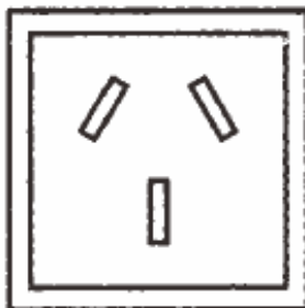
Figure 3- Standard 10A 240VAC Australia / New Zealand receptacle
