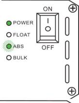
When the charger is in the second stage of charge, the Abs LED will be flashing
