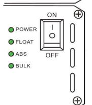
If all lights are illuminated solid, turn the charger off and inspect all connections between the charger and battery to ensure that they are tight.
