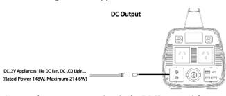
2. How to charge car accessories via the DC Cigarette Lighter socket? The ITECH500 has a 12V-16.8V cigarette lighter port with a rated output of 10A and a maximum of 14.5A, which can power equipment, such as car vacuum cleaners. car refrigerators, and car power tools. Press the DC button, once the DC indicator is on, it can supply power to car electrical devices.
