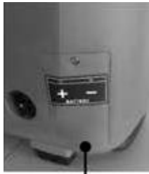
Battery access panel
