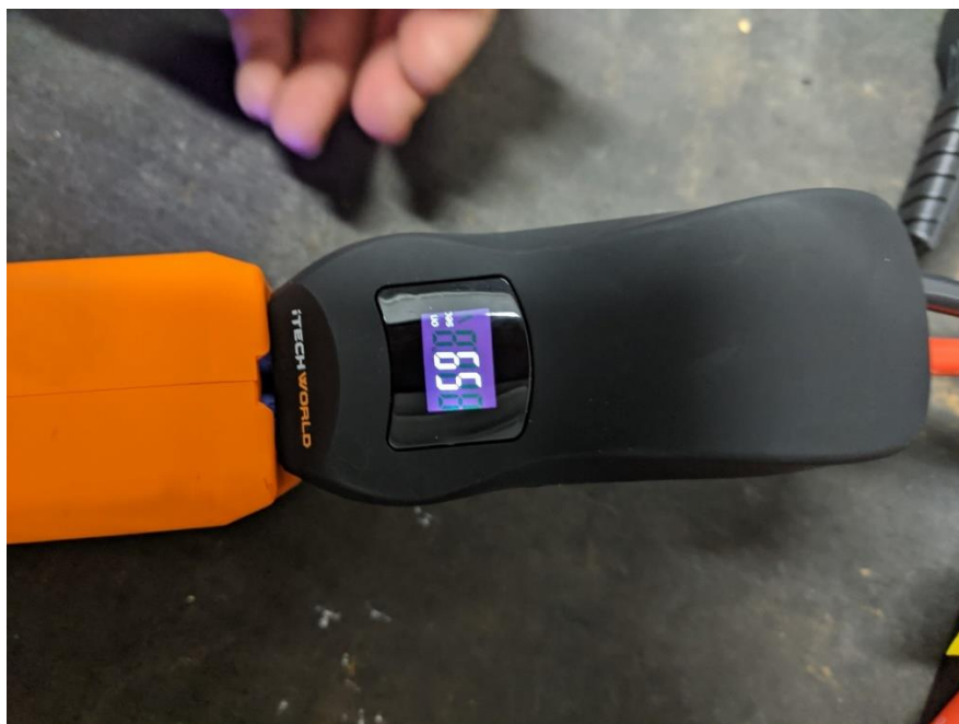
Figure 6 Countdown initiated on the iTECH2000A
