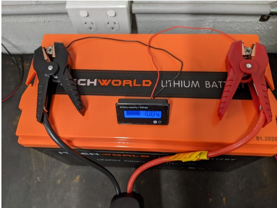
Figure 7 iTECH120X BMS successfully reset and allowing current to flow
