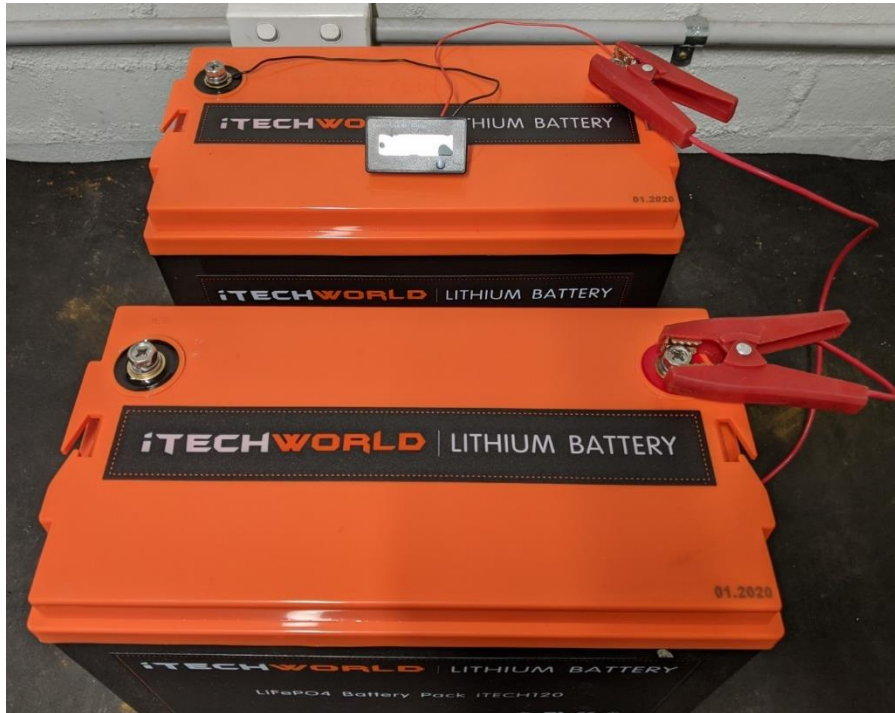
Figure 2 Resetting iTECH120X BMS with jumper cables
