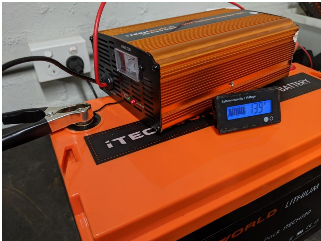
Figure 10 Reconnected charger clamp and charger is now outputting power
