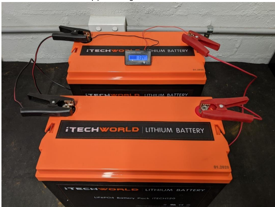
Figure 3 iTECH120X battery connected in parallel with jumper cables
