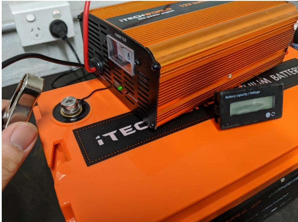
Figure 9 Temporarily removing the negative charger clamp
