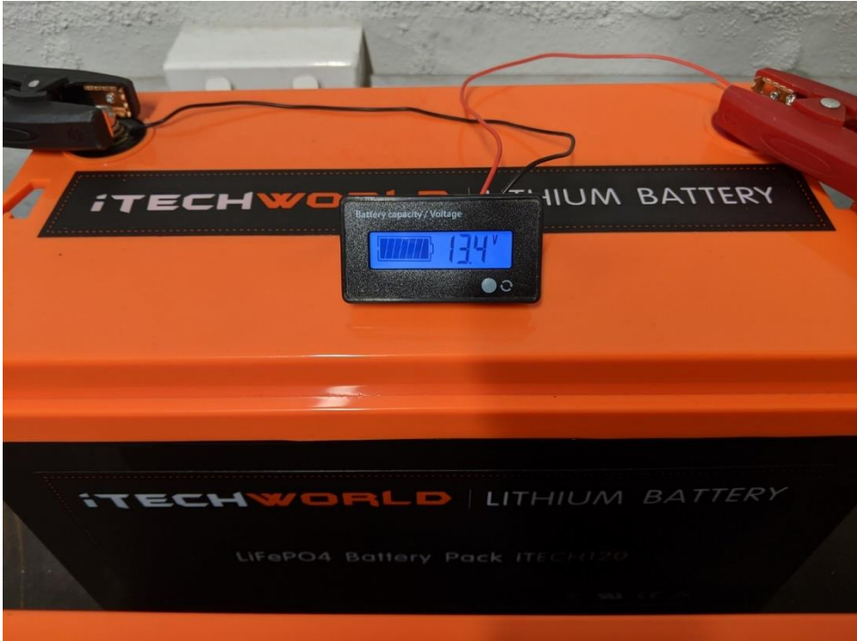
Figure 4 iTECH120X BMS successfully reset and allowing current to flow
