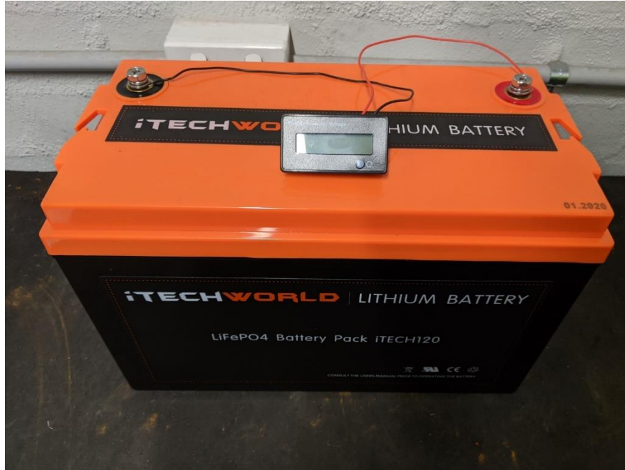
Figure 1 iTECH120X with the BMS in safe mode and not allowing any current flow
