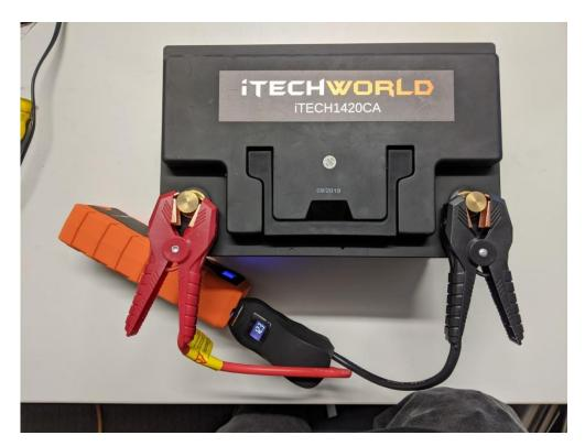
3. Locate the jumpstart button on the side of the clamps and press it. (it is a small black round button on the side of the clamps) Once pressed the countdown timer will start.
