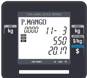
④ Press the PRINT key. Markdown(STRIKE THROUGH) printed on label as figure.
