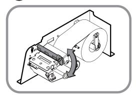
7 Press the FEED key. Scale prints twice for auto Label adjustment
