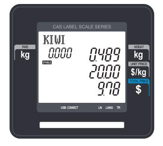
③ Place an item on the platter. In this case, discount is possible because the weight of item(0.526 kg) is greater than 1st target (0.500 kg) therefore the total price is 10.26.
