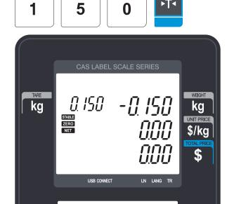
② Enter the weight of container using numeric keys.
