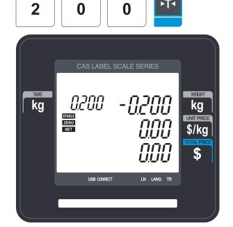
③ Press "TARE key after removing item and container from the platter.
