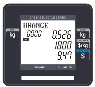
4 Place items on the platter. In this case, the weight of items(1.076 kg) is greater than 2nd target(1.000 kg) therefore you can have 20% discount. (Total price is 17.22)
