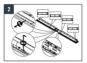
For larger frames, connect profiles together ensuring the numbers match. Use the Allen keys to screw the joint connectors in place. Connect electrical cables.
