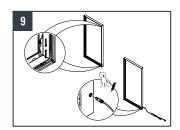
Before plugging the lightbox into the power outlet, make sure that all of the internal plugs are connected and the lightbox is set up correctly.
