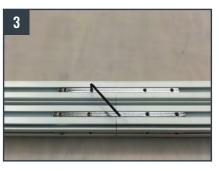
Use the allen key provided to tighten & secure the connectors into the profiles. Perform the same process for the connectors on the sides of the profiles. There will be 6 connectors total.
