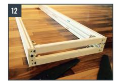
Now, position yourself at the bottom of the frame to install the feet. Unscrew the screws, set the feet in place and screw them into the structure.
