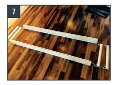
Once the vertical profiles have been assembled, position your BASE and TOP profiles.
