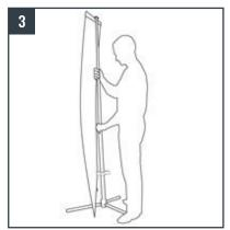
Unscrew one of the two black rings to release and adjust the telescopic pole.
