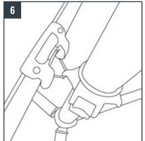
Attach the bottom hanger to the pin on the adjustable ring. The thumbscrew will allow you to adjust the position up or down. The tension between the top/bottom hangers secures the graphic on the stand.
