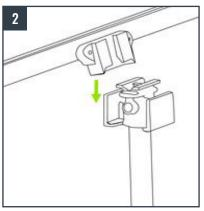
Take the graphic by the top hanger bat and clip it onto the pole head using the center piece.
