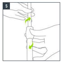
Twist to the left to loosen and right to tighten the grip plastic locks, while adjusting the banner height.
