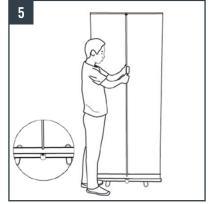
Insert the pole into the base and adjust the perpendicularity in order to avoid waving of the graphic.
