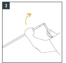
Unfold 3-piece pole. The tension of the bungee cord adjusts the pole into the base automatically.
