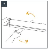
Turn out the stabilizing feet of the base.
