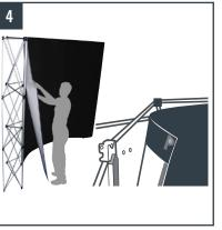
Hang panels by aliging magnets on top corners of panels to magnets on top hubs. Align magnetic tape on rear of panels to the magnetic channel bars.
