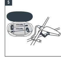
Install lights located inside the case lid by inserting the base of the light adapter into the 'X' created by the top horizontal cross bars of the frame.
