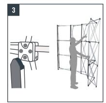
Install the magnetic channel bars into the vertical columns across the entire front of the display as well as the two rear edges of the frame.
