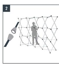
Ensure that the grey adjustable feet located on the bottom of the frame are facing the ground and pull the frame open until the magnetic locking connectors engage.
