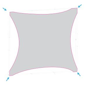
**STEP 2.** Position the graphic on the frame, make sure the top of the graphic is at the top of the frame. Begin pressing the silicone edge into the frame, start with all 4 corners first.
