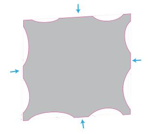
**STEP 3.** With the corners of the graphic in place, press the silicone edge in the middle of the frame on all 4 sides.
