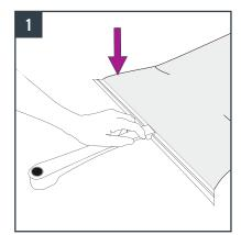
On a clean surface, put the base into the groove of the graphic kicker by centering
