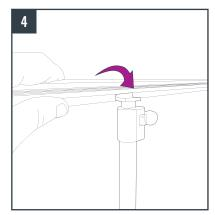
Insert the graphic hanger into the centre of the pole's head.
