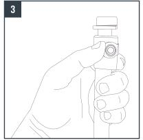
Open the locking clamp on the top of the telescopic pole.
