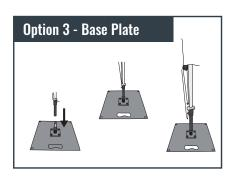
Place the pole onto the base plate and secure the graphic using the provided cord.
