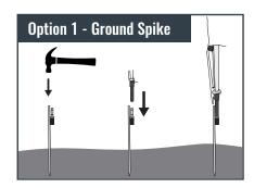
Hammer the top of the steel rod into the ground. Place the pole onto the ground spike and secure the graphic using the provided cord.
