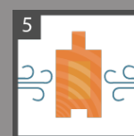
5 Timber is left to air dry
