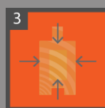
3 Preservative is absorbed into the surface of the timber.
