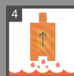
4 Timber is removed from cylinder containing preservative
