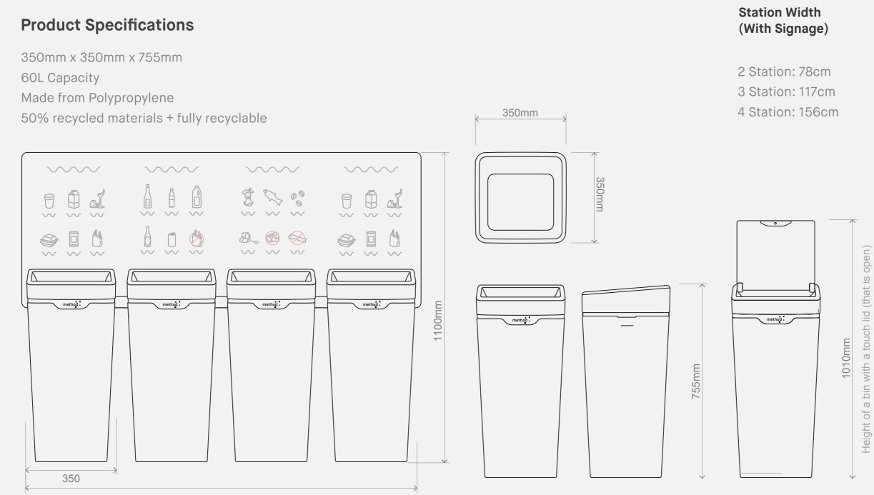
1560mm - 4 bins connected with HD connectors
