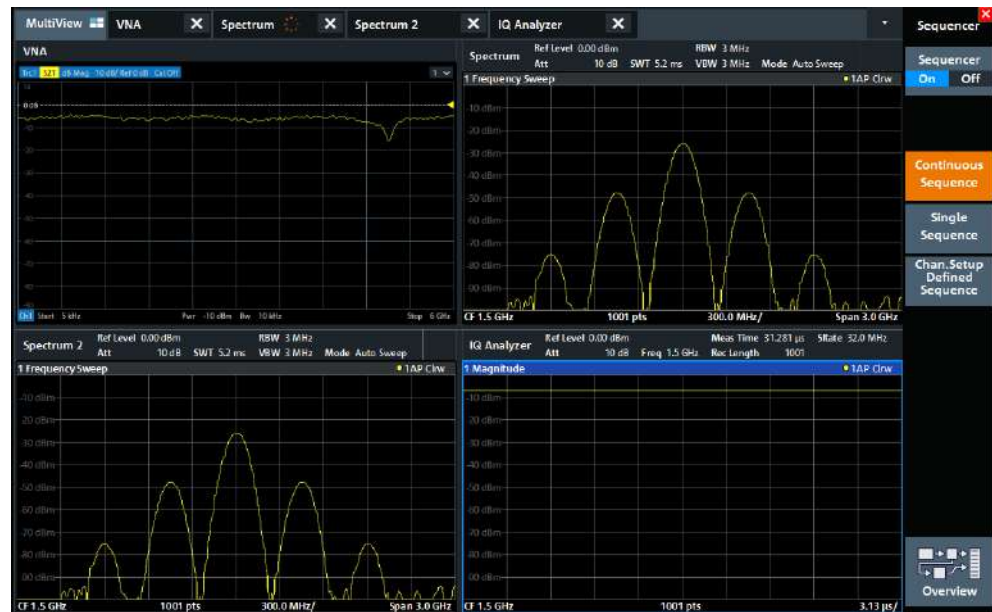
Figure 4-16: "MultiView" tab with active Sequencer
