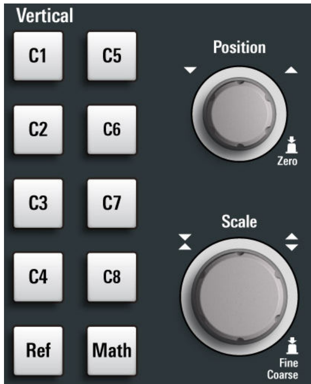
Figure 3-5: Vertical controls of R&S MXO 5 with 8 input channels
