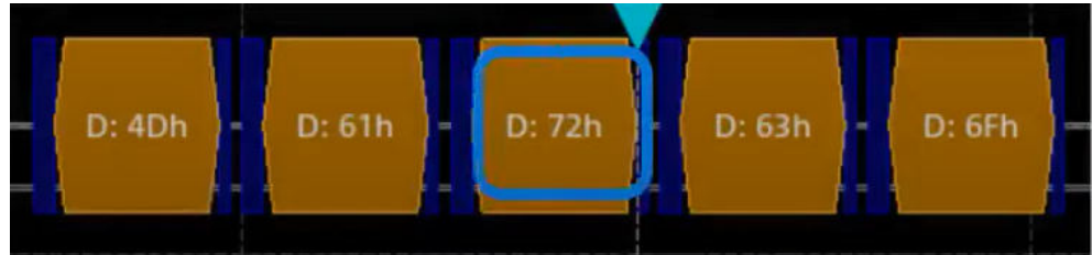
Figure 13-12: Trigger on Type= Tx, Data =0x72 and Position=3
