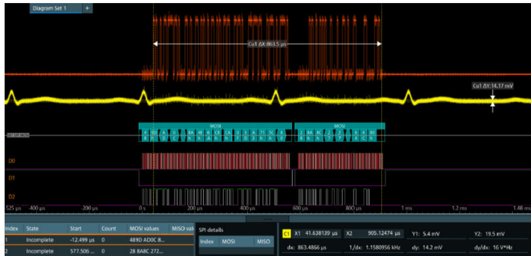
Figure 13-3: Decoded and binary SPI signal
