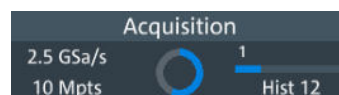
Figure 4-9: Progress of incomplete long acquisition in average mode, Run Single = 5, first acquisition is finished
