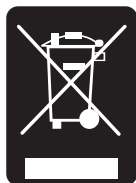
Fig. 1.4: Product labeling in accordance with EN 50419.
