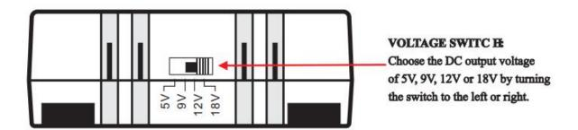
Warning: Please make sure that the output voltage is correct, a wrong voltage may destroy the device which you want to power up.
