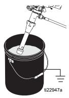
Turn prime valve down DRAIN position. Unplug sprayer.
