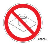
**Grounding a metal pail:** connect a ground wire to the pail by clamping one end to pail and other end to a true earth ground.
