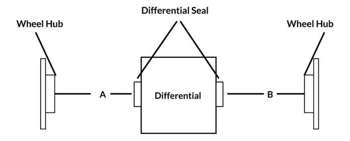
Typical measurements *from diff stubs to inside of hubs*.
