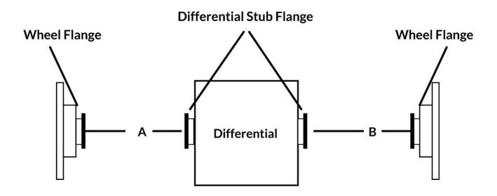
Typical measurements <u>from splined diff stub shafts to inside of wheel hubs</u>.
