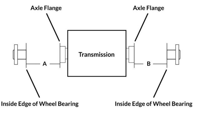
Typical measurement with stub shafts on transmission
