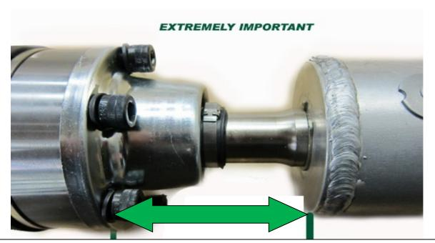
Driveshaft CV Clearance <u>MUST BE CHECKED</u> after installation. This measurement must be between <u>3.25" – 3.75"</u> If dimension is not within the allowed range, do not run the driveshaft
