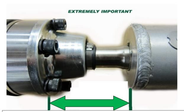
Driveshaft CV Clearance <u>MUST BE CHECKED</u> after installation. Camaro ZL1 (Auto / Manual) must be between <u>3.25" – 3.75"</u> If dimension is not within the allowed range, do not run the driveshaft
